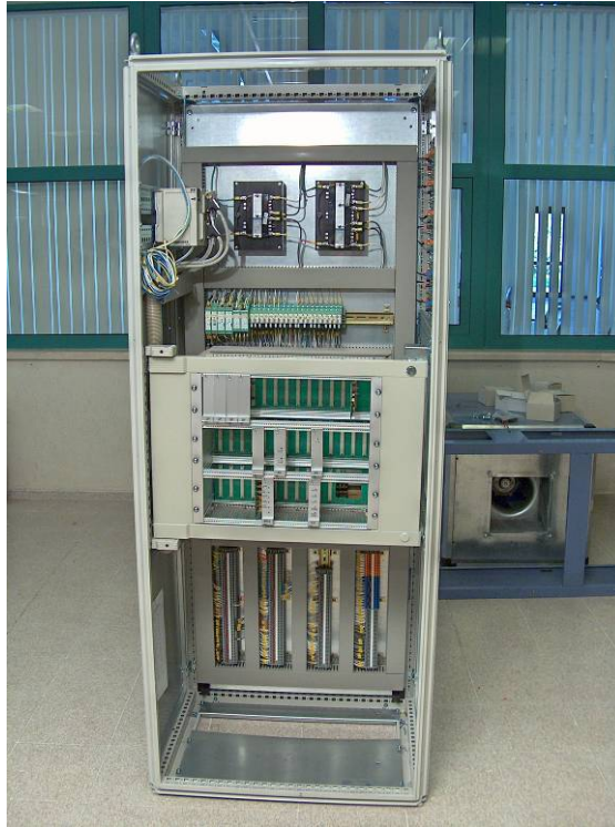
Fig.4.19. Control panel designed for YLI SVC system.
