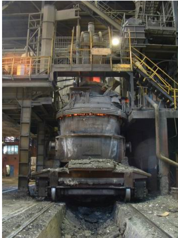
Fig.2.9. ISDEMIR Ladle furnace (120 metric tones) [4]
