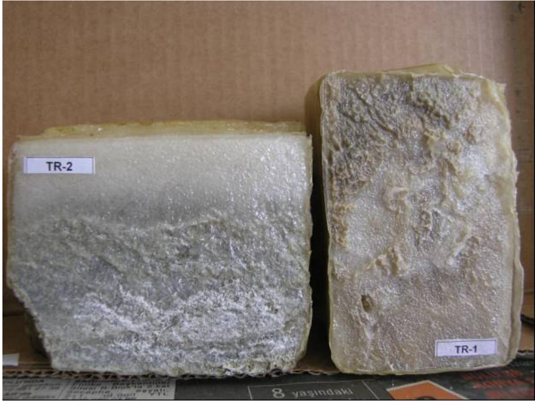
Figure 1 Leaching surfaces of samples taken from heap stored during decline driving
