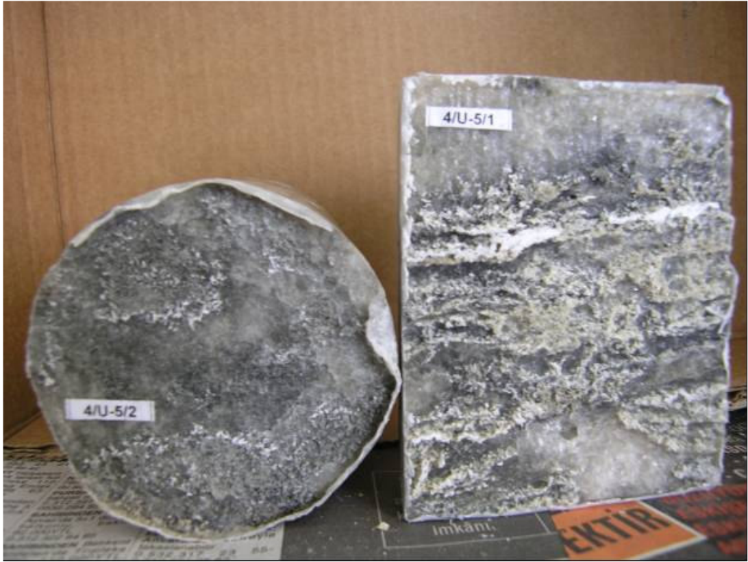
Figure 3 Leaching surfaces of samples taken from V004 vertical well U-5 seam
