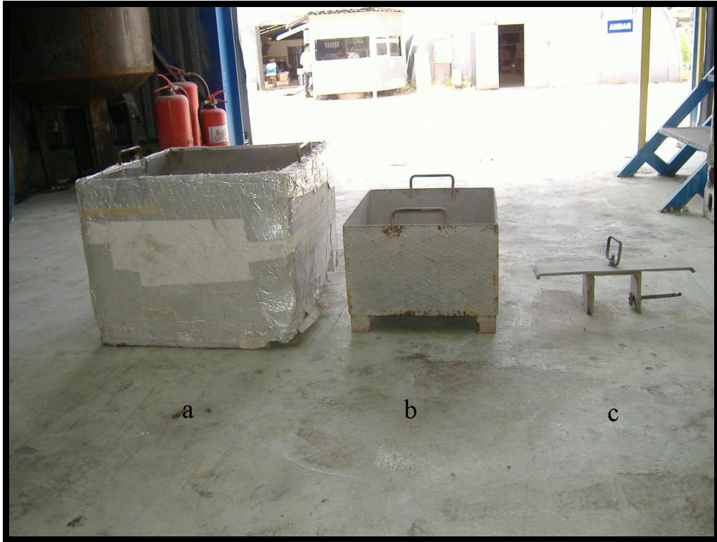
Figure 6.3 (a) thermostat box, (b) leaching tank, (c) sample holder
