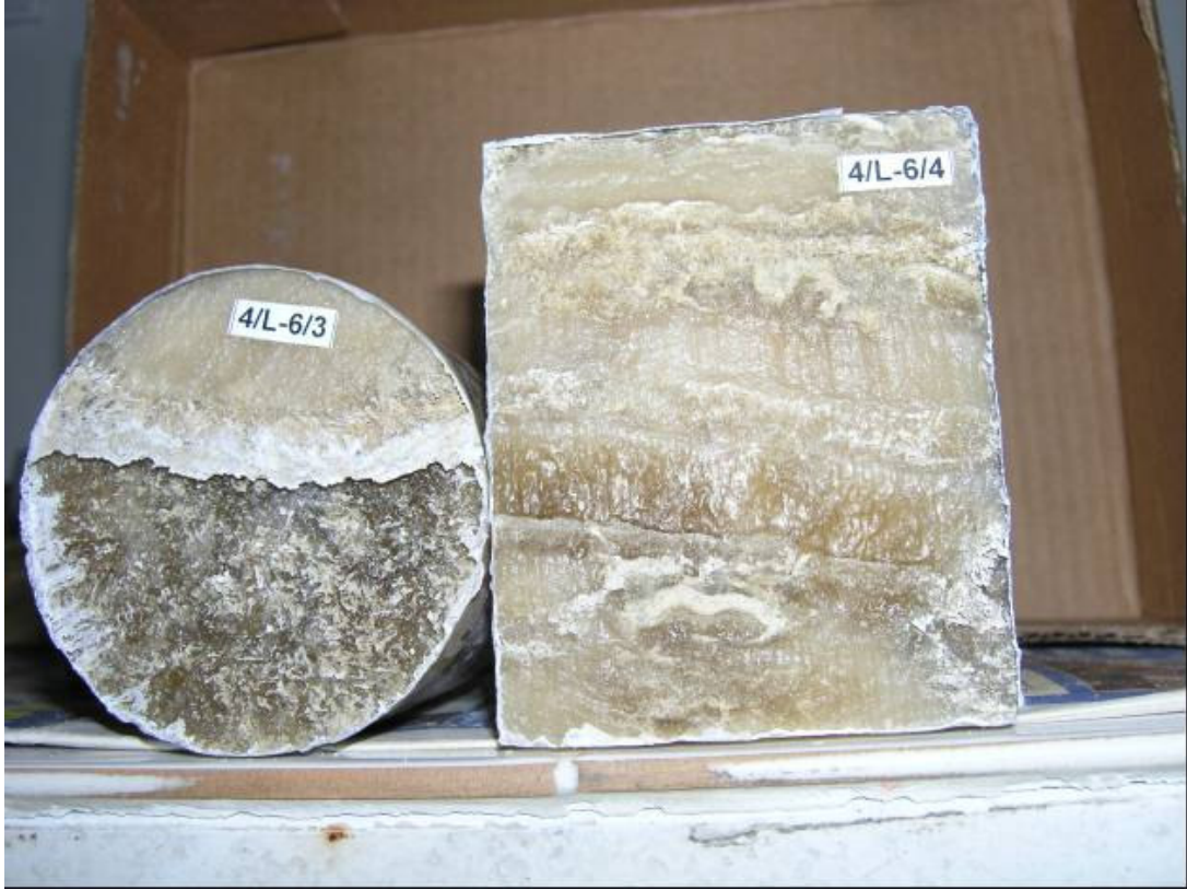
Figure 6: Leaching surfaces of samples taken from V004 vertical well L-6 seam
