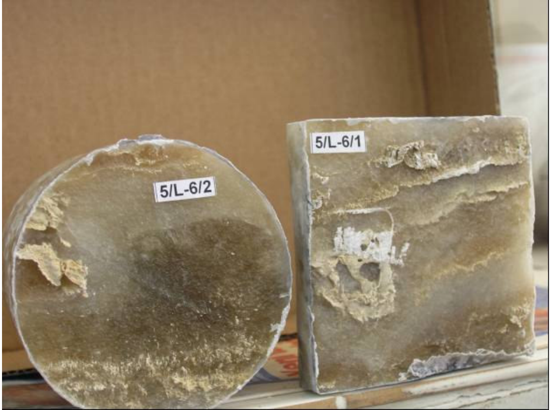
Figure 7: Leaching surfaces of samples taken from V005 vertical well L-6 seam
