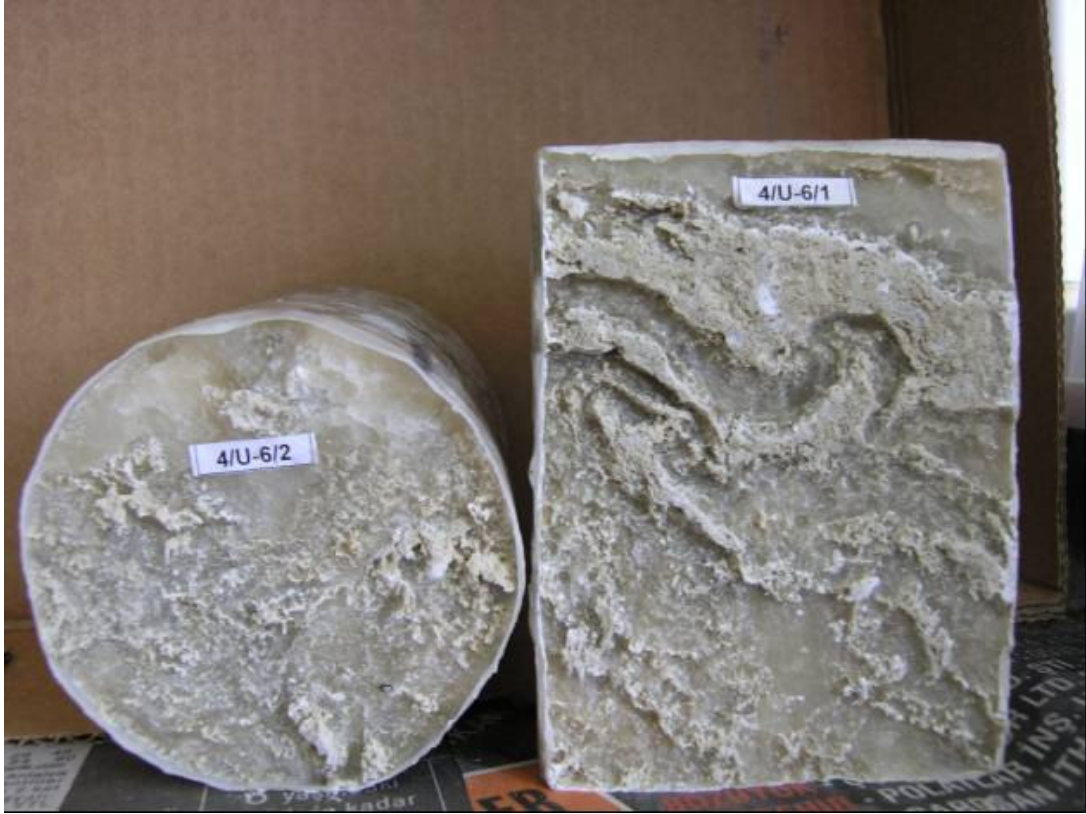
Figure 4 Leaching surfaces of samples taken from V004 vertical well U-6 seam
