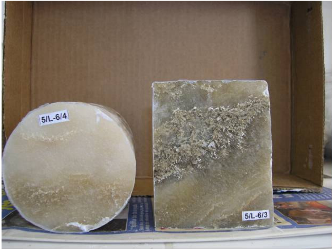
Figure 8 Leaching surfaces of samples taken from V005 vertical well L-6 seam
