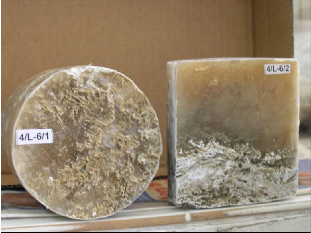
Figure 5 Leaching surfaces of samples taken from V004 vertical well L-6 seam
