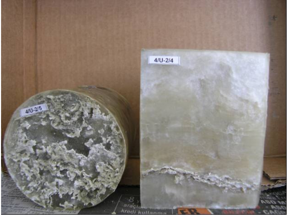
Figure 2 Leaching surfaces of samples taken from V004 vertical well U-2 seam
