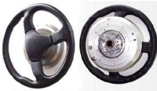
Figure 2 Steering wheel measurement system
