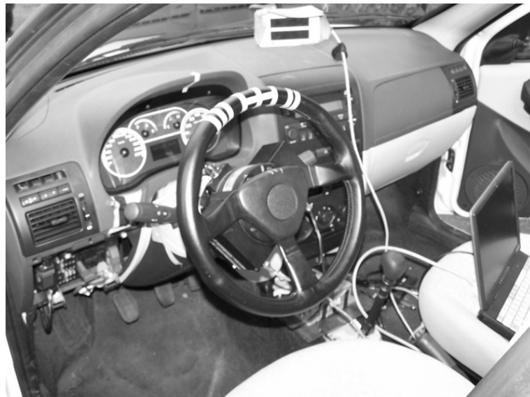
Figure 12 Steering wheel system on the experimental vehicle
