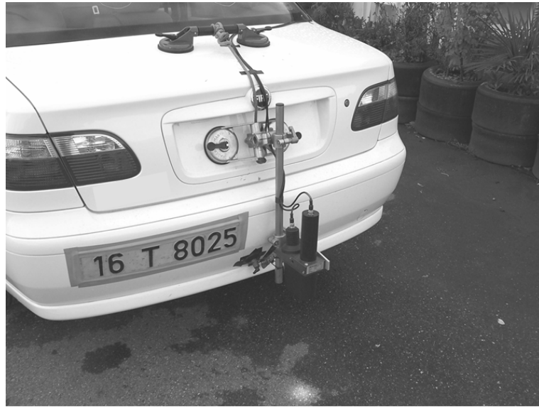
Figure 11 Forward and lateral velocity sensors, at point Q, on the experimental vehicle
