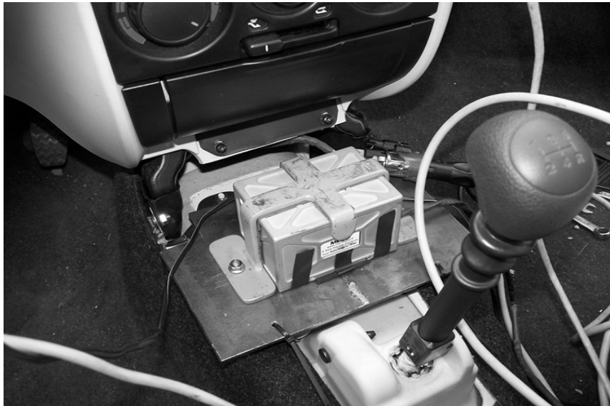
Figure 10 Inertial platform at point P on the experimental vehicle
