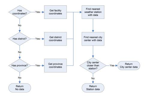
Figure 5.2: Flowchart of nearest weather data retrieval
