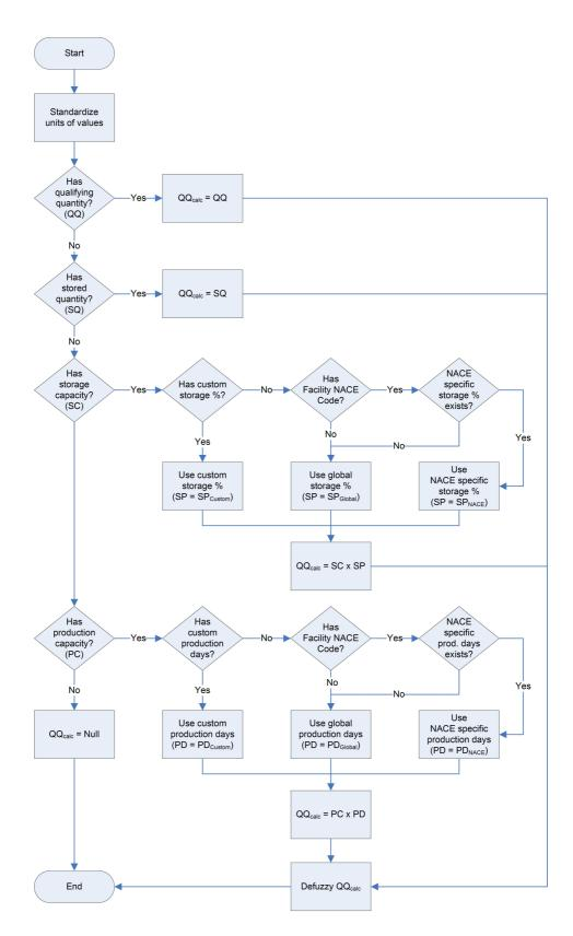
Figure 4.72: Flowchart of qualifying quantity calculation
