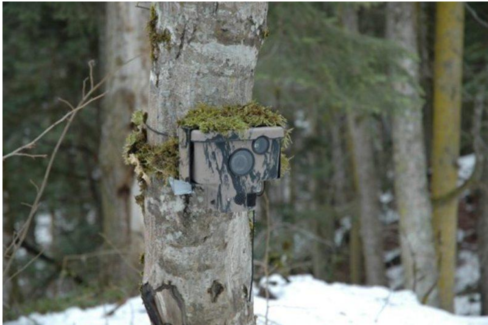
Figure 1. A camera trap unit fixed at a tree. Extra camouflage was achieved by placing moss on the unit (Photograph by Ö. E. Can).
