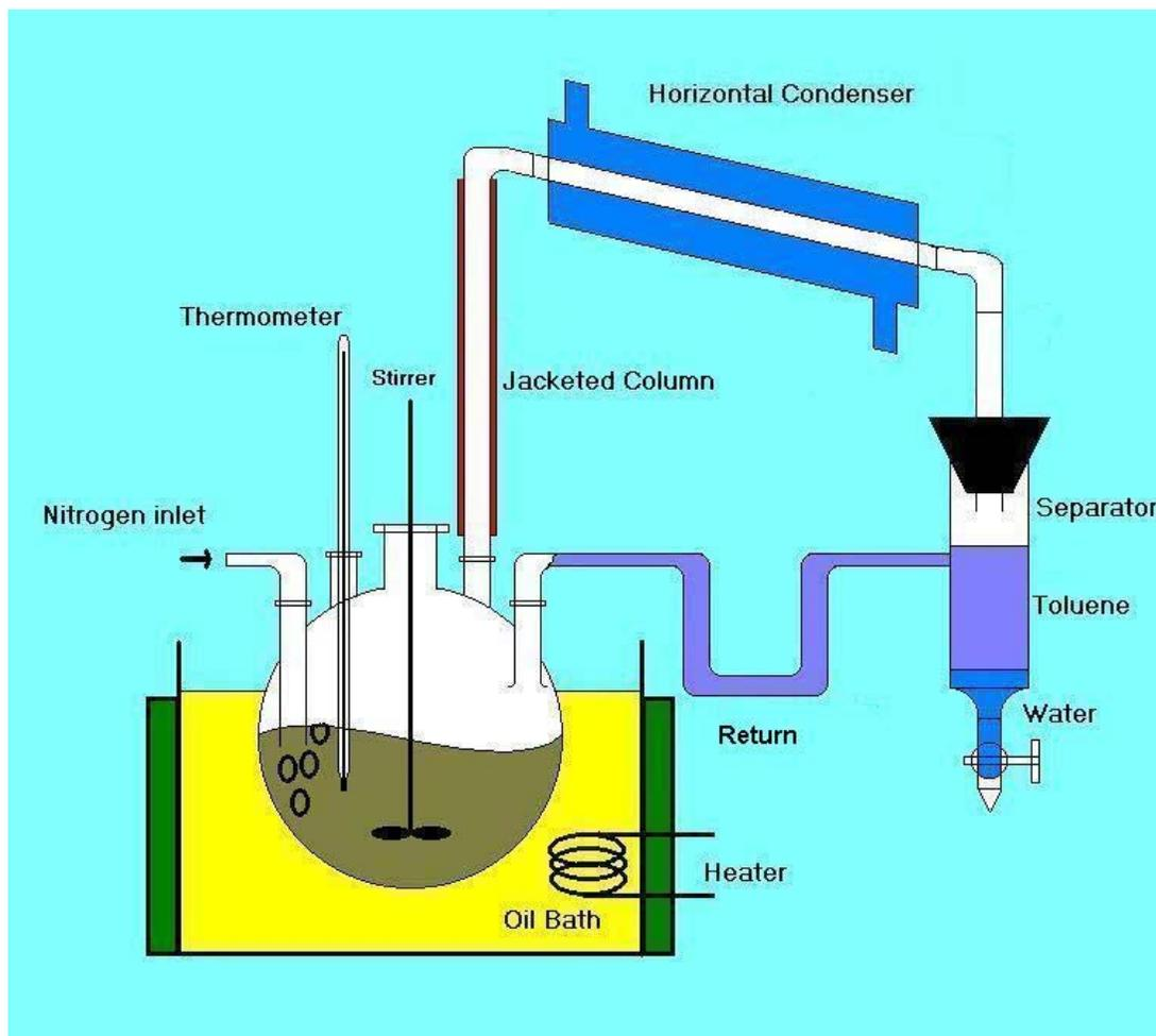
**Figure 2.3** Experimental setup of the hyperbranched polyesters and HBR synthesis (Bat 2005).
