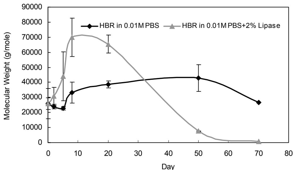
**Figure 3.5** Hydrolytic degradation of HBR in 0.01 M PBS and enzymatic degradation in 0.01M PBS and 2% lipase from *Pseudomonas sp.* (4mg/ml) at 37°C with 50 rpm shaking.
