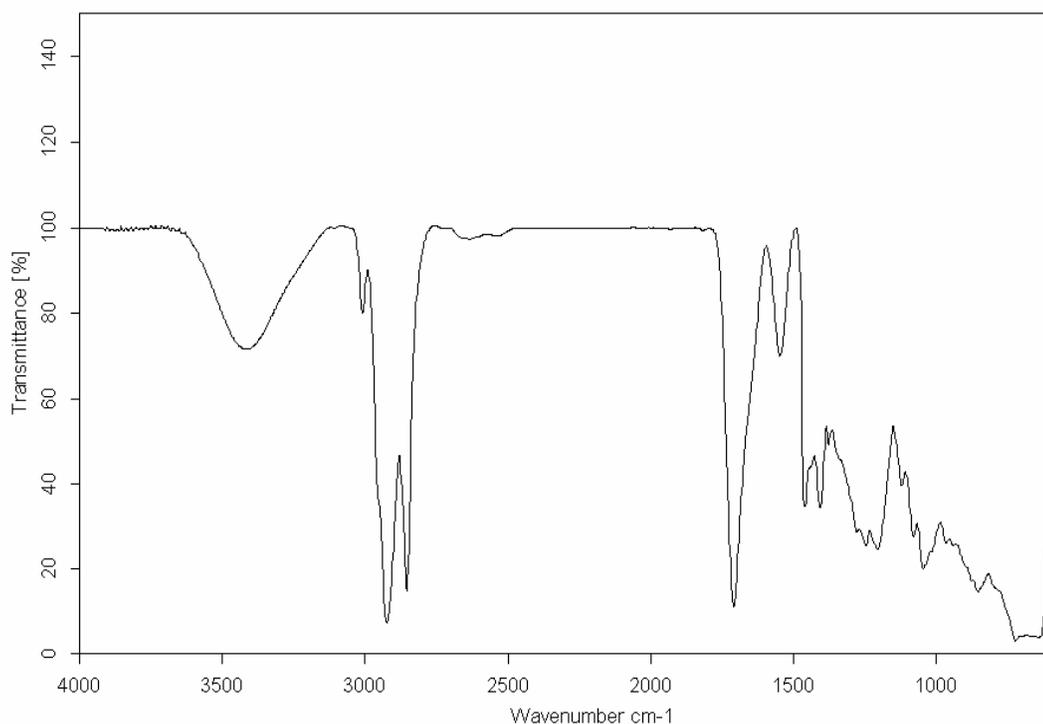
**Figure 3.1** FTIR spectra of castor oil fatty acids (mainly ricinoleic acid).
