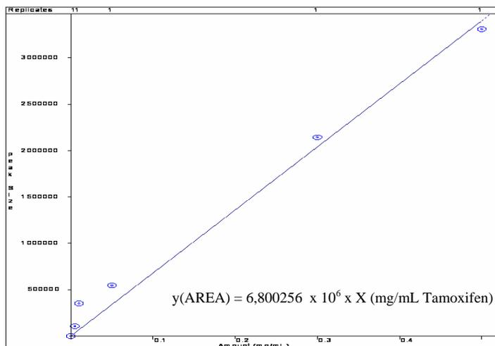
**Figure 2.8** Calibration Curve of tamoxifen by using HPLC method.
