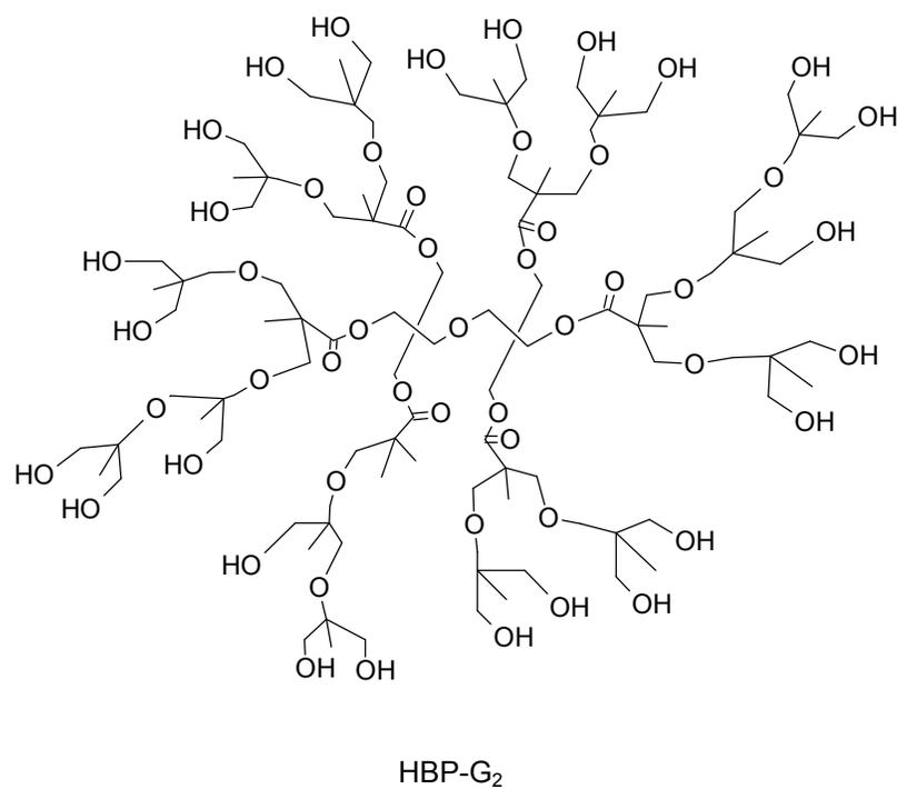
**Figure 2.5** Synthesis and theoretical representation of second generation hyperbranched polyesters ( $\text{HBP-G}_2$ ) by esterification of first generation polyesters ( $\text{HBP-G}_1$ ) and DMPA.
