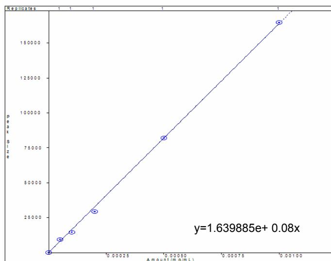
**Figure 2.9** Calibration curve of idarubicin determined by HPLC method.
