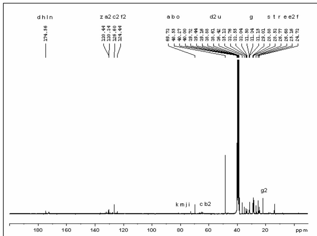
**Figure 3.4**  $^{13}\text{C}$  NMR results of HBR structure. Letters on the top of the peaks are correlated with the letters that shows carbon atoms of HBR in Figure 3.3.
