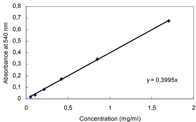
**Figure 2.7** Calibration curve of idarubicin which was determined by UV-vis spectrophotometry at  $\lambda_{\text{max}}=540\text{nm}$ .
