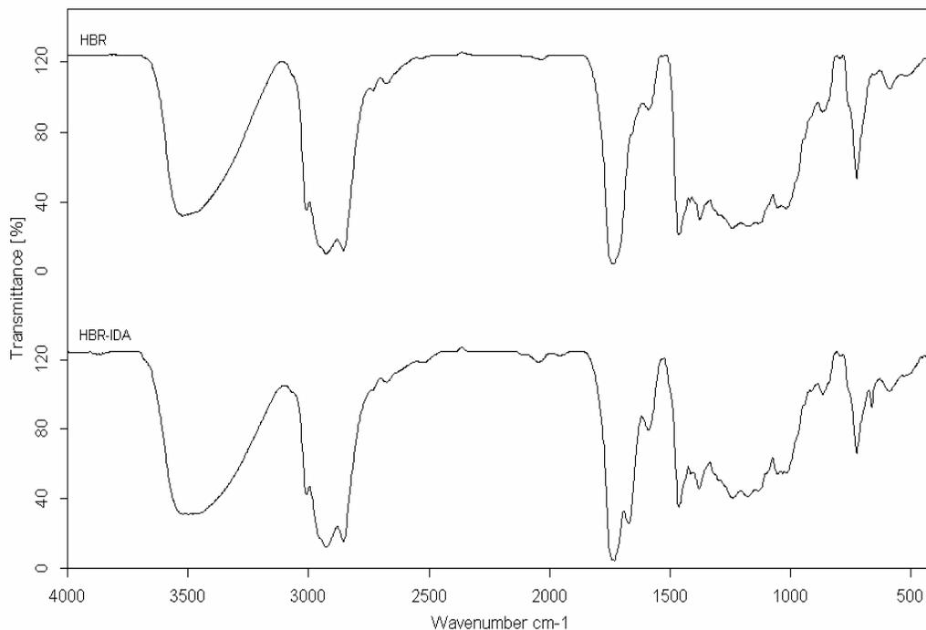
**Figure 3.10** The comparison of FTIR spectra of HBR and HBR-Idarubicin ( HBR-IDA).
