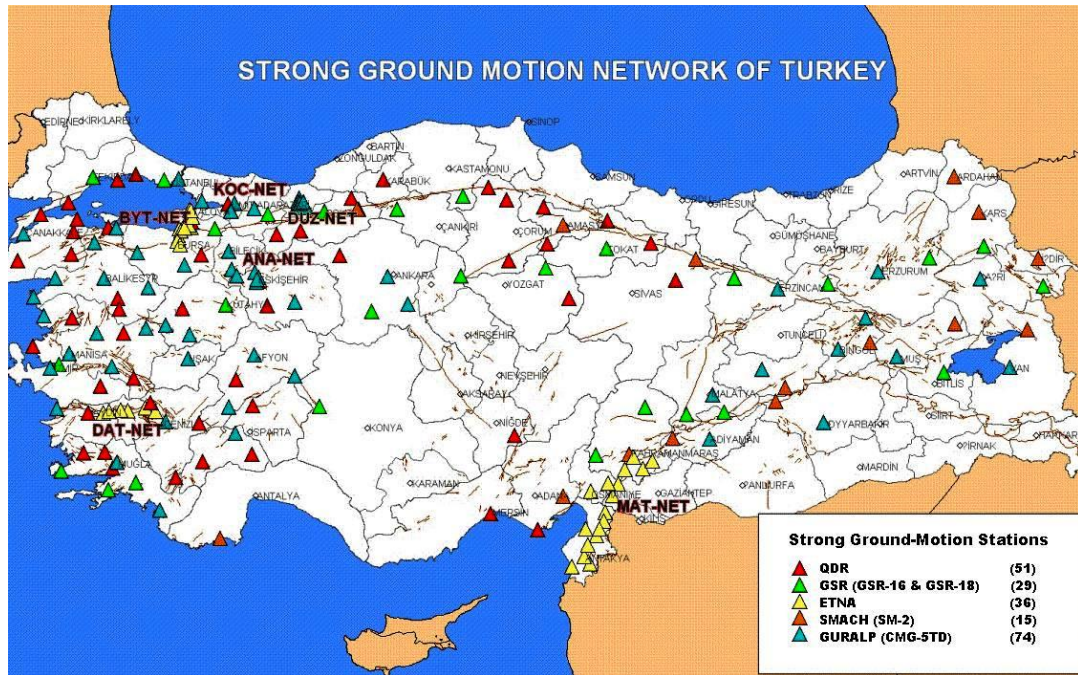
Figure 2.1 Strong ground-motion network of Turkey including regional seismic arrays such as DATNET, ANANET, MATNET, BYTNET, KOCNET and DUZNET (Courtesy of ERD - GDDA).
