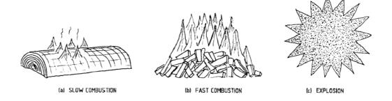
Figure 2.7: As surface area of solid substance increases, combustion rate increases [56]
