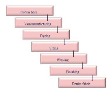
Figure 4.2: Process scheme inside the mill
