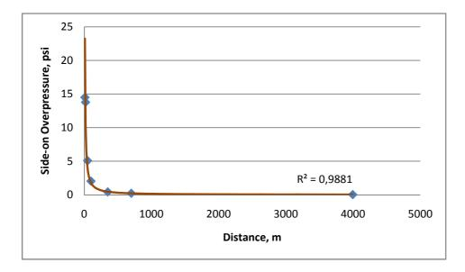
Figure 7.16: Side-on Overpressure vs. Distance
