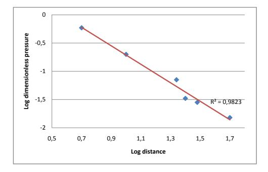
Figure C.1: Side-on overpressure vs. distance
