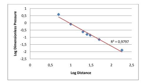
Figure C.2: Side-on overpressure vs. distance
