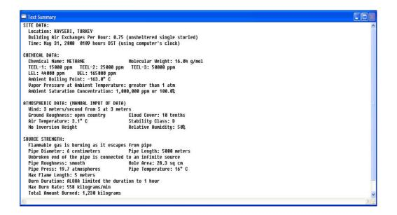
Figure D.3: Text summary of jet fire resulting from natural gas leak
