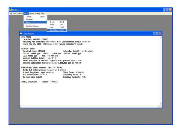
Figure 7.9: Input information regarding to jet fire modelling of methane
