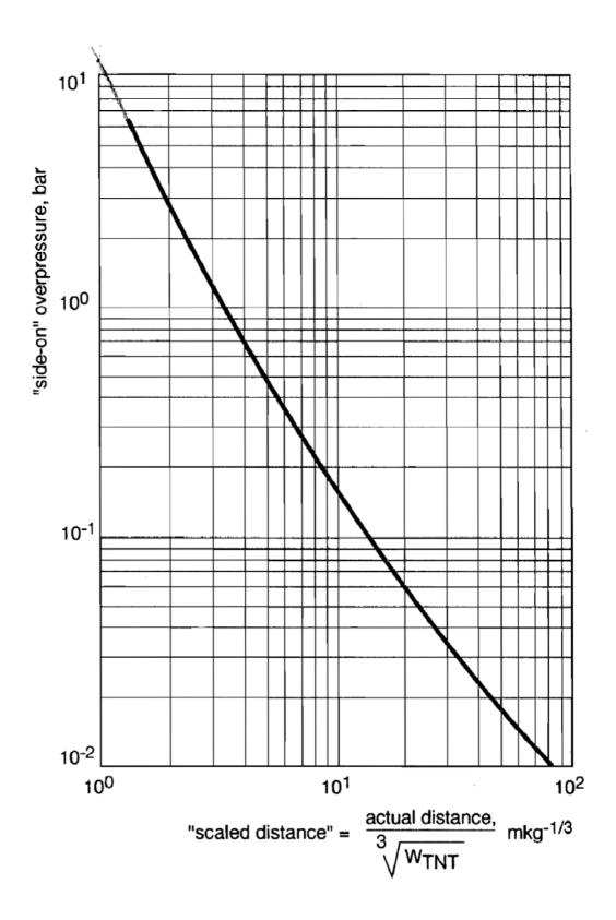
Figure E.1. Hopkinson-scaled TNT Charge Blast Graph [65]
