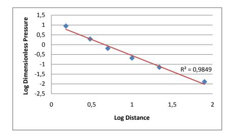
Figure 7.3: Side-on overpressure vs. distance
