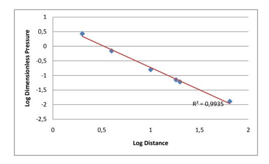
Figure 7.5: Side-on overpressure vs. distance
