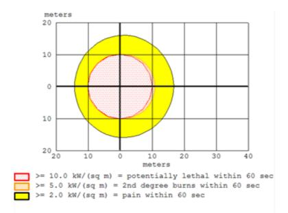
Figure D.4: Thermal radiation threat zone
