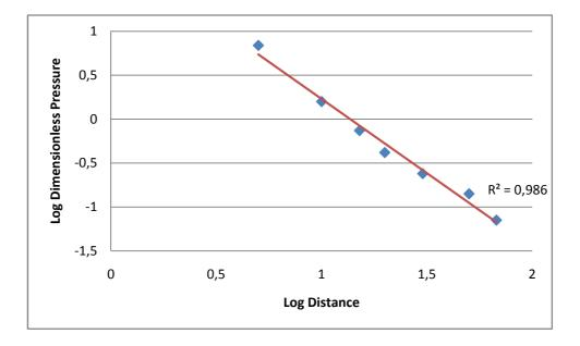
Figure 7.1: Side-on overpressure vs. distance
