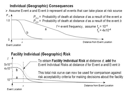
Figure 2.1: Calculation of facility individual risk via summation of event individual risks calculated by multiplying event frequency with the individual event consequences [34]
