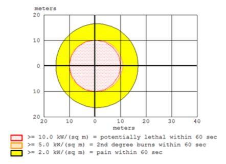
Figure 7.13: Thermal radiation threat zone
