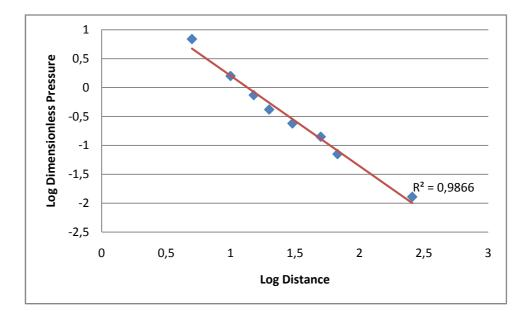
Figure 7.4: Side-on overpressure vs. distance
