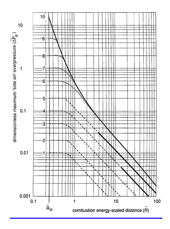
Figure F.1: Sachs scaled side-on peak overpressure of blast from a hemispherical fuel-air charge [65]
