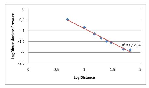
Figure C.3: Side-on overpressure vs. distance
