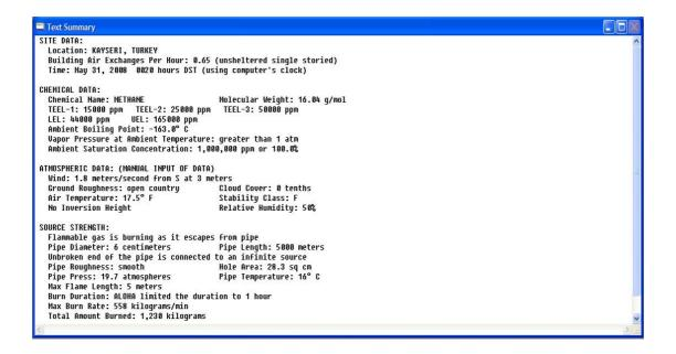
Figure 7.12: Text summary of jet fire resulting from natural gas leak
