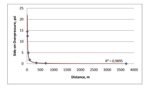
Figure 7.15: Side-on Overpressure vs. Distance
