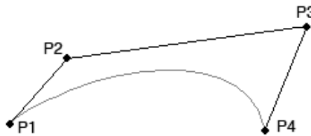
Figure 3 A cubic spline curve which is defined by CP P1, P2, P3, and P4
