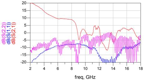
Figure 4.10 S-Parameters After Improved Grounding of Connectors
