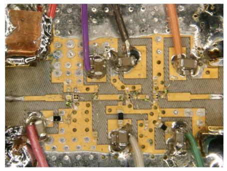
Figure 4.16 Fabricated Circuit of The Second CRTSSDA
