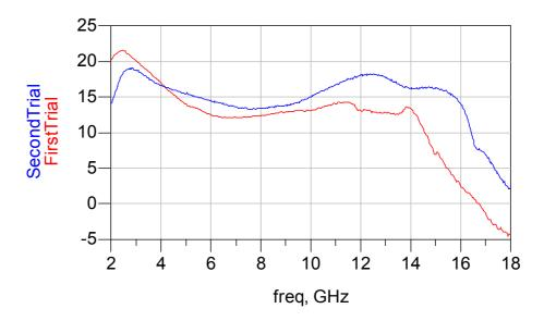
Figure 4.25 Comparison of Gains of First and Second Fabrications
