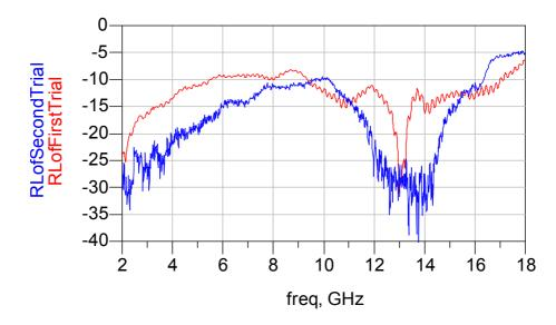
Figure 4.26 Comparison of Input Return Losses of First and Second Fabrications
