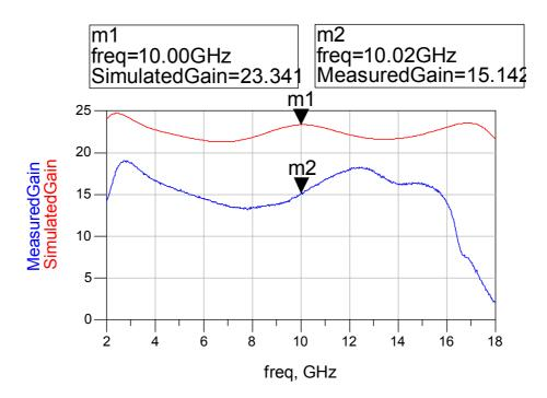
Figure 4.23 Comparison of Gains Between Simulated And Measured Amplifier
