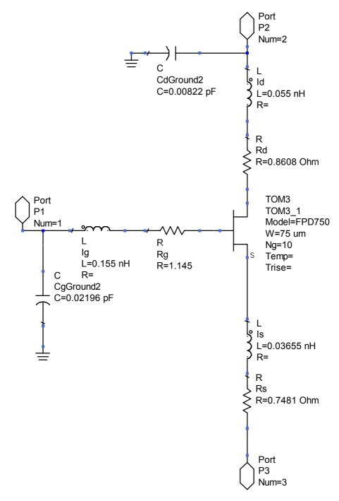
Figure A.3 TOM3 Model with External Parasitic of FPD750
