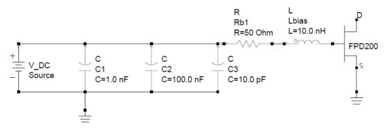
Figure 4.7 Gate Biasing of The First Stage
