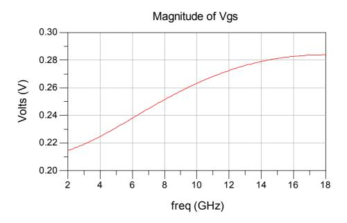
Figure 3.3 Enhancement of Voltage Swing Across  $C_{\rm gs}$  With Reactive Terminations
