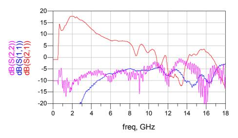
Figure 4.9 S-Parameters After Eliminating Oscillation
