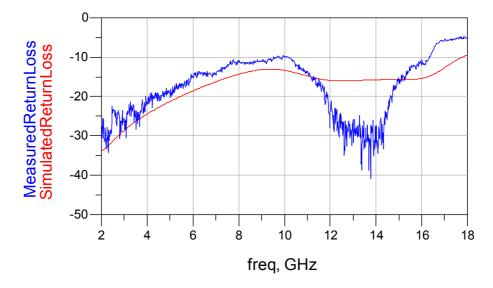
Figure 4.24 Comparison of Input Return Loss Between Simulated And Measured Amplifier
