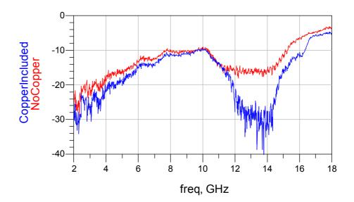
Figure 4.20 Effects of Including Copper Paltes on Input Return Loss
