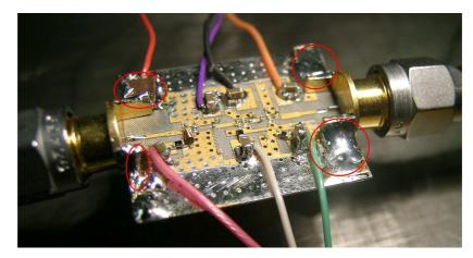
Figure 4.19 Copper Plates Soldered to Improve Grounding
