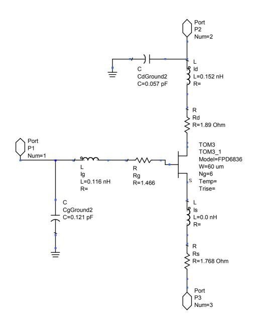
Figure A.2 TOM3 Model with External Parasitic of FPD6836
