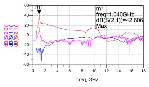
Figure 4.8 Oscillation Caused By Biasing Inductor
