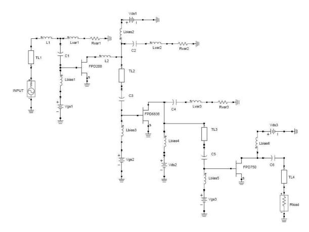
Figure 3.4 Schematic of the Proposed Amplifier
