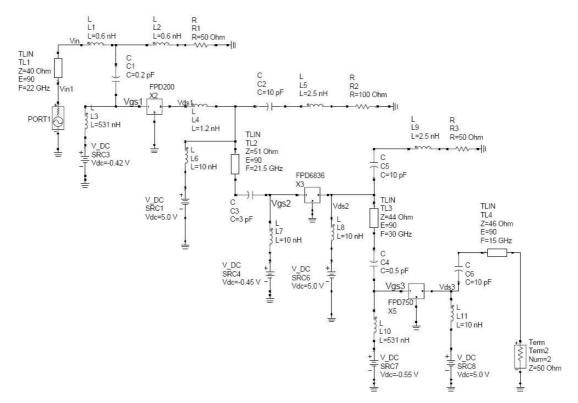
Figure 3.6 Schematic of the Firstly Designed CRTSSDA
