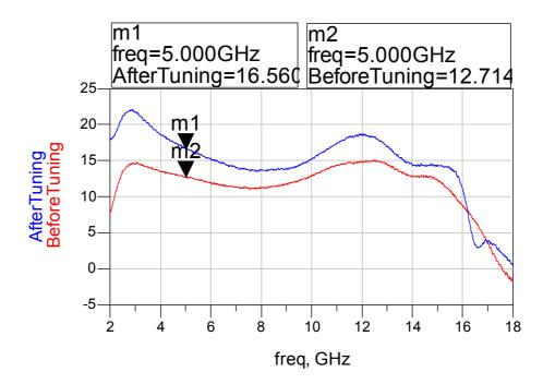
Figure 4.21 Gain of the Second CRTSSDA Before and After First Tuning
