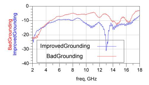
Figure 4.11 Input Return Loss After Improved Grounding of Connectors
