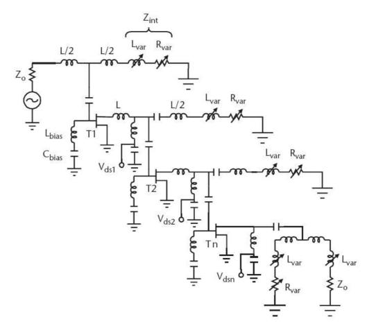
Figure 3.1 Block Diagram of a CRTSSDA [4]
