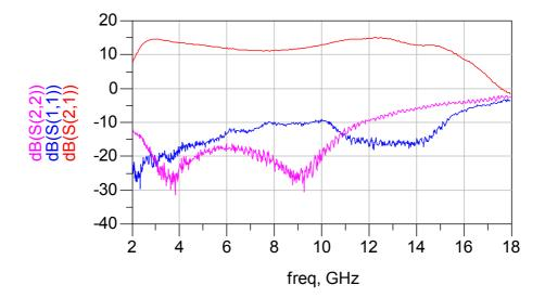
Figure 4.18 S-Parameters of the 2nd CRTSSDA Before Tunings
