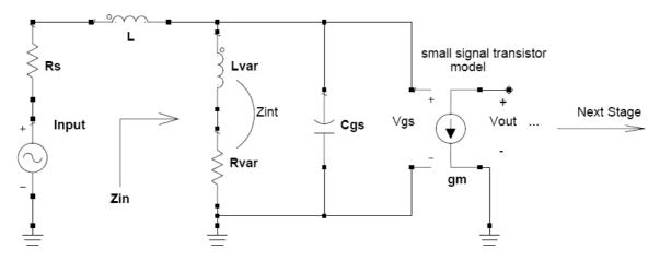
Figure 3.2 Small Signal Model of a Transistor with Reactive Terminations
