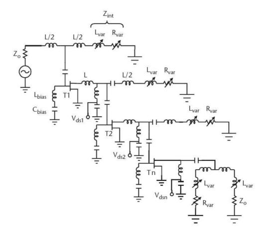
Figure 2.4 Cascaded Reactively Terminated Single Stage Distributed Amplifier [4]
