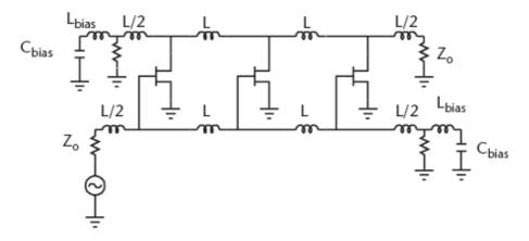
Figure 2.3 Traveling Wave Distributed Amplifier [4]
