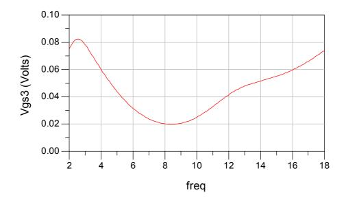
Figure 3.11 Voltage Swing Enhancement of The Third Stage
