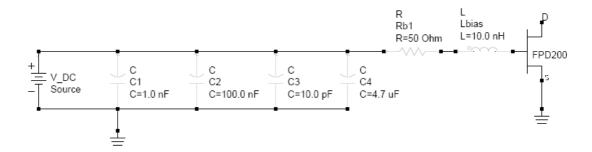
Figure 4.17 Gate Biasing of the First Stage of the 2nd CRTSSDA
