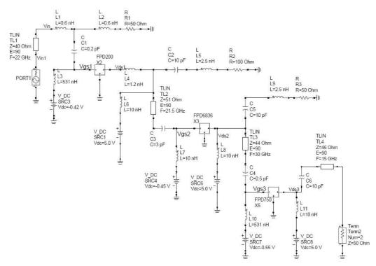
Figure 4.4 Schematic of the First Designed CRTSSDA
