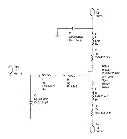
Figure A.1 TOM3 Model with External Parasitic of FPD200
