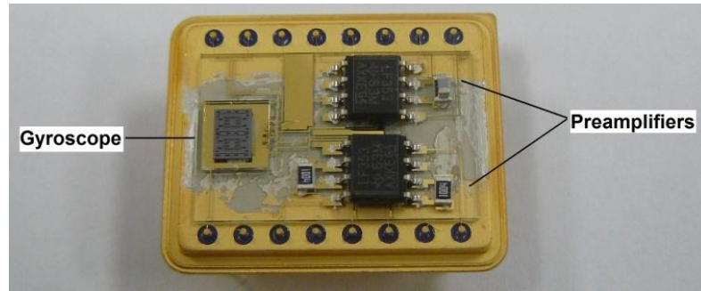
Figure 4.3: A gyroscope hybrid connected to preamplifiers on a platform package.
