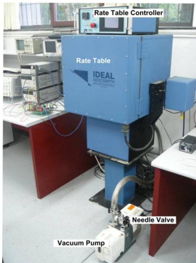
Figure 4.9: Vacuum pump, needle valve assembly externally connected to vacuum chamber of rate table.
