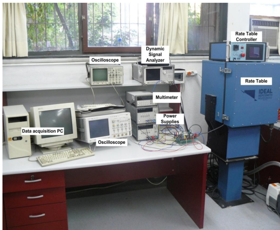
Figure 4.4: Test setup used for all tests under vacuum conditions.
