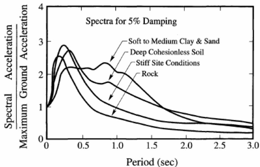
Figure 1.1 The mean acceleration spectra for different site conditions (Seed et al. 1976)
