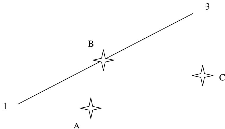
Figure 2.2 Typical site investigation plan view: Line 1-3 is the seismic line, point A is the seismograph station, point B is the center point of the seismic line, and point C is the borehole location
