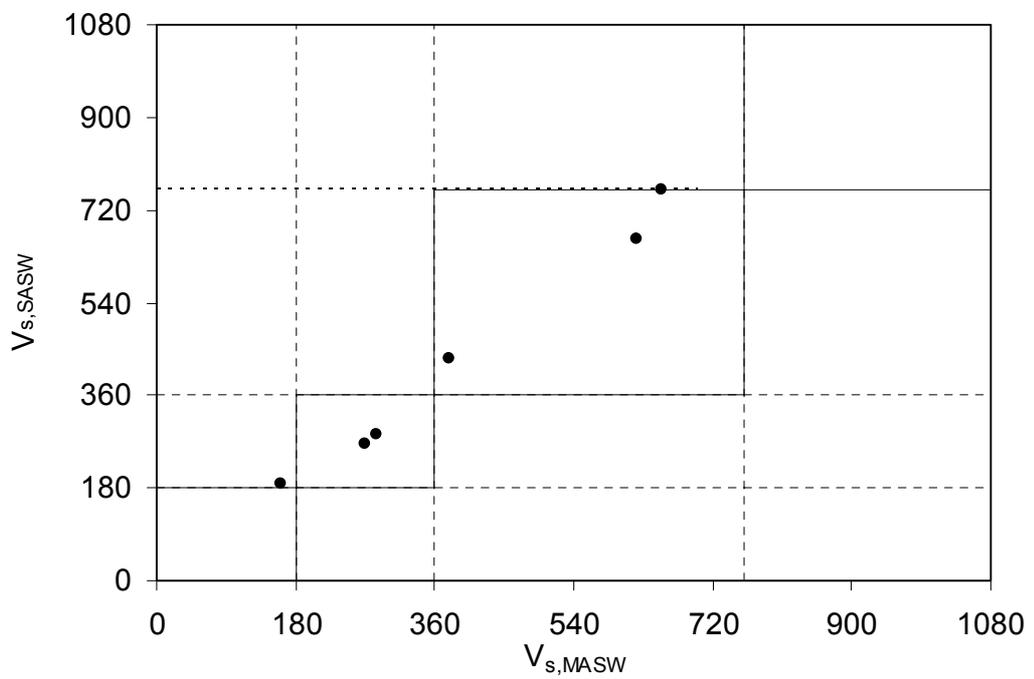
Figure 5.3 Comparison of mean  $V_s$  obtained by MASW and SASW
