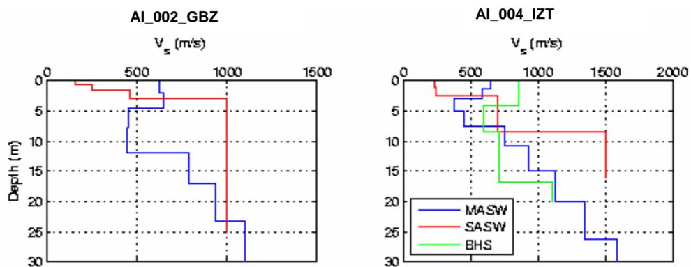
Figure 5.1 Comparison of  $V_s$  profiles obtained by MASW, SASW and BHS
