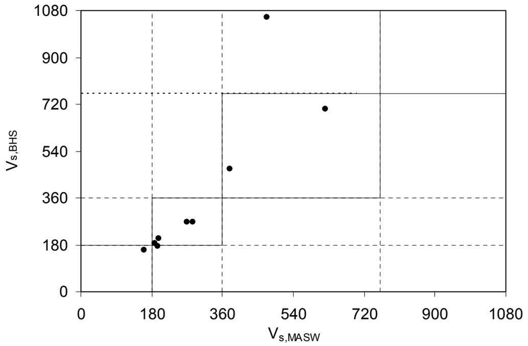
Figure 5.2 Comparison of mean  $V_s$  obtained by MASW and BHS
