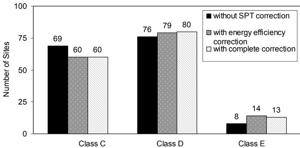
Figure 3.5 Comparison of site classes obtained without SPT correction, with energy efficiency correction, and with complete SPT correction procedure
