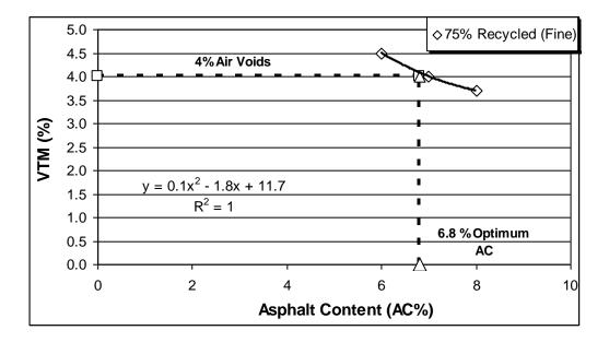
Figure 3.14 Optimum AC% calculation of a specimen with 75 % RCC
