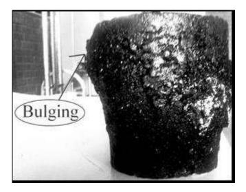
Figure 3.17 Bulging in a test specimen after rutting test
