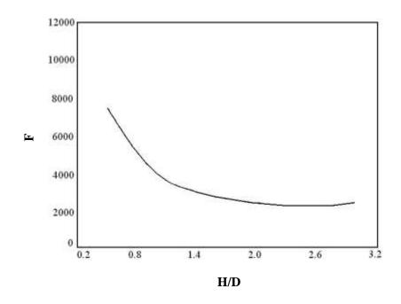
Figure 2.13 H/D ratio vs. flow number relationship (Witczak et al., 1999)
