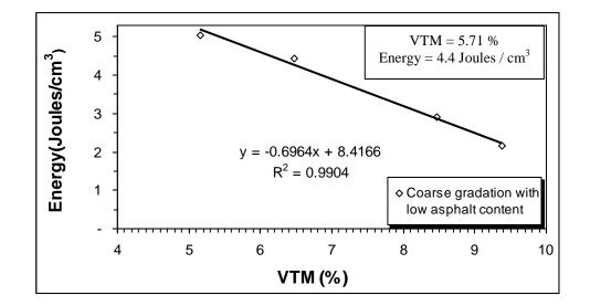
Figure A7 Graph for coarse graded tall specimen with low asphalt content,
