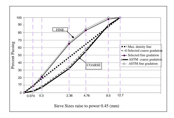
Figure 3.1 Gradations selected in accordance with ASTM D3515
