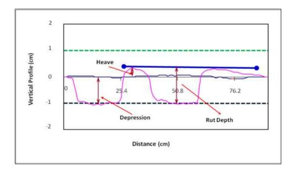
Figure 2.2 Rut profile example (Wu and Hossain, 2002)
