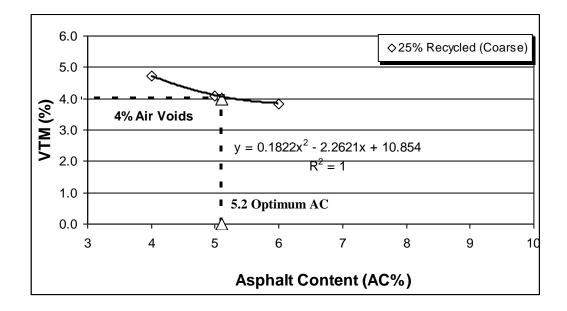
Figure D8 Optimum asphalt content calculation for coarse graded tall specimen with 25 % recycled cement concrete
