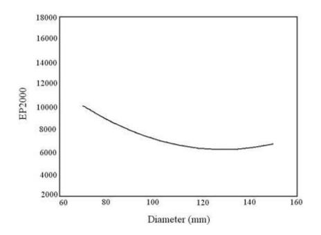
Figure 2.10 Change in permanent strain at 2000 cycles with specimen diameter (Witczak et al., 1999)
