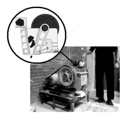
Figure 3.10 The crushing of recycled cement concrete aggregates with a jaw crusher
