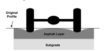
Figure 2.6 Rutting due to consolidation (Superpave Mix Design Superpave Series No. 2 (SP-2), Asphalt Institute)
