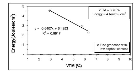
Figure A3 Graph for fine graded tall specimen with low asphalt content,
