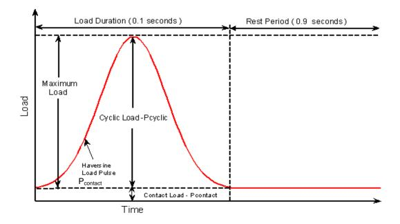
Figure 2.4 Haversine loading pattern applied in a permanent deformation test (National Cooperative Highway Research Program, Research Results Digest Number 285, 2004)
