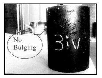
Figure 3.18 No bulging in a test specimen after rutting test (3iv is a number used to differentiate from other specimens)
