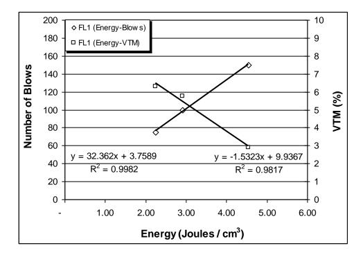
Figure A4 Graph for fine graded tall specimen with low asphalt content,
