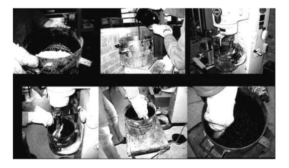
Figure 3.3 Mixing of asphalt and aggregate before compaction
