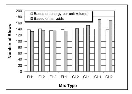
Figure 4.3 Number of blows calculated through two different methods
