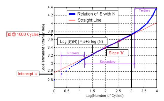
Figure 3.11 Calculation of slope, intercept and (E) @ 1000 cycles for fine graded tall specimen with 75 % RCC content
