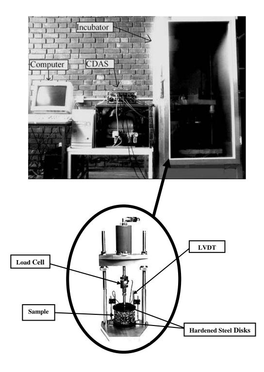
Figure 3.16 Repeated creep test setup
