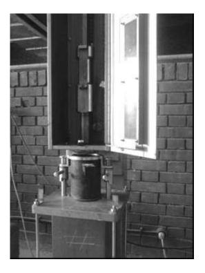
Figure 3.4 A picture of a standard Marshall compactor
