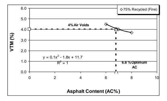
Figure D1 Optimum asphalt content calculation for fine graded tall specimen with 75 % recycled cement concrete
