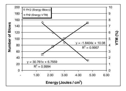
Figure A2 Graph for fine graded tall specimen with high asphalt content,
