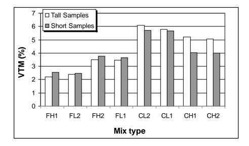
Figure 4.5 Relationship between air voids of tall and short specimens
