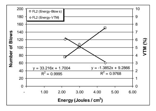
Figure A12 Graph for fine graded tall specimen with low asphalt content,
