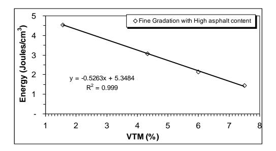
Figure 4.2 Graph for fine graded tall specimen with high asphalt content, replicate 1
