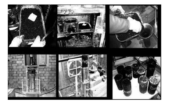
Figure 3.6 Typical steps in preparation of a modified Marshall specimen
