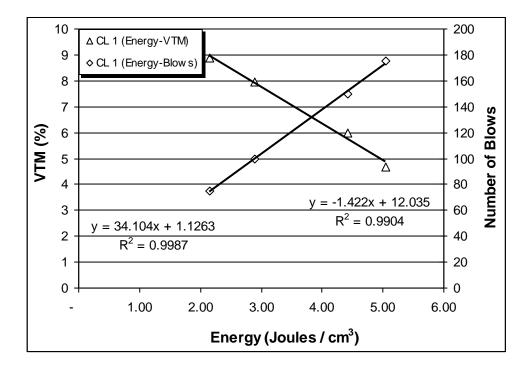
Figure A8 Graph for coarse graded tall specimen with low asphalt content,
