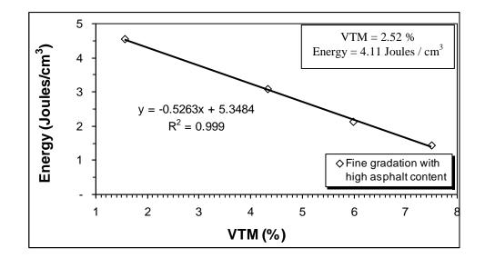
Figure A15 Graph for fine graded tall specimen with high asphalt content, replicate 1
