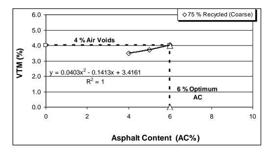
Figure D4 Optimum asphalt content calculation for coarse graded tall specimen with 75 % recycled cement concrete
