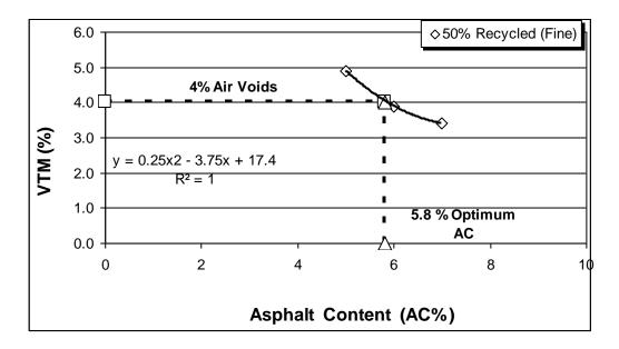
Figure D3 Optimum asphalt content calculation for fine graded tall specimen with 50 % recycled cement concrete
