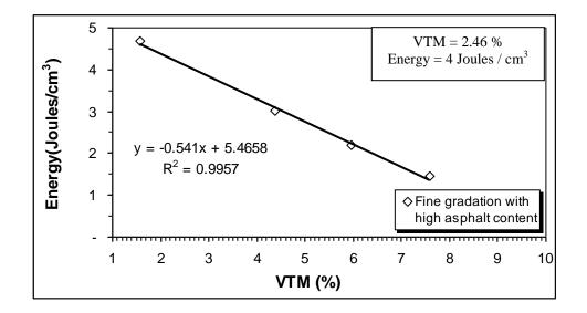
Figure A1 Graph for fine graded short specimen with high asphalt content,
