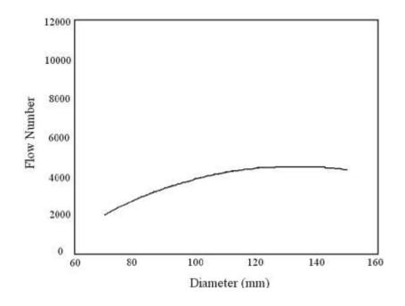
Figure 2.11 Effect of specimen diameter on flow number (Witczak et al., 1999)
