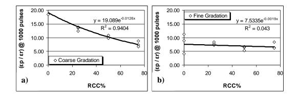
Figure 5.5  $\epsilon_p/\epsilon_r$  @ 1000 cycles vs. RCC content a) for coarse graded specimens, b) for fine graded specimens
