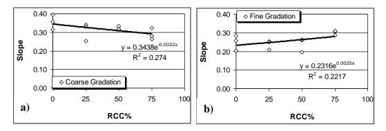
Figure 5.2 Slope constant vs. RCC content a) for coarse graded specimens, b) for fine graded specimens
