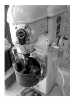
Figure 3.2 Mixer used for mixing bitumen with blended aggregates
