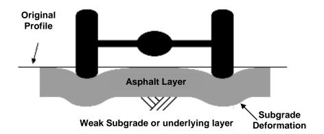
Figure 2.9 Structural rutting (Superpave Mix Design Superpave Series No. 2 (SP-2), Asphalt Institute)
