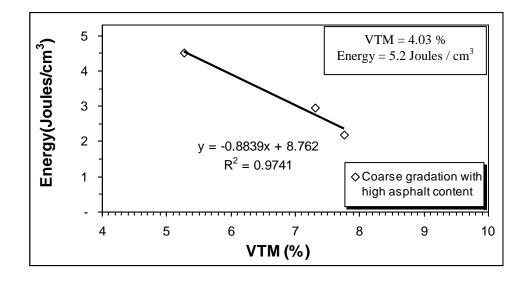
Figure A13 Graph for coarse graded tall specimen with high asphalt content,
