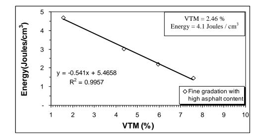
Figure A11 Graph for fine graded tall specimen with high asphalt content,
