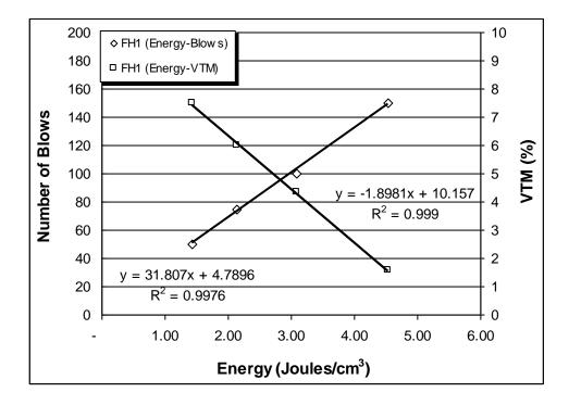
Figure 4.1 Graph for fine graded modified Marshall specimen with high asphalt content, replicate 1
