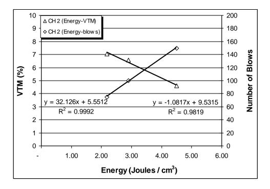
Figure A6 Graph for coarse graded tall specimen with high asphalt content,
