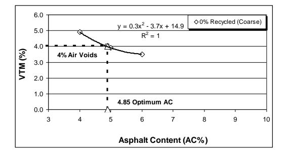
Figure D7 Optimum asphalt content calculation for coarse graded tall specimen with 0 % recycled cement concrete
