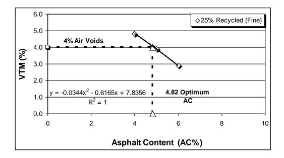
Figure D6 Optimum asphalt content calculation for fine graded tall specimen with 25 % recycled cement concrete
