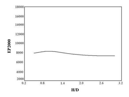
Figure 2.12 Change in permanent strain at 2000 cycles with H/D ratio (Witczak et al., 1999)
