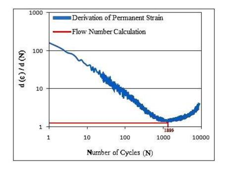
Figure 3.12 Calculation of flow number for fine graded specimen with 75 % RCC content
