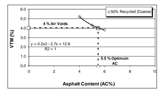
Figure D2 Optimum asphalt content calculation for coarse graded tall specimen with 50 % recycled cement concrete
