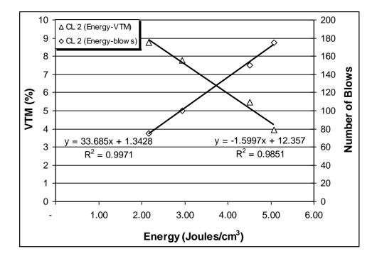
Figure 4.4 Graph for coarse graded tall specimen with low asphalt content, replicate 2
