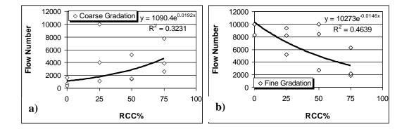
Figure 5.1 Flow number vs. RCC content a) for coarse graded specimens, b) for fine graded specimens
