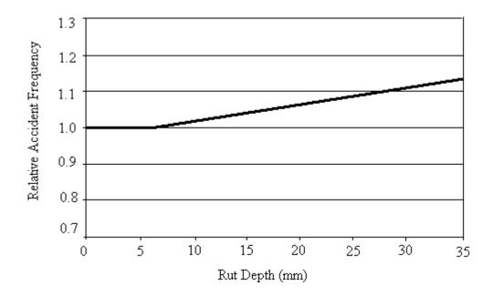
Figure 2.1 Rut Depth vs. Relative Accident Frequency (Optimal Road Maintenance and Operations – Results of New Research and Analysis in Norway" NORDIC Road and Transportation Research NPRA, Norway, 2002)
