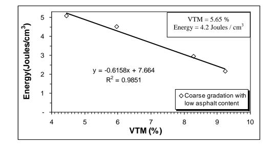
Figure A9 Graph for coarse graded tall specimen with low asphalt content,
