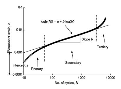
Figure 2.5 Permanent strain vs. number of cycles in log–log scale (Kanitpong et. al., 2006)
