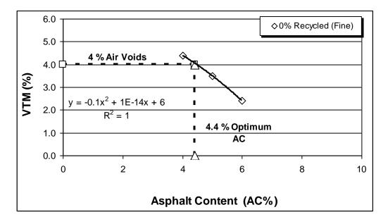
Figure D5 Optimum asphalt content calculation for fine graded tall specimen with 0 % recycled cement concrete
