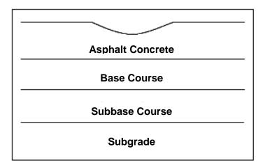
Figure 2.7 Rutting due to surface wearing (Ozturk, 2007)
