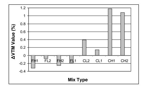
Figure 4.7 Values of the difference between air voids of tall and short specimens
