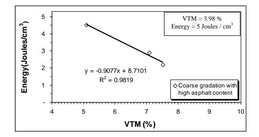
Figure A5 Graph for coarse graded tall specimen with high asphalt content,
