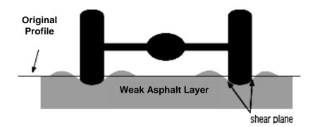
Figure 2.8 Rutting due to plastic flow (Superpave Mix Design Superpave Series No. 2 (SP-2), Asphalt Institute)
