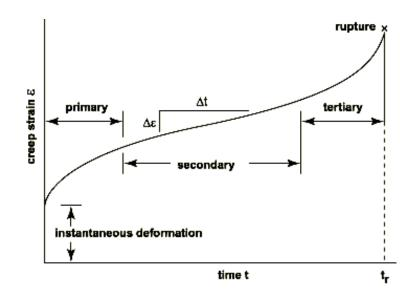
Figure 2.3 Creep Curve (Martin Tarr, "Stress and its effect on materials")
