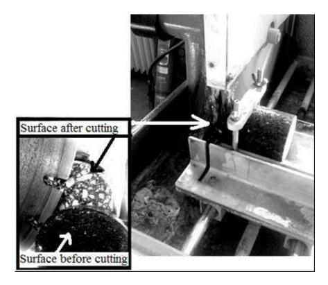
Figure 3.15 Specimen cutting process
