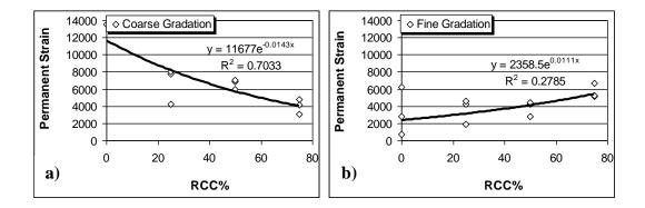
Figure 5.4 Permanent strain @ 1000 cycles vs. RCC content a) for coarse graded specimens, b) for fine graded specimens
