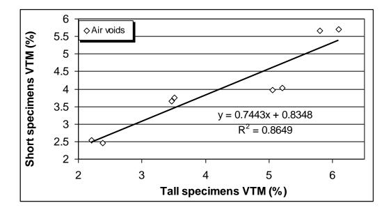
Figure 4.6 Comparison of air voids for tall (modified) and short (standard) specimens
