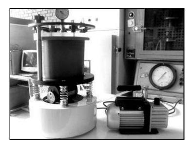
Figure 3.8 A picture of Rice test measurement system
