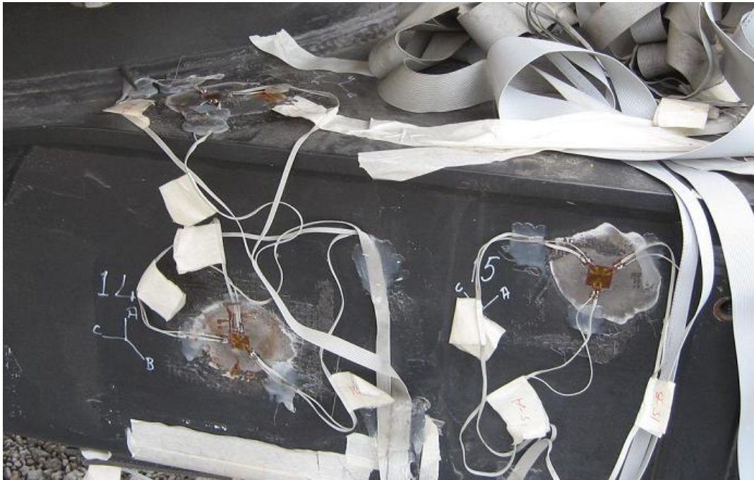
Figure 3.11 – The strain gauges used in the test
