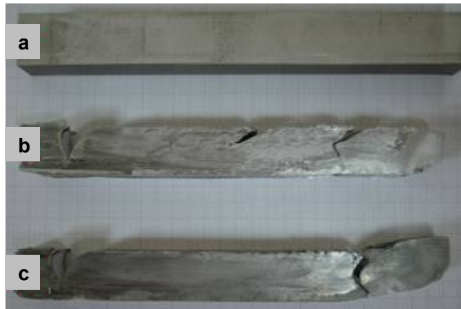
Figure 3.9 Photographs of 5083 Al-alloy specimens in (a) unECAPed (b) ECAPed (c) Annealed (415°C / 144h) + ECAPed conditions.
