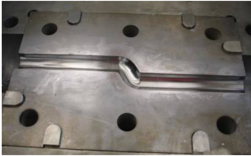
Figure 3.13 ECAP die with double 120° channel angle having cross-section with 18 mm \Phi .
