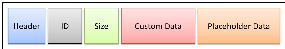
Figure 15 MMOG Data Packet Structure
