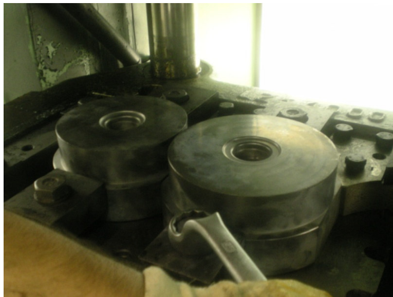
Figure 5.7 View of Clamping of Lower Finish Die
