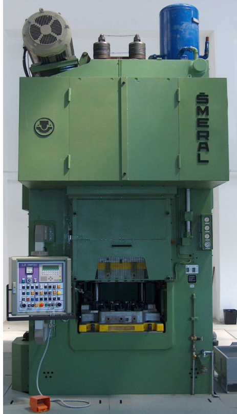
Figure 5.1 1000-ton SMERAL Mechanical Press Available in METU-BILTIR Center Forging Research and Application Laboratory [18]
