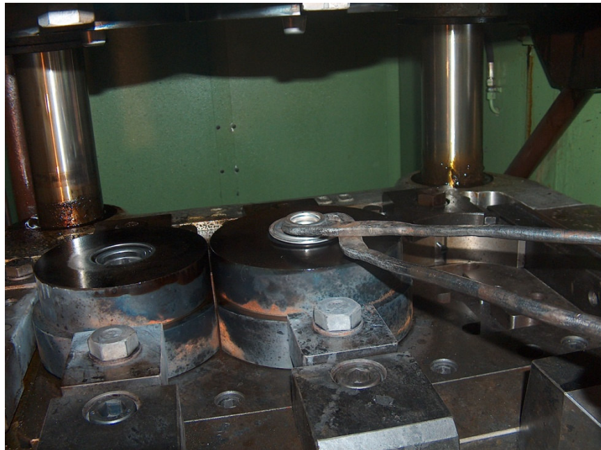
Figure 5.14 View of Finish Part Taken by Tongs
