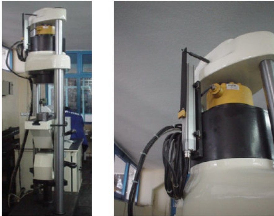
Figure 4.5 40 tons Tensile Test Machine (left), Displacement Sensor (right)
