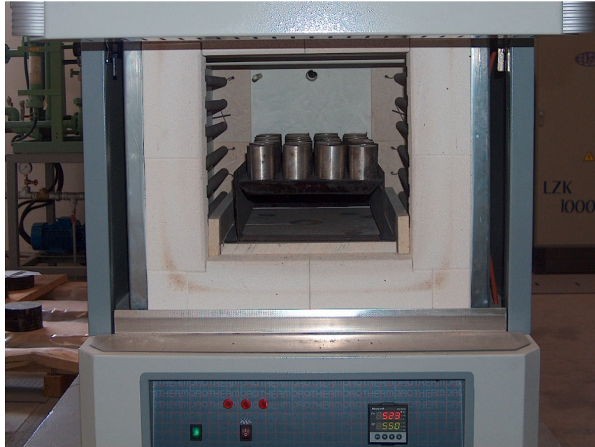
Figure 5.9 View of Billets in Electric Furnace
