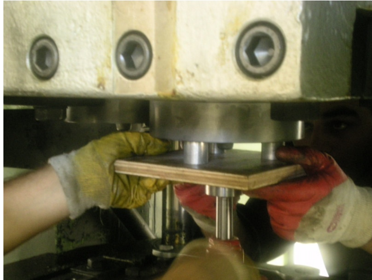
Figure 5.6 View of Lifting of the Upper Finish Die by Hydraulic Jack
