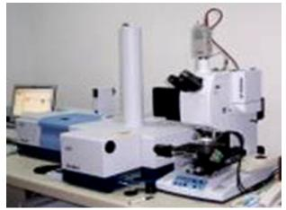
Figure 2.4 FTIR Spectrometer with ATR objective
