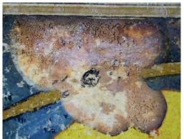
Figure 1.11 Corroded white lead pigment, black colored regions show occurence of PbS
