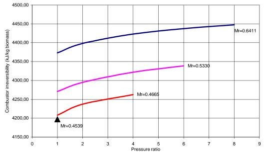
Figure 5. 35 : Combustor irreversibility vs pressure ratio
