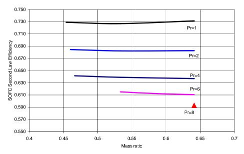
Figure 5. 14 : SOFC second law efficiency vs mass ratio
