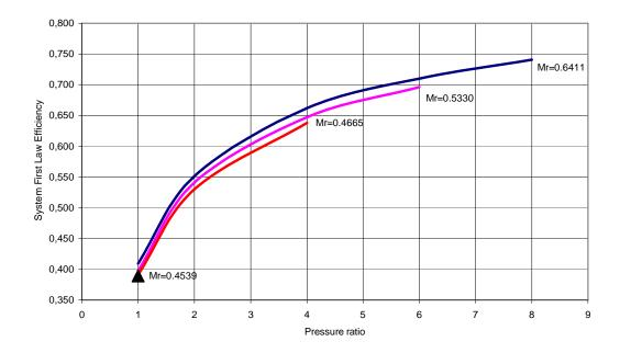
Figure 5. 26 : System first law efficiency vs pressure ratio
