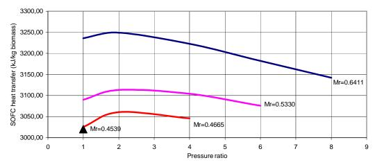
Figure 5. 27 : SOFC required heat transfer vs pressure ratio
