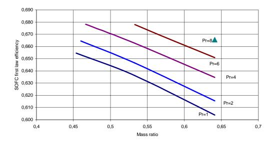
Figure 5. 4 : SOFC first law efficiency vs mass ratio
