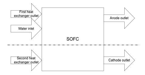
Figure 4. 2: SOFC inlet and outlet flows
