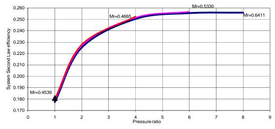
Figure 5. 30 : System second law efficiency vs pressure ratio
