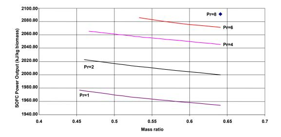
Figure 5. 7 : SOFC power output vs mass ratio
