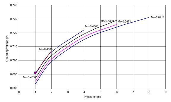
Figure 3. 1 : SOFC Operating voltages vs pressure ratio
