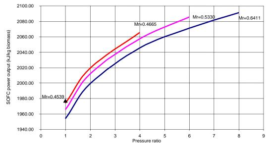
Figure 5. 22 : SOFC power output vs pressure ratio
