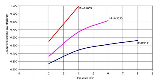
Figure 5. 37 : GT second law efficiency vs pressure ratio
