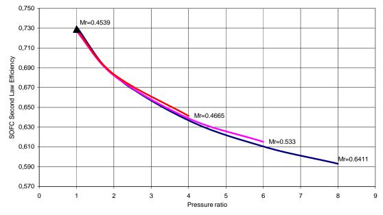
Figure 5. 33 : SOFC second law efficiency vs pressure ratio
