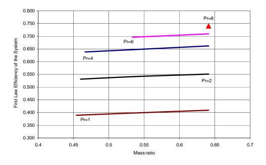
Figure 5.1: First law efficiency of the system vs mass ratio
