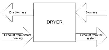
Figure 4. 1: Dryer inlet and outlet flows
