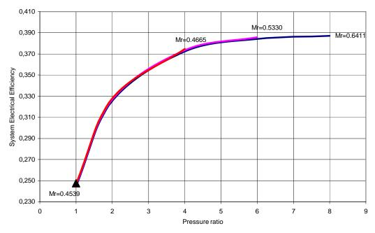
Figure 5. 21 : System electrical efficiency vs pressure ratio
