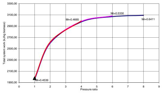
Figure 5. 20 : Total system power output vs pressure ratio
