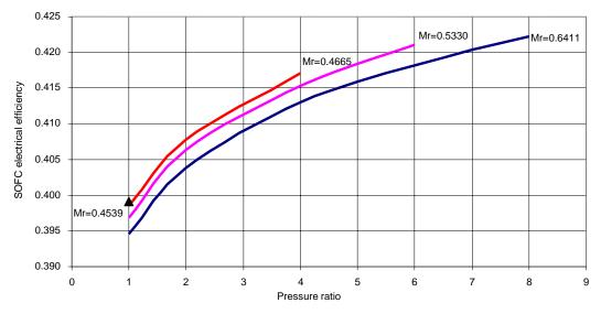
Figure 5. 23 : SOFC electrical efficiency vs pressure ratio
