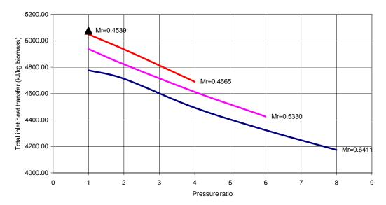
Figure 5. 25 : Total inlet heat transfer vs pressure ratio
