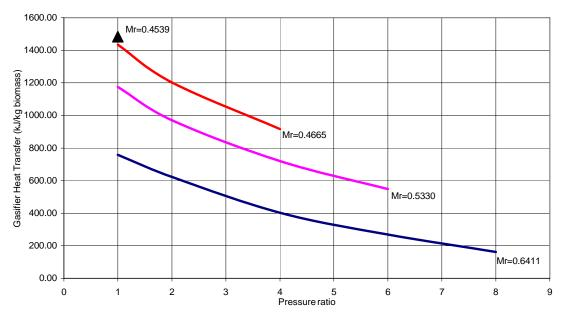
Figure 5. 29 : Gasifier required heat transfer vs pressure ratio
