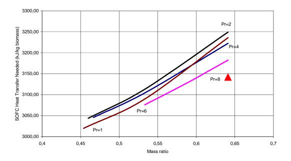
Figure 5. 9 : SOFC required heat transfer vs mass ratio
