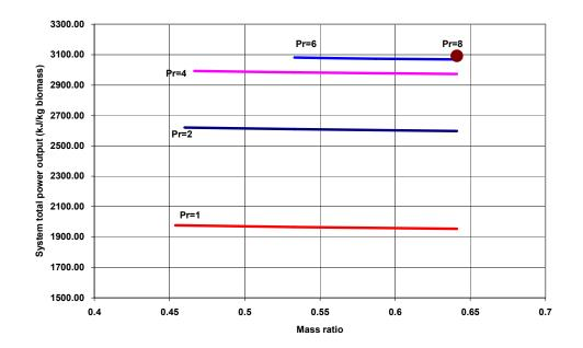
Figure 5. 5 : System total power output vs mass ratio
