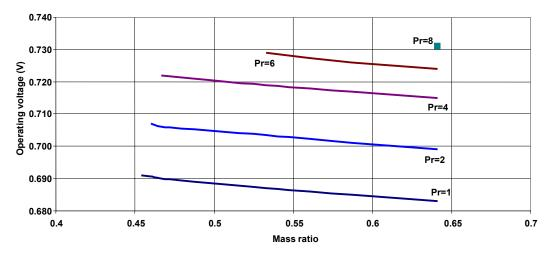
Figure 3. 2 : SOFC Operating voltages vs mass ratio
