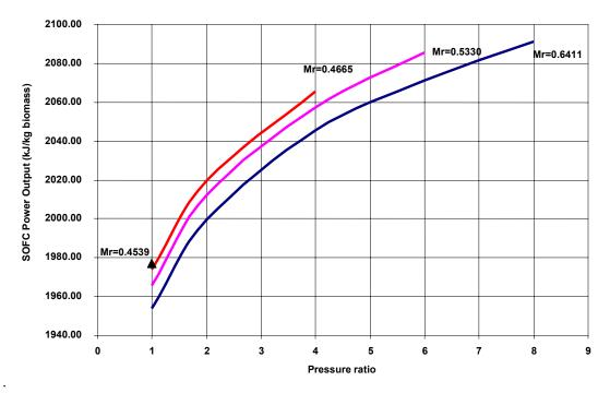
Figure 5. 6 : SOFC power output vs pressure ratio
