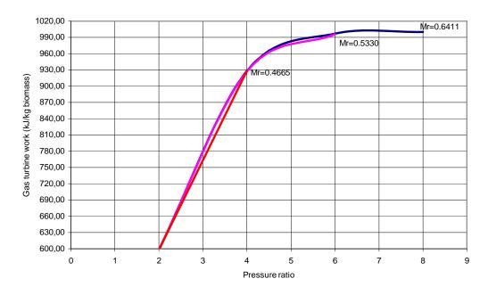
Figure 5. 24 : GT power output vs pressure ratio
