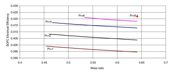
Figure 5.3: SOFC electrical efficiency vs mass ratio
