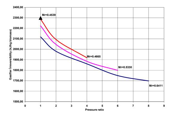
Figure 5. 36 : Gasifier irreversibility vs pressure ratio
