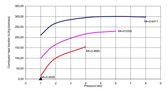
Figure 5. 28 : Combustor required heat transfer vs pressure ratio
