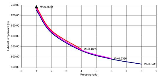
Figure 5. 31: Exhaust temperature vs pressure ratio
