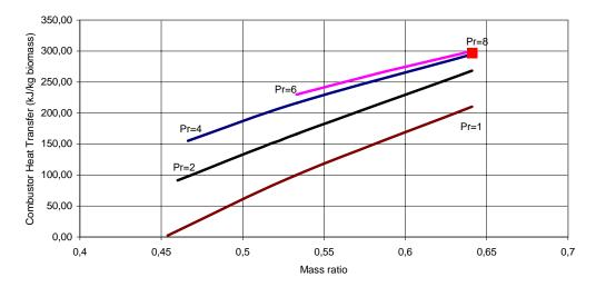
Figure 5. 10 : Combustor required heat transfer vs mass ratio
