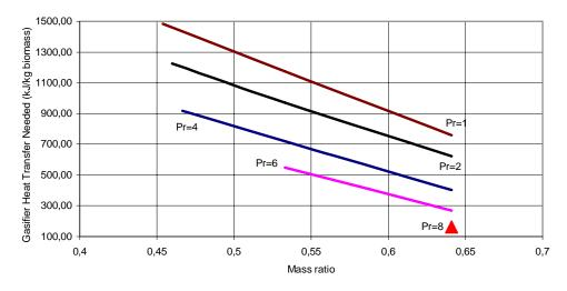
Figure 5. 11 : Gasifier required heat transfer vs mass ratio
