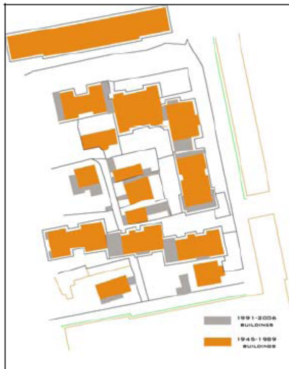
Figure 4: Extension of the ground floors around the existing building blocks in a residential neighborhood of Tirana after 1991 (Source: Author, Odeta Durmishi)
