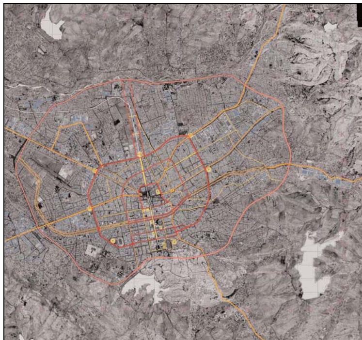
Figure 60: Road System proposed by Architecture Studio, Legend: in red: the inner ring roads; in rose: the outer peripheral road; in orange: roads radiating from the centre; in yellow: pedestrian roads (Architecture Studio unpublished Report, p. 47)
