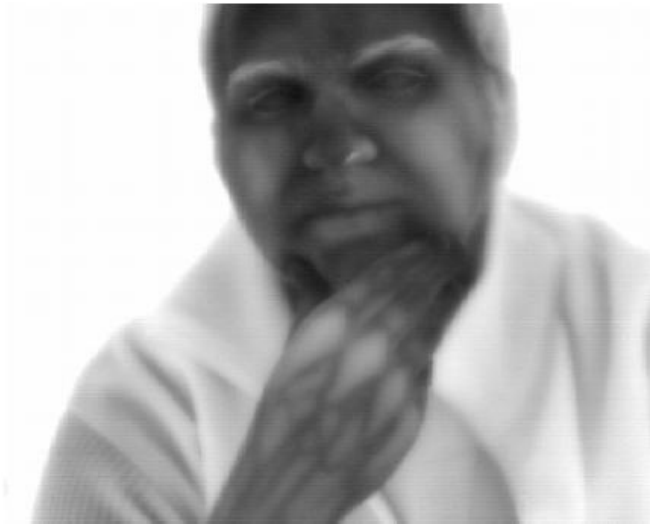
Figure 25: 640×512 image of a person taken with the InP based MWIR detector operating at 80 K
