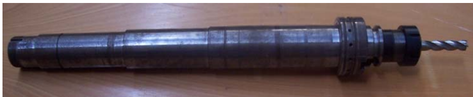
Figure 3.4 Spindle – holder – tool assembly used in experiments.
