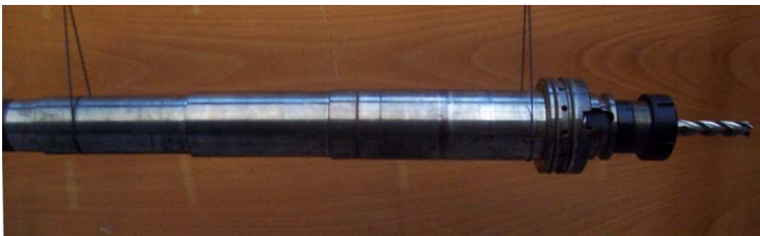
Figure 3.5 Free free suspended spindle-holder-tool assembly.
