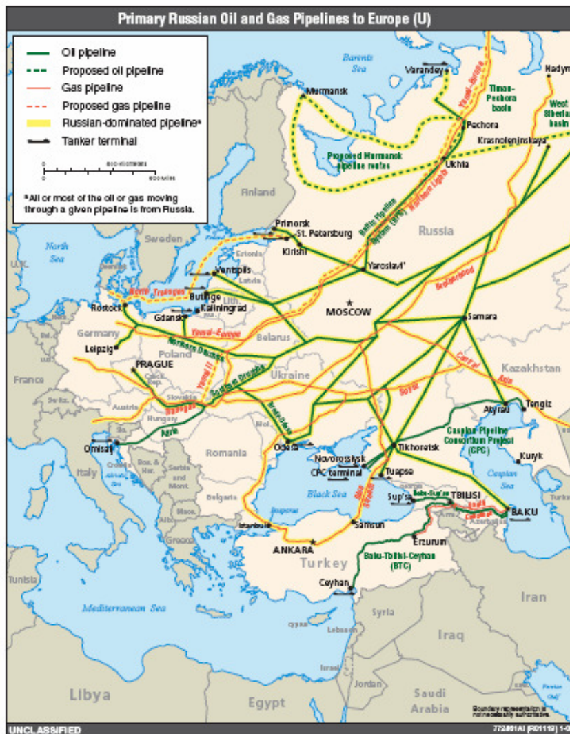
Figure 2: Primary Russian Oil and Gas pipelines to Europe 256
