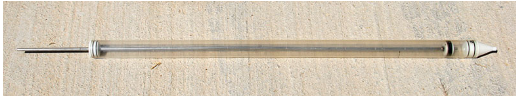
Figure 2.6: Syringe sampler used to take water samples in enclosures with minimum possible disturbance on periphyton and sediment. It is made of plexyglass tube with 4 cm diameter and one 1 m length and have 1 l sample capacity. It works like a piston and sucks up water through an opening with 4 mm diameter at desired depth.
