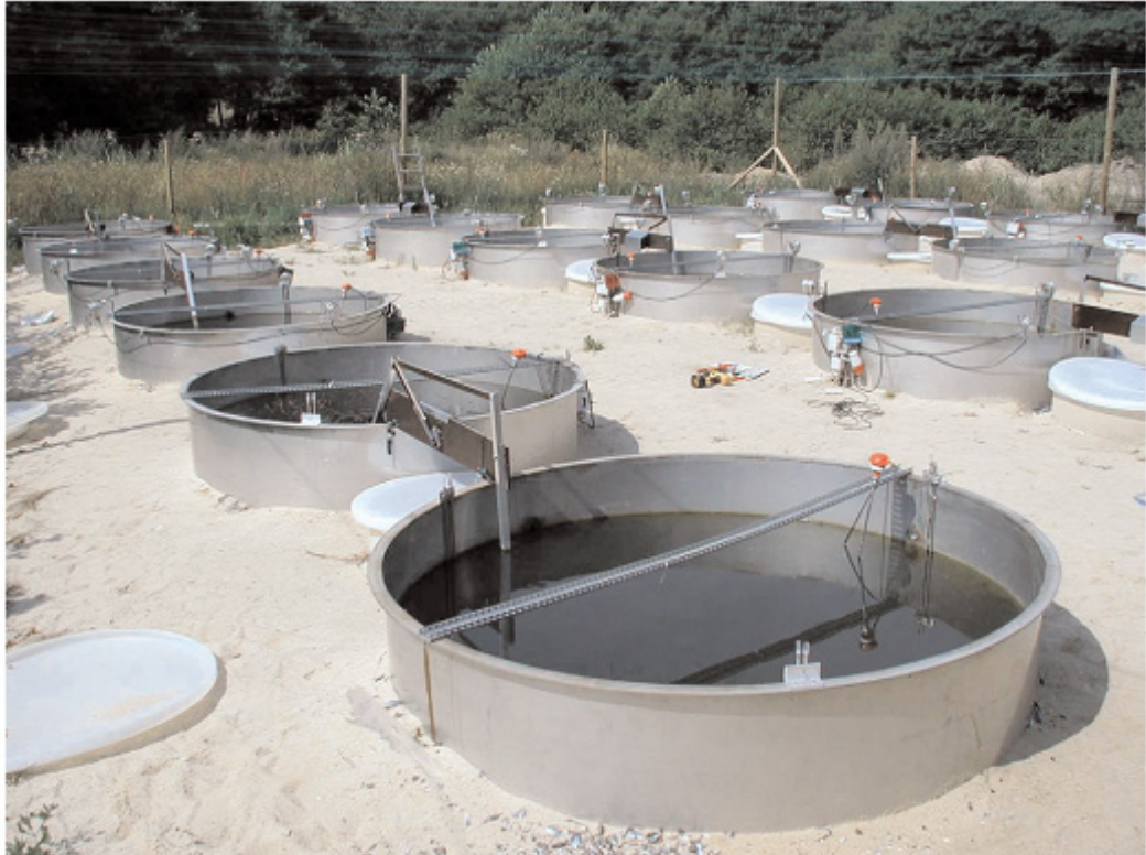
Figure 1.6: A large-scale ex situ mesocosm experiment setup at National Environmental Research Institute, Denmark. This fully automatized system enables automatic sampling and temperature manipulation in 24 enclosures stocked with natural lake sediment. Whole setup is reported to cost 140.000 €, excluding construction and maintenance labor. Photograph and information are taken from Liboriussen et al. (2005b).
