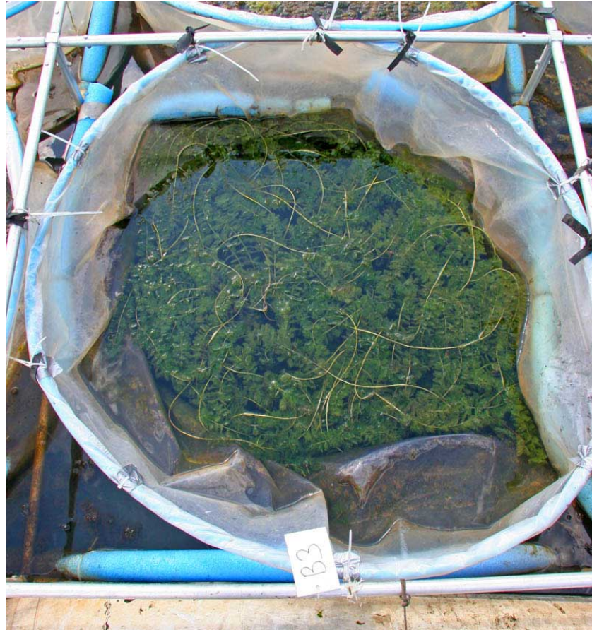
Figure 3.21: Photograph of macrophyte growth in enclosures at the end of the experiment. Full surface coverage and 50% PVI observed in enclosures.
