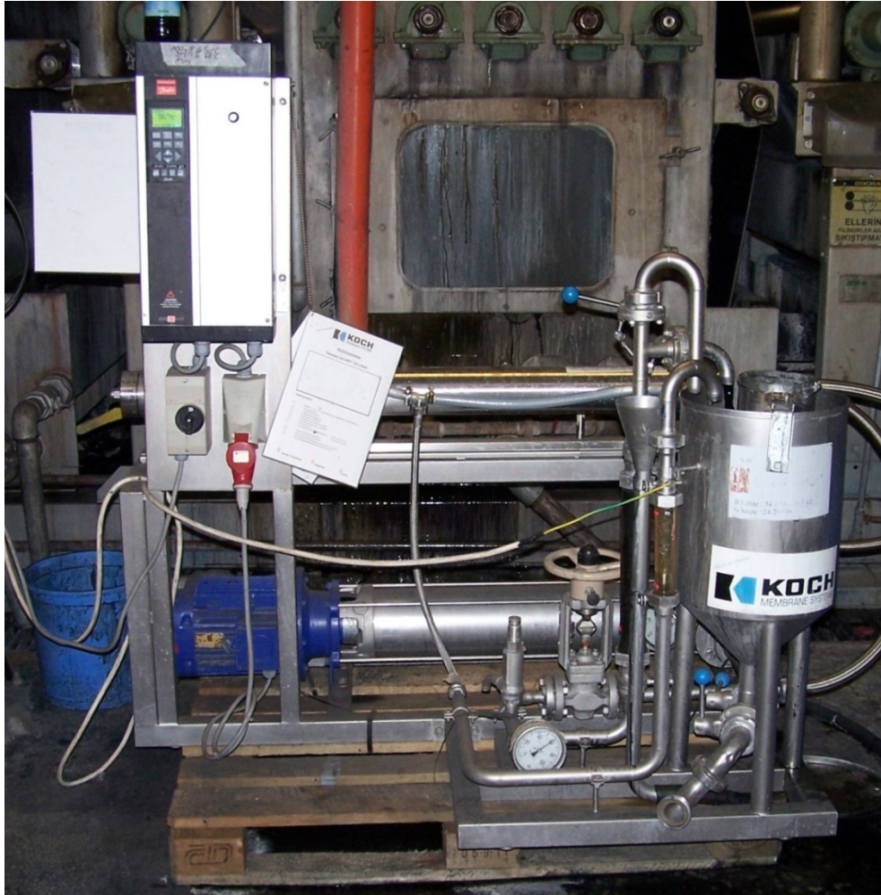
Figure 3.4 SelRO MPT34 Pilot Plant set up in the mercerizing unit of the mill
