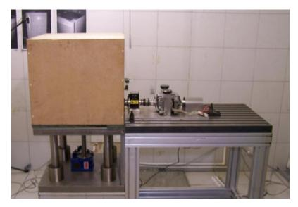
Figure 162 SRM test bed with noise attenuation cabinet
