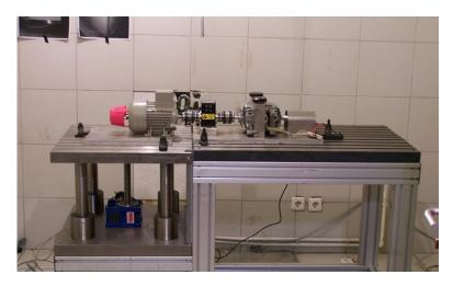
Figure 160 Test setup used for loading SRM during sound measurements.
