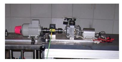
Figure 176 The test motor (SR3) and the mechanical load.
