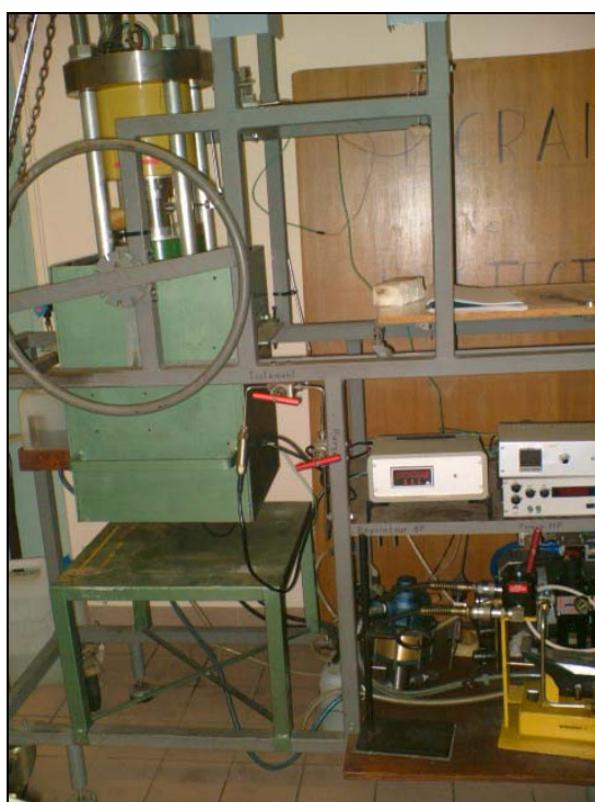
Fig. III.5. HHP equipment with indirect compression system used for HPCD experiments
