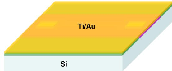
Deposit 200+2000 $\text{\AA}$  Ti/Au by sputter.
