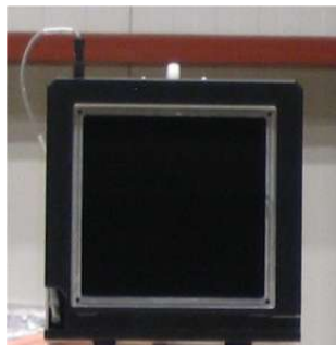
Figure 4-2 Blackbody Device without Mask (Experiment 1)
