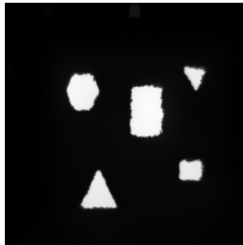
Figure 4-4 Typical Infrared Image of Blackbody Device with Mask (Experiment 1)
