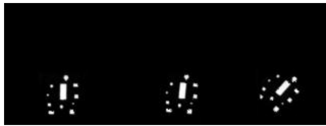
Figure 4-68 MWIR Band Infrared Images with 150°C Blackbody at 43m.
