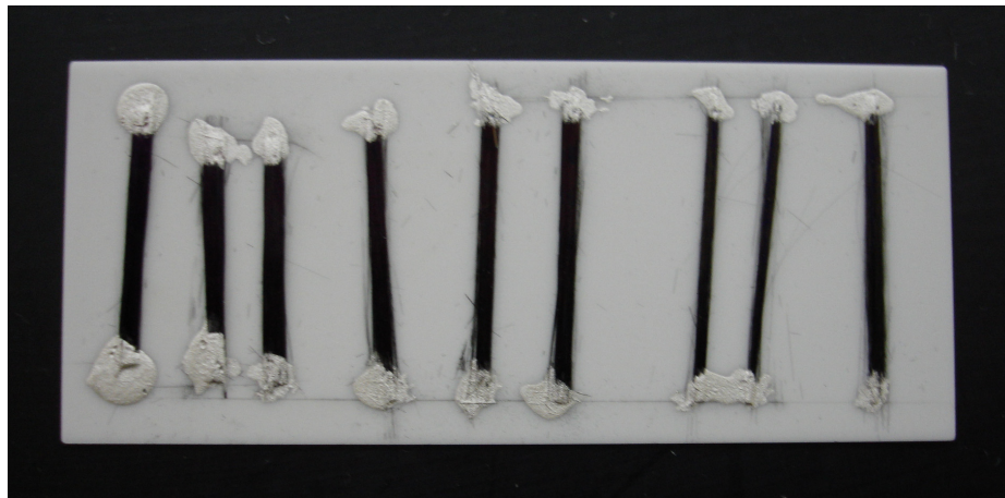
Figure 3.3 Bundle preparation step for electrical conductivity measurement.
