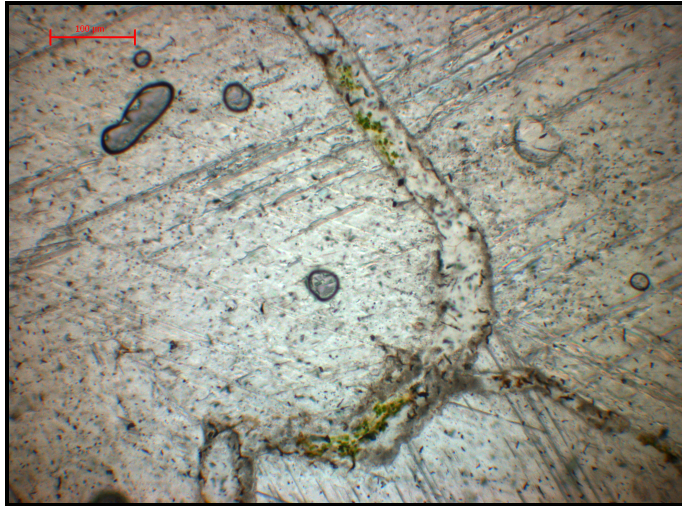
Figure 3. 18 Thin section view of Pessinous quarry marble (PM3U) showing biological activity in intergranular and intragranular zones of calcite grains, (20X, single nicol).
