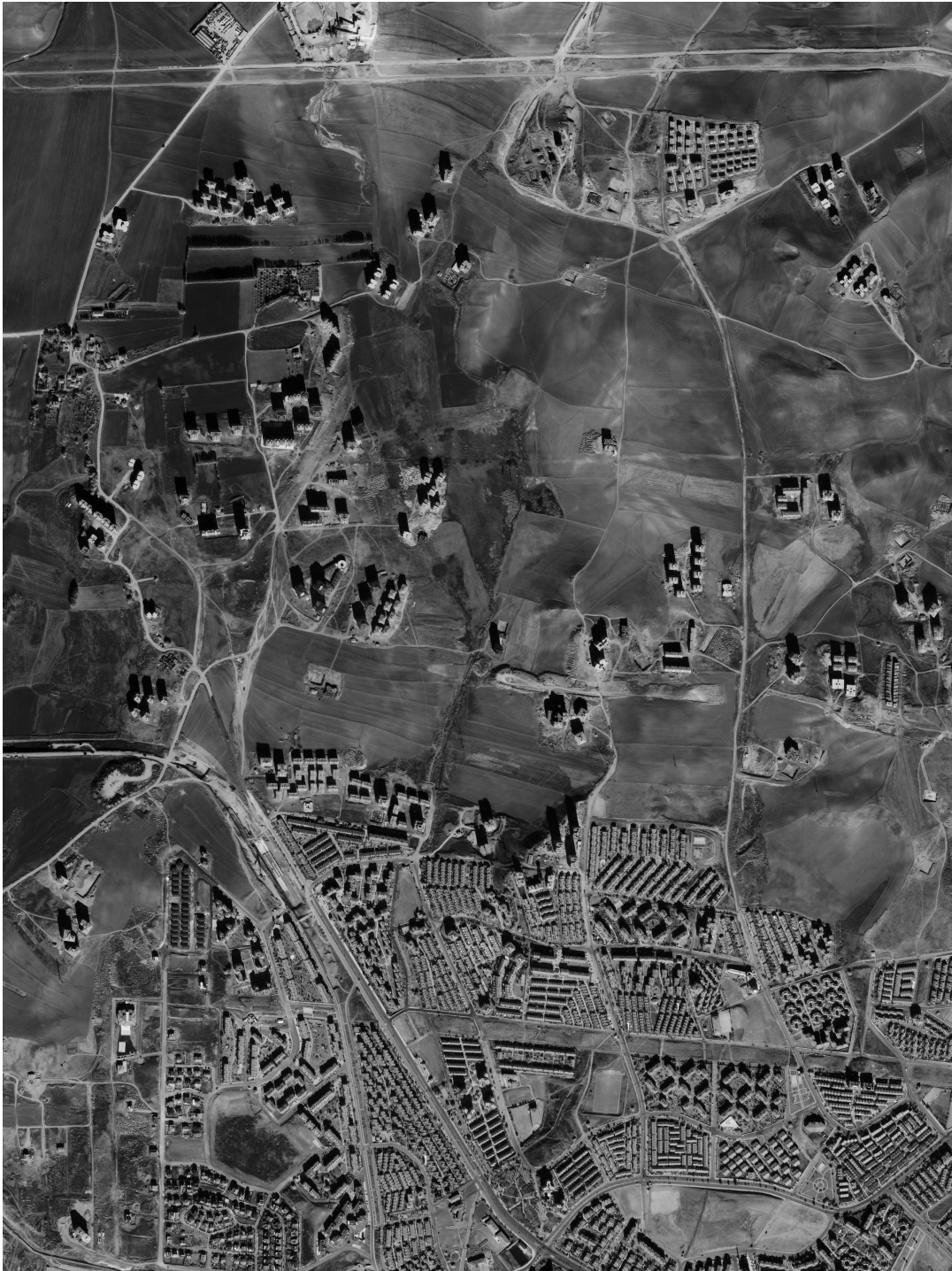
Figure 5.4: A panchromatic SPOT image. Image size is 3200x2400 and spatial resolution is 10 meters per pixel.
