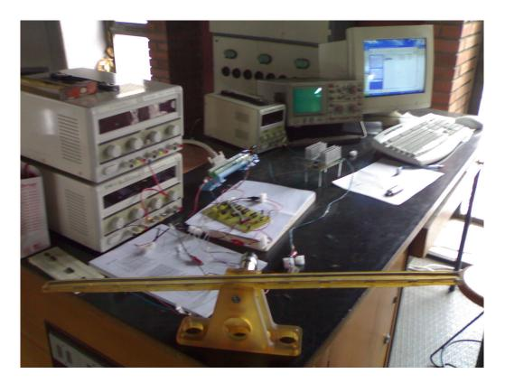
Figure 6. 2 Beam & Ball System
