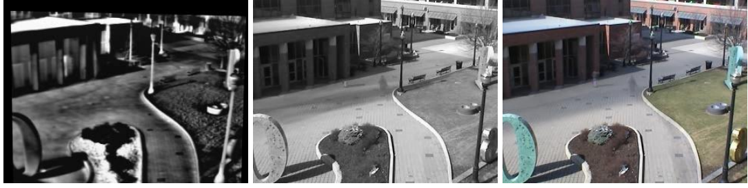
Figure 3-5 Mean Images of Infrared, Color Intensity and Color Channels of Single Gaussian Background Method
