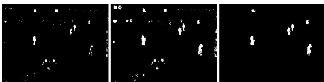
Figure 3-33 Foreground Region of Infrared, Resulting Final Foreground Region and Application of Snake Algorithm
