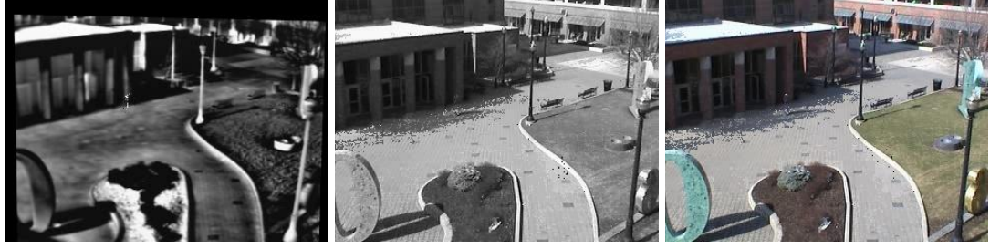
Figure 3-12 Mean Images of Infrared, Color Intensity and Color Channels of Mixture of Gaussian Background Method
