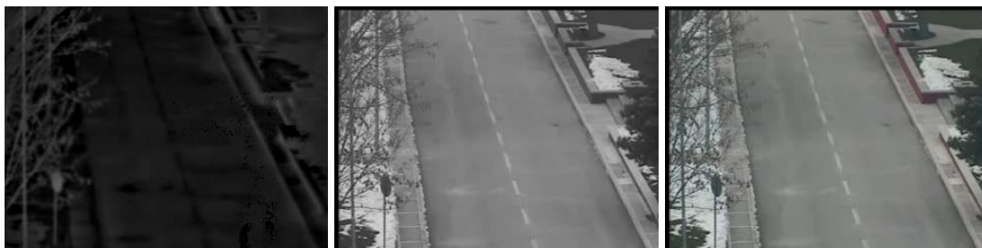
Figure 4-3 Mean Images of Infrared, Color Intensity and Color Channels of Mixture Gaussian Background Method
