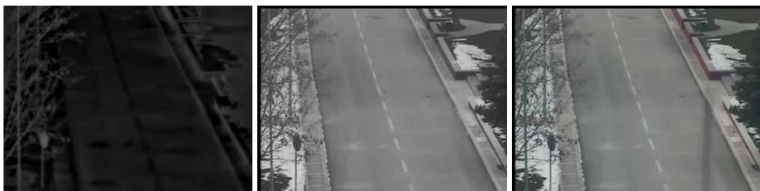
Figure 4-2 Mean Images of Infrared, Color Intensity and Color Channels of Single Gaussian Background Method
