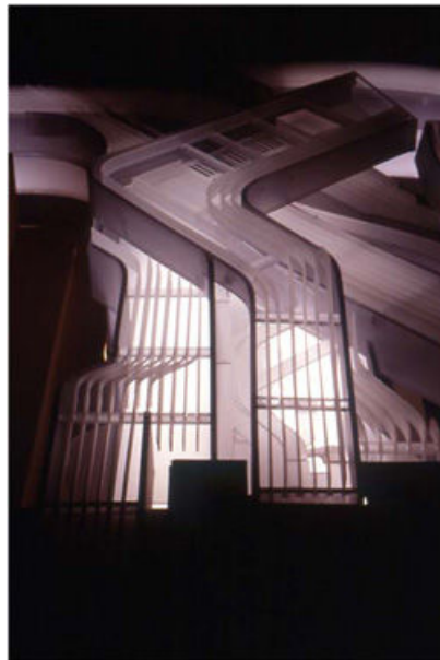
Figure 6. The model of Zaha Hadid’s New Center for Contemporary Arts in Rome. Built by Ademir Volic. He used materials as perspex, acrylic and Urial. CNC technologies are also employed in this model.
