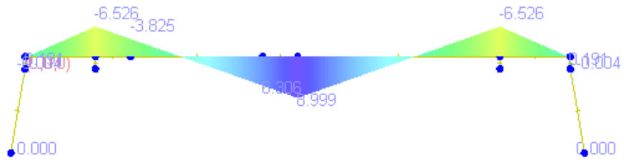
a) Linear Elastic Analysis (P=27 kN)
