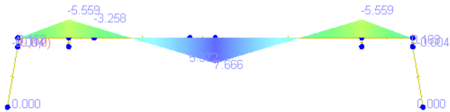
a) Linear Elastic Analysis (P=23 kN)
