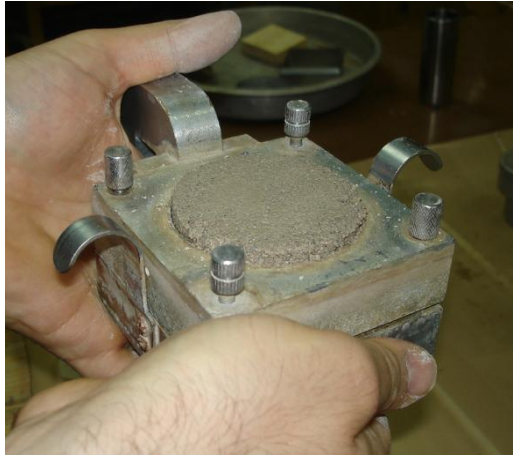
Figure 3.26 The sample is placed into the shear box
