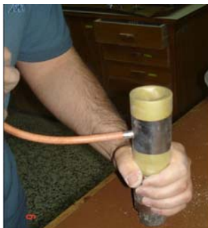
Figure 3.21 Sample is carried on the base pedestal of the cell
