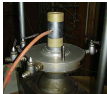
Figure 3.21 Sample is carried on the base pedestal of the cell
