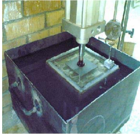
Figure 3.24 Plexiglas box in water tank is placed under loading jack
