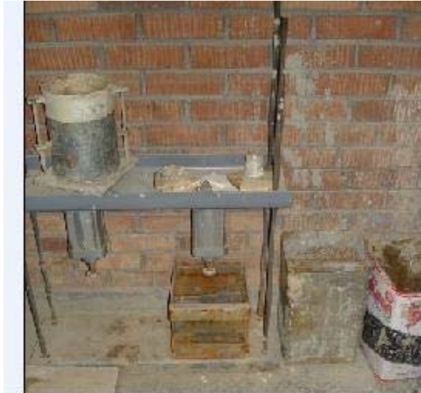
Figure 3.2 Loading frame and jack system
