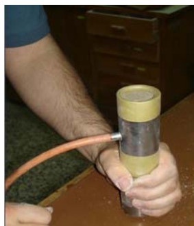
Figure 3.21 Sample is carried on the base pedestal of the cell
