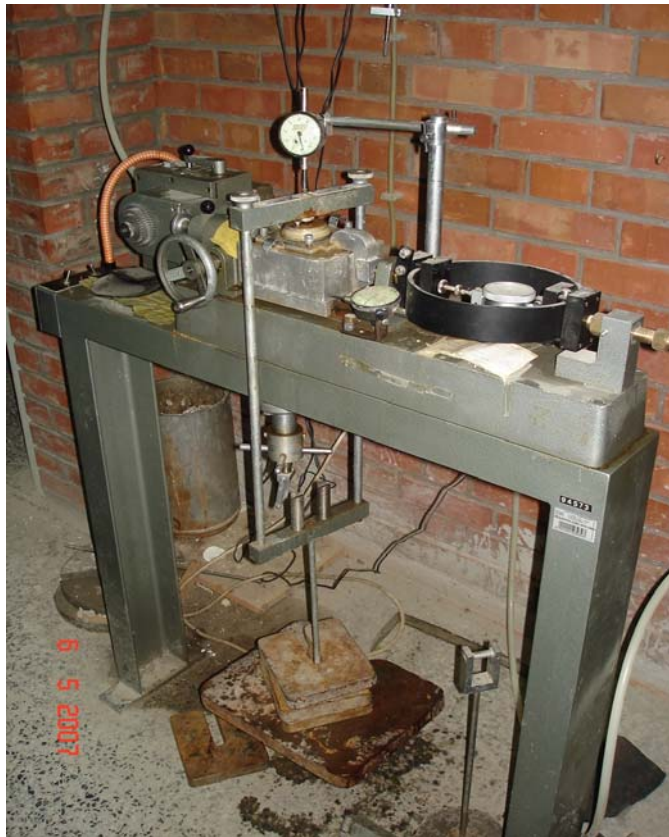
Figure 3.27 Direct shear test machine during shear
