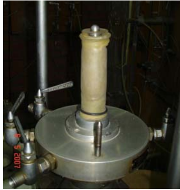
Figure 3.22 Sample is mounted on the base pedestal of the cell
