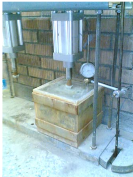
Figure 3.17 Plexiglas box is placed under loading jack with displacement dial
