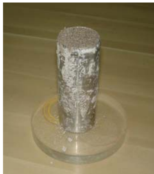
(b) Steel sampling mold after taking sample
