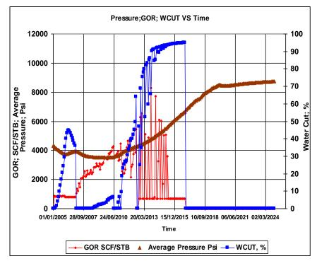
Figure 5. 16 Average Pressure, Water cut and GOR for the Base Case of the South Flank region
