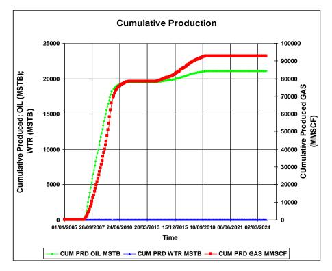
Figure 6. 45 Cumulative Produced Gas, Oil, and Water from SP3 well of the Scenario 52
