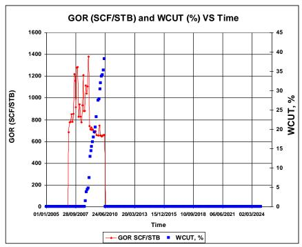
Figure 5. 28 GOR and Water cut for SP4 well of the Base Case
