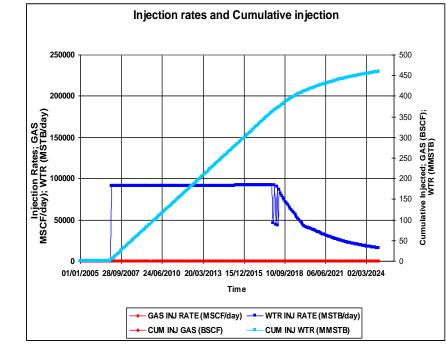
Figure 5. 17 Injection Rates and Cumulative Injection for Base Case of the South Flank region
