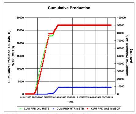
Figure 5. 26 Cumulative Produced Gas, Oil, and Water from SP3 well of the Base Case
