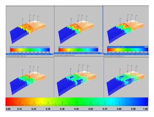
Figure 6. 11 Water saturation map showing down flow of water during injection for Scenario 53
