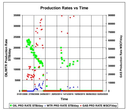
Figure 6. 26 Gas, Oil, Water Production rates for SP4 well of the Scenario 53
