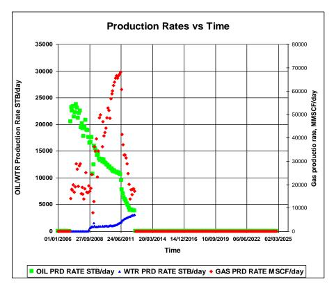
Figure 6. 46 Gas, Oil, Water Production rates for SP4 well of the Scenario 52
