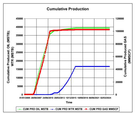
Figure 5. 20 Cumulative Produced Gas, Oil, and Water from SP1 well of the Base Case
