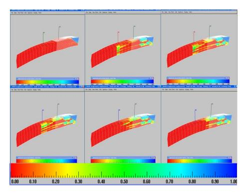
Figure 6. 12 Gas saturation map showing upper segregation of gas during injection for Scenario 53
