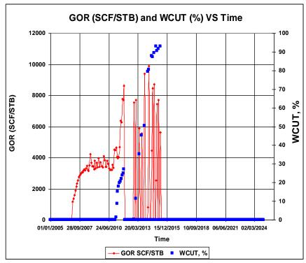
Figure 5. 22 GOR and Water cut for SP2 well of the Base Case
