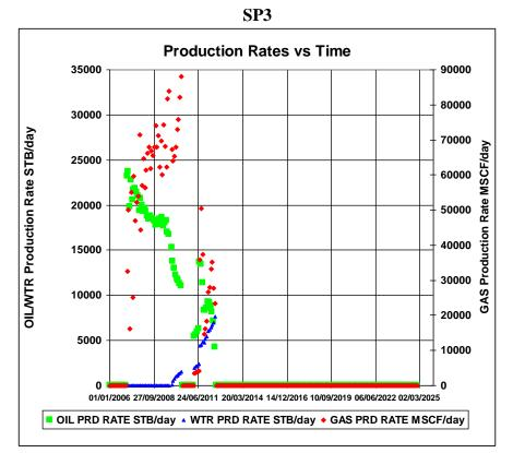
Figure 5. 24 Gas, Oil, Water Production rates for SP3 well of the Base Case
