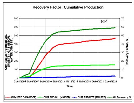
Figure 6. 6 Recovery Factor and Cumulative Production of Scenario 39 of South Flank Region
