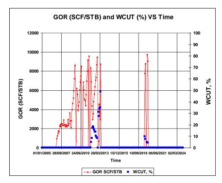
Figure 6. 18 GOR and Water cut for SP1 well of the Scenario 53
