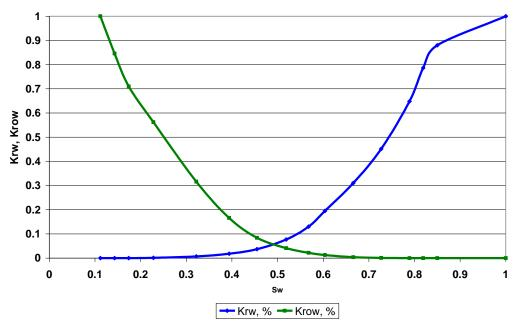
Figure 5. 11 Water saturation versus relative permeability to water and oil
