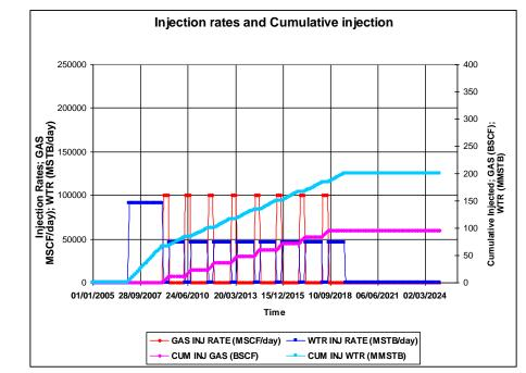
Figure 6.8 Injection Rates and Cumulative Injection of Scenario 40 of South Flank Region
