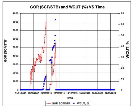
Figure 5. 25. GOR and Water cut for SP3 well of the Base Case
