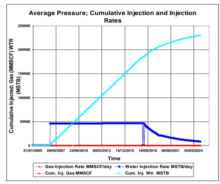
Figure 5. 31 Injection Rates and Cumulative Injection of WI2 well of Base Case
