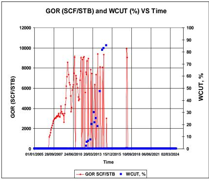
Figure 6. 21 GOR and Water cut for SP2 well of the Scenario 53
