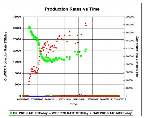
Figure 6. 37 Gas, Oil, Water Production rates for SP1 well of the Scenario 52
