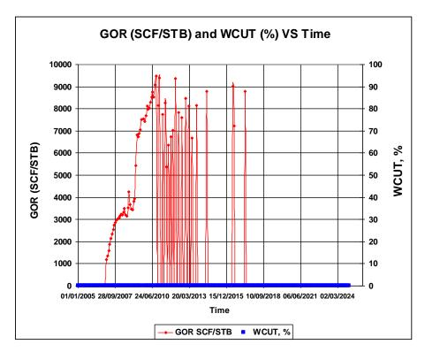
Figure 6. 41 GOR and Water cut for SP2 well of the Scenario 52
