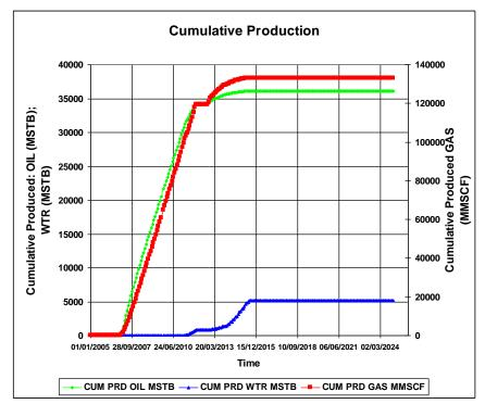
Figure 5. 23 Cumulative Produced Gas, Oil, and Water from SP2 well of the Base Case
