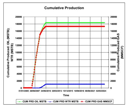
Figure 5. 29 Cumulative Produced Gas, Oil, and Water from SP4 well of the Base Case
