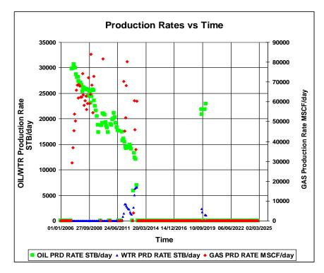
Figure 6. 17 Gas, Oil, Water Production rates for SP1 well of the Scenario 53
