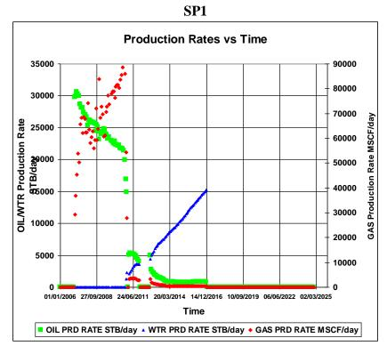
Figure 5. 18 Gas, Oil, Water Production rates for SP1 well of the Base Case
