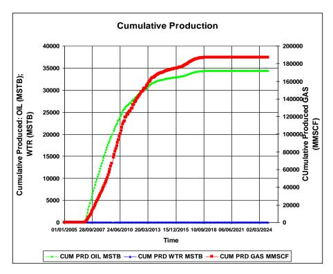
Figure 6. 42 Cumulative Produced Gas, Oil, and Water from SP2 well of the Scenario 52
