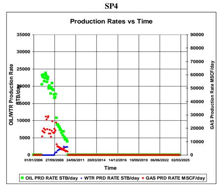
Figure 5. 27 Gas, Oil, Water Production rates for SP4 well of the Base Case
