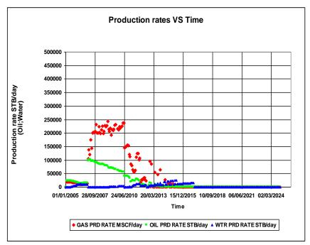
Figure 5. 15 Gas, oil, and water production rates for the Base Case of the South Flank region
