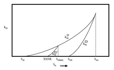
Figure 1D. 1 Nonwetting Phase Relative Permeability Curves for Hysteresis
