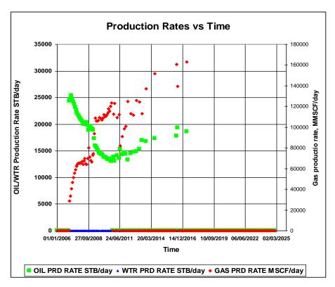
Figure 6. 40 Gas, Oil, Water Production rates for SP2 well of the Scenario 52
