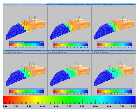
Figure 6. 31 Water saturation map showing down flow of water during injection for Scenario 52
