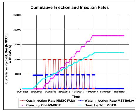
Figure 6. 29 Injection Rates and Cumulative Injection of WI1 well of Scenario 53
