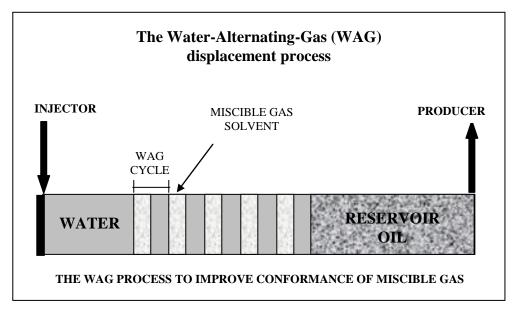
Figure 2.1 Schematic view of the process [4]
