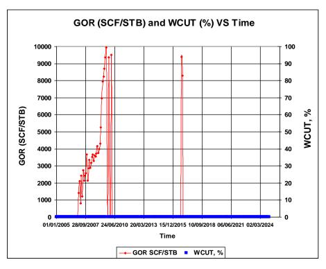
Figure 6. 44 GOR and Water cut for SP3 well of the Scenario 52
