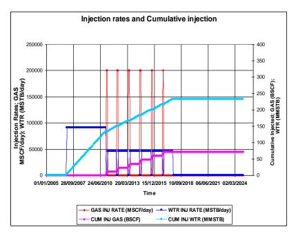
Figure 6.4 Injection Rates and Cumulative Injection of Scenario 39 of South Flank Region
