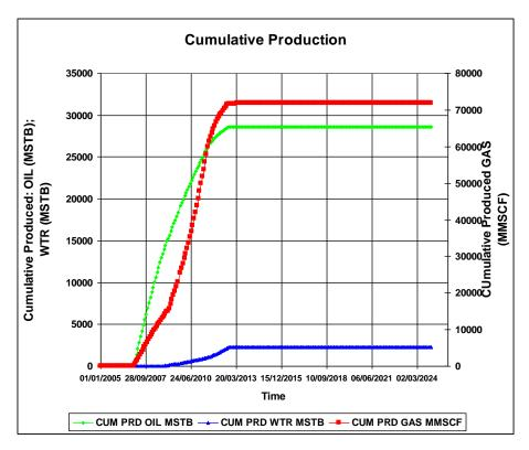
Figure 6. 48 Cumulative Produced Gas, Oil, and Water from SP4 well of the Scenario 52
