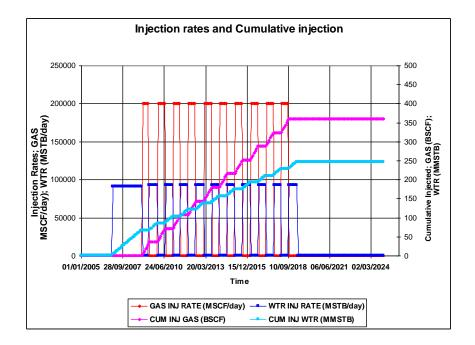
Figure 6. 14 Injection Rates and Cumulative Injection of Scenario 53 of South Flank Region
