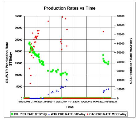
Figure 6. 23 Gas, Oil, Water Production rates for SP3 well of the Scenario 53
