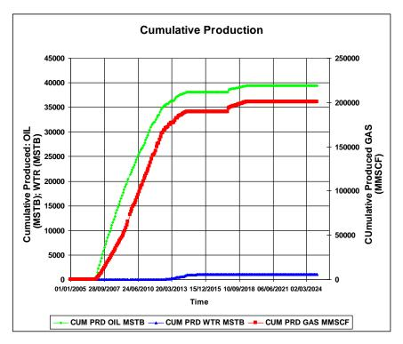
Figure 6. 22 Cumulative Produced Gas, Oil, and Water from SP2 well of the Scenario 53
