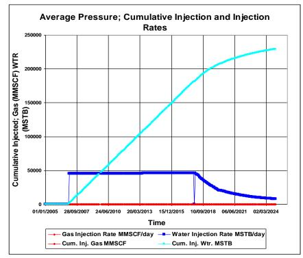
Figure 5. 30 Injection Rates and Cumulative Injection of WI1 well of Base Case
