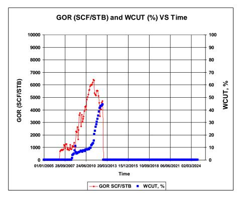
Figure 6. 47 Figure 37 GOR and Water cut for SP4 well of the Scenario 52
