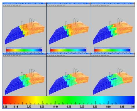
Figure 6. 49 Water saturation map showing down flow of water during injection for Scenario 59
