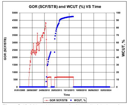
Figure 5. 19 GOR and Water cut for SP1 well of the Base Case
