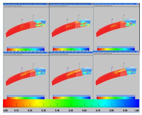
Figure 6. 50 Gas saturation map showing upper segregation of gas during injection for Scenario 59
