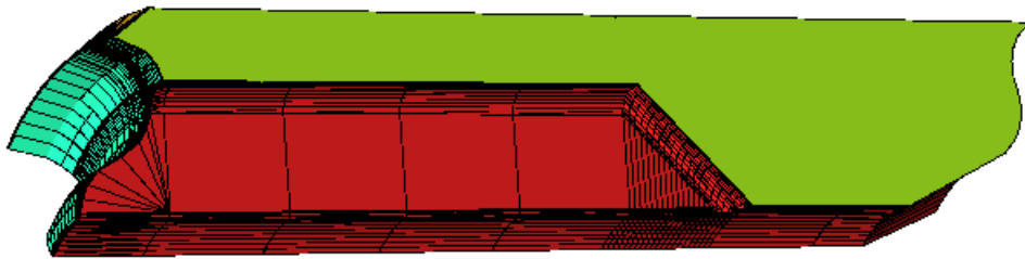
Figure 3.2: Finocyl grain partial surface mesh
