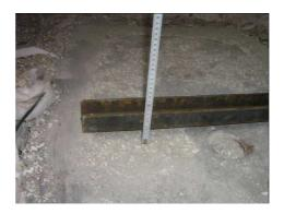
Figure 3.13 Spalling of Specimen (Test 1)
