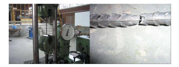
Figure 3.3 Tensile Strength Tests of Reference Segment Reinforcement Samples
