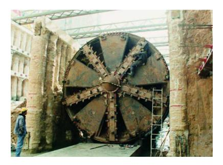
Figure 1.4 TBM Cutting Head [8]
