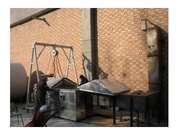
Figure 3.4 Fire Test Furnace
