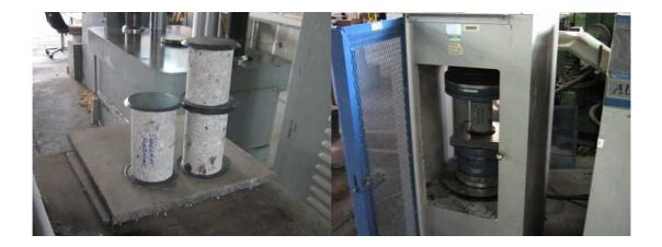
Figure 3.2 Compressive Strength Tests of Reference Segment Core Samples
