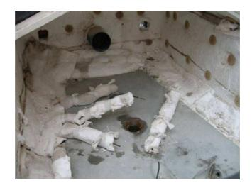
Figure 3.6 Placements of Thermocouples and Inside of Furnace
