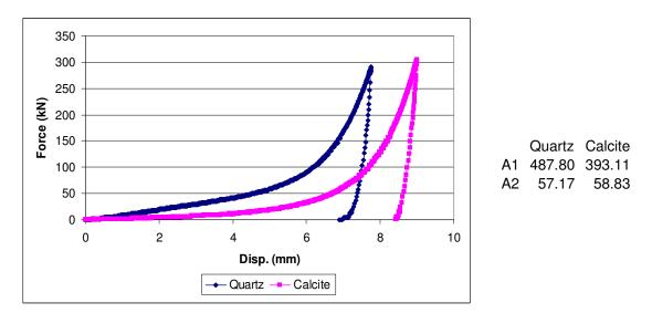
**Figure C. 13:** -1.18+0.85mm quartz and calcite samples comminuted in die-piston under 300kN force
