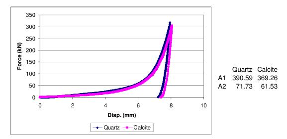
**Figure C. 1:** -3.35+2.36mm quartz and calcite samples comminuted in die-piston under 300kN force
