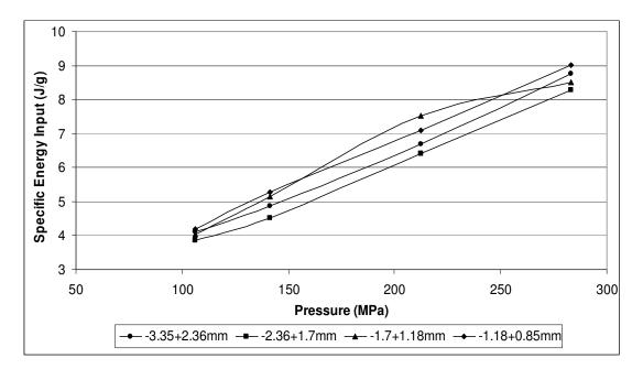
Figure 36: Specific Energy versus Pressure for different sizes of calcite sample
