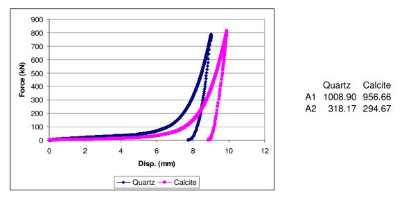
**Figure C. 8:** -2.36+1.7mm quartz and calcite samples comminuted in die-piston under 800kN force
