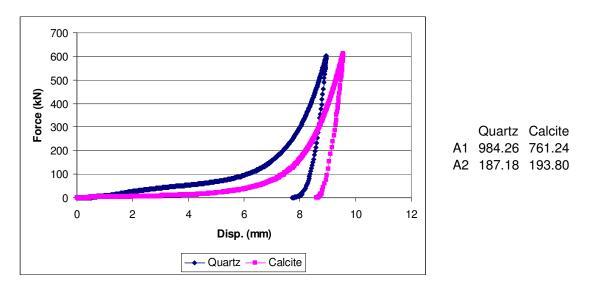
Figure C. 15: 1.18+0.85mm quartz and calcite samples comminuted in die-piston under 600kN force
