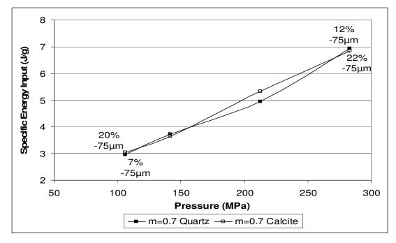
Figure 32: Specific energy comparison of m=0.7 quartz and calcite samples at specified pressures
