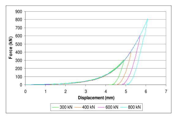
Figure 10: Force versus Displacement graph of m=0.5 calcite sample
