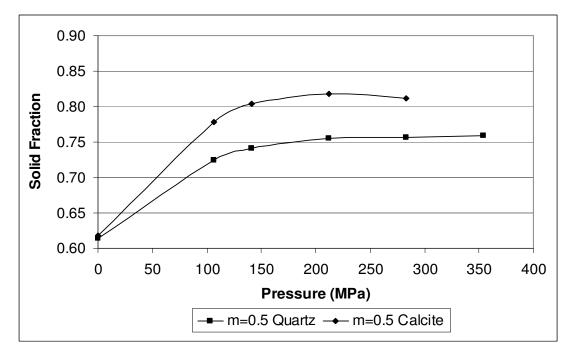
Figure 42: Solid fraction as a function of pressure applied in the particle bed comminution of quartz and calcite
