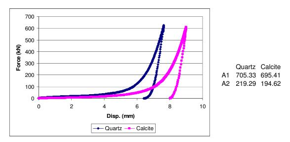
**Figure C. 3:** -3.35+2.36mm quartz and calcite samples comminuted in die-piston under 600kN force
