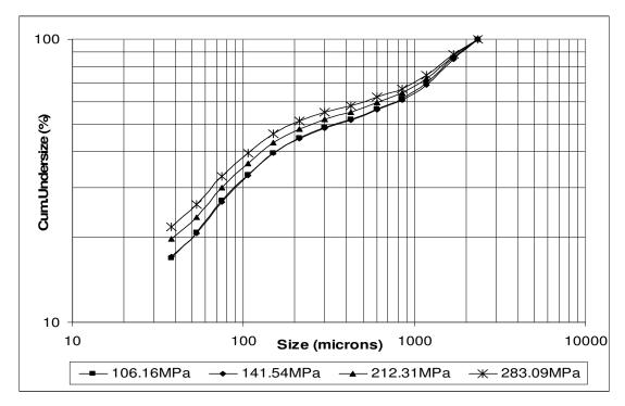
Figure D. 11: Product particle size distribution graph of -2.36+1.7mm calcite sample
