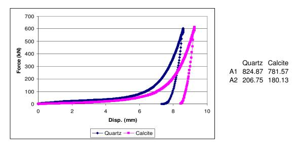
**Figure C. 11:** -1.7+1.18mm quartz and calcite samples comminuted in die-piston under 600kN force
