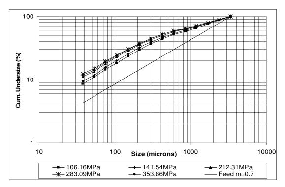
Figure D. 7: Product particle size distribution graph of m=0.7 quartz sample
