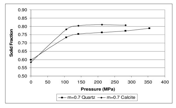
Figure 43: Solid fraction as a function of pressure applied in the particle bed comminution of quartz and calcite
