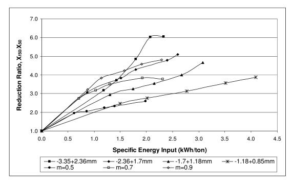
**Figure 49:** Reduction ratio as a function of specific energy input for different sizes of quartz samples comminuted in the piston-die-press
