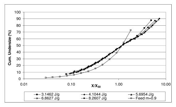
Figure 19: Self-similar size distributions of m=0.9 quartz sample comminuted in piston-die-press
