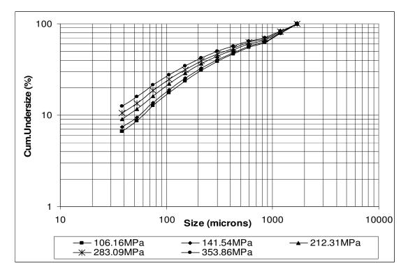
Figure D. 3: Product particle size distribution graph of -1.7+1.18mm quartz sample
