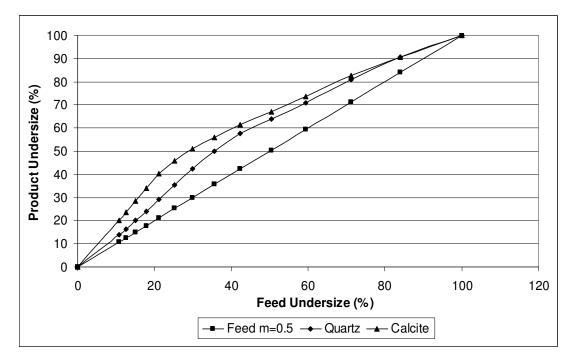
**Figure 71:** Comparison of size reduction curves of quartz and calcite at 300kN pressure in piston-die-press
