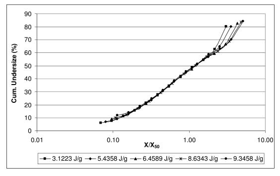
**Figure 14:** Self-similar size distributions of -2.36+1.7mm quartz sample comminuted in piston-die-press
