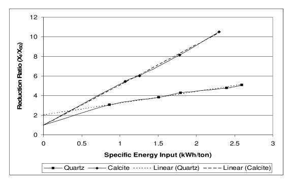
**Figure 52:** Reduction ratio as a function of specific energy input for -2.36+1.7mm quartz and calcite samples comminuted in the piston-die-press
