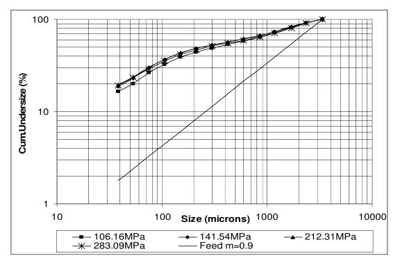
Figure D. 16: Product particle size distribution graph of m=0.9 calcite sample
