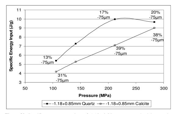
**Figure 30:** Specific energy comparison of -1.18 +0.85mm quartz and calcite samples at specified pressures
