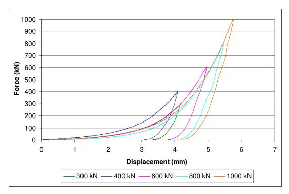
Figure 9: Force versus Displacement graph of m=0.5 quartz sample
