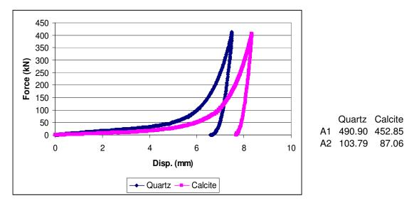
**Figure C. 2:** -3.35+2.36mm quartz and calcite samples comminuted in die-piston under 400kN force
