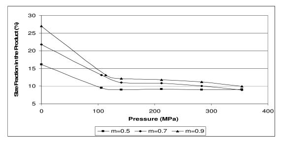
**Figure 58:** Size fraction of -3.35+2.36mm quartz sample in m=0.5, m=0.7 and m=0.9 distribution moduli at specified pressures
