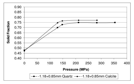
**Figure 41:** Solid fraction as a function of pressure applied in the particle bed comminution of quartz and calcite
