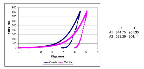
**Figure C. 20:** m=0.5 quartz and calcite samples comminuted in die-piston under 800kN force
