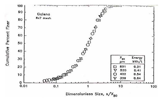
**Figure 5:** Self-similar size distribution of galena comminuted in the single-particle mode (Fuerstenau and Kapur, 1994)
