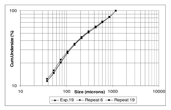
**Figure F. 4:** Repeatability of particle size distribution of -1.18+0.85mm quartz sample at 80 ton load in piston-die-press set-up
