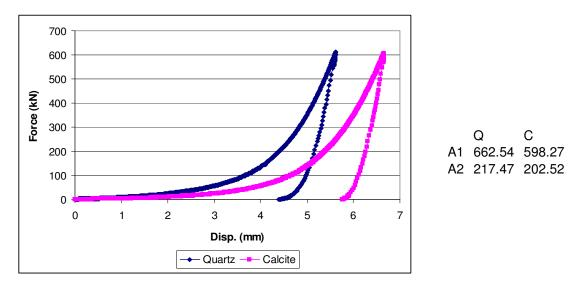
**Figure C. 23:** m=0.7 quartz and calcite samples comminuted in die-piston under 600kN force
