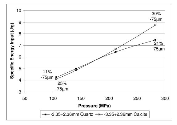
**Figure 27:** Specific energy comparison of -3.35 +2.36mm quartz and calcite samples at specified pressures
