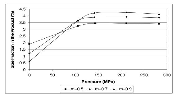
**Figure 67:** Size fraction of  $-53+38\mu$ m calcite sample in m=0.5, m=0.7 and m=0.9 distribution moduli at specified pressures
