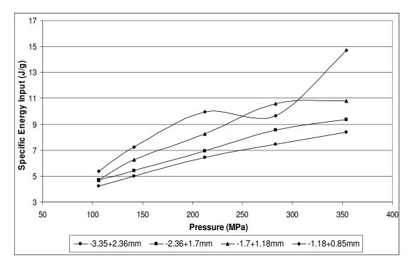
Figure 34: Specific Energy versus Pressure for different sizes of quartz sample
