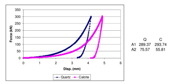
**Figure C. 17:** m=0.5 quartz and calcite samples comminuted in die-piston under 300kN force
