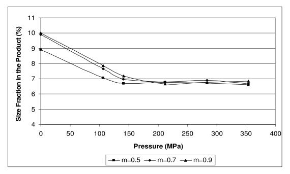
**Figure 60:** Size fraction of -1.18+0.85mm quartz sample in m=0.5, m=0.7 and m=0.9 distribution moduli at specified pressures
