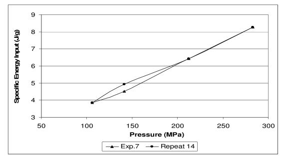
**Figure F. 9:** Repeatability of specific energy input values of -2.36+1.7mm calcite sample at 40 ton load in piston-die-press set-up
