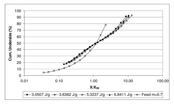
**Figure 25:** Self-similar size distributions of m=0.7 calcite sample comminuted in piston-die-press
