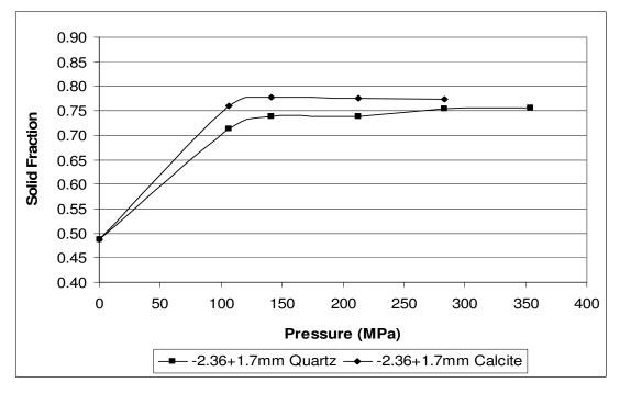
Figure 39: Solid fraction as a function of pressure applied in the particle bed comminution of quartz and calcite
