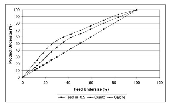
**Figure 72:** Comparison of size reduction curves of quartz and calcite at 800kN pressure in piston-die-press
