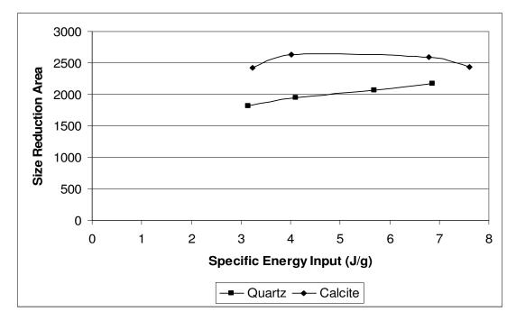
**Figure 77:** Comparison of size reduction areas for quartz and calcite samples having distribution moduli of 0.7 to evaluate the energy utilization
