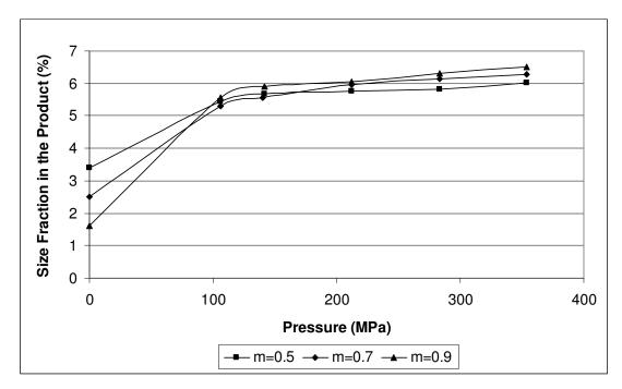
**Figure 64:** Size fraction of -150+106µm quartz sample in m=0.5, m=0.7 and m=0.9 distribution moduli at specified pressures
