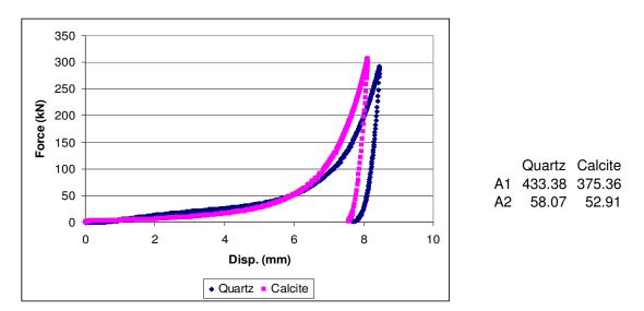
**Figure C. 9:** -1.7+1.18mm quartz and calcite samples comminuted in die-piston under 300kN force
