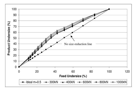
Figure 68: Size reduction curves for quartz sample of m=0.5
