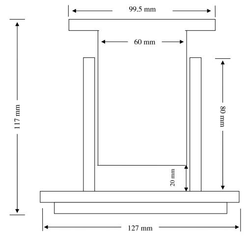
Figure 8: Illustration of the die-piston
