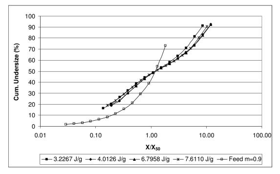
Figure 26: Self-similar size distributions of m=0.9 calcite sample comminuted in piston-die-press
