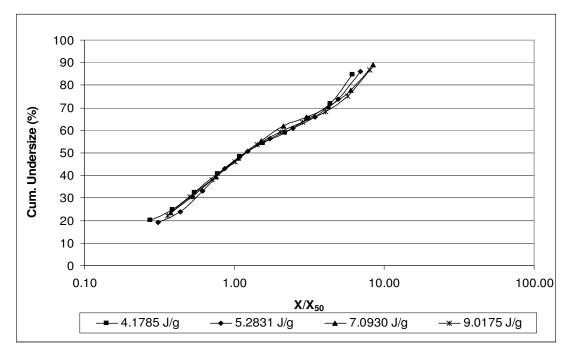
**Figure 23:** Self-similar size distributions of -1.18+0.85mm calcite sample comminuted in piston-die-press
