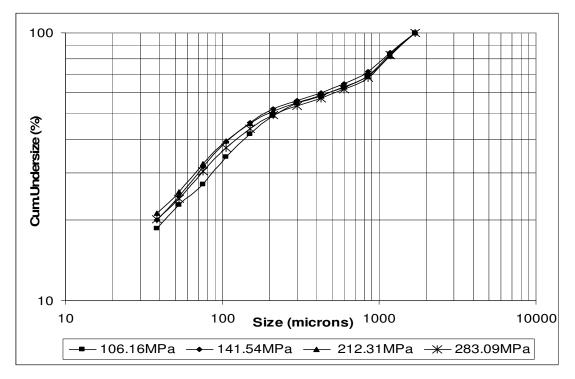
Figure D. 12: Product particle size distribution graph of -1.7+1.18mm calcite sample
