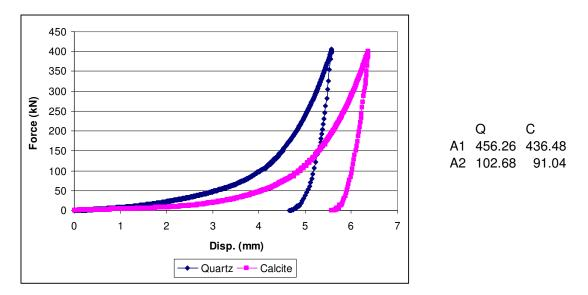
**Figure C. 22:** m=0.7 quartz and calcite samples comminuted in die-piston under 400kN force
