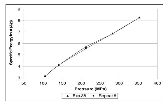
**Figure F. 5:** Repeatability of specific energy input values of m=0.9 quartz sample at 60 ton load in piston-die-press set-up
