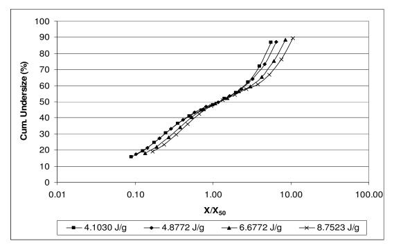
**Figure 20:** Self-similar size distributions of -3.35+2.36mm calcite sample comminuted in piston-die-press
