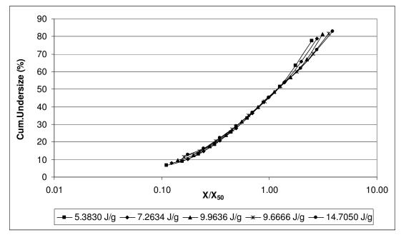
**Figure 16:** Self-similar size distributions of -1.18+0.85mm quartz sample comminuted in piston-die-press
