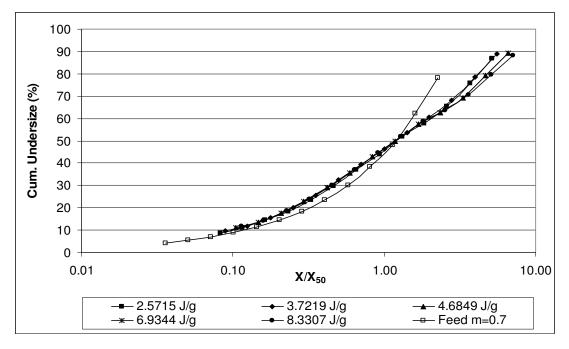
Figure 18: Self-similar size distributions of m=0.7 quartz sample comminuted in piston-die-press
