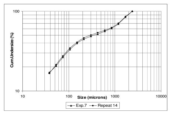
**Figure F. 10:** Repeatability of particle size distribution of -2.36+1.7mm calcite sample at 40 ton load in piston-die-press set-up
