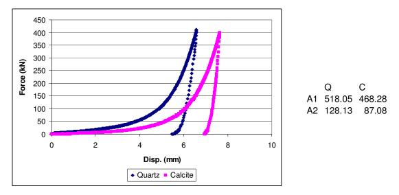
**Figure C. 26:** m=0.9 quartz and calcite samples comminuted in die-piston under 400kN force
