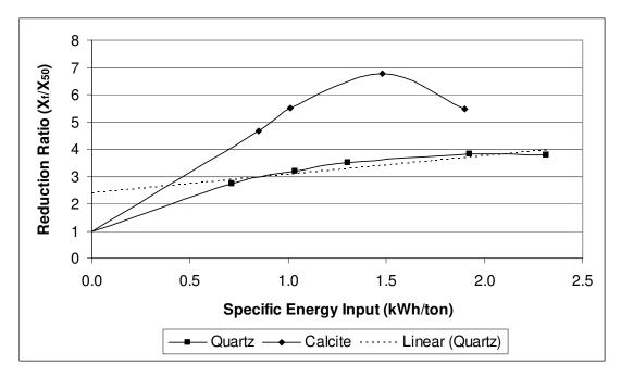
**Figure 56:** Reduction ratio as a function of specific energy input for m=0.7 quartz and calcite samples comminuted in the piston-die-press
