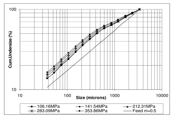
Figure D. 6: Product particle size distribution graph of m=0.5 quartz sample
