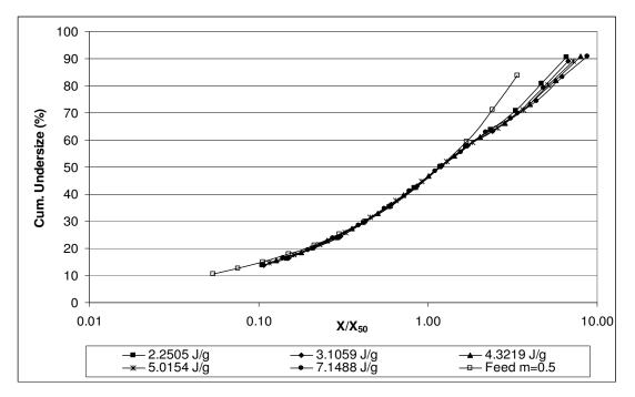
Figure 17: Self-similar size distributions of m=0.5 quartz sample comminuted in piston-die-press
