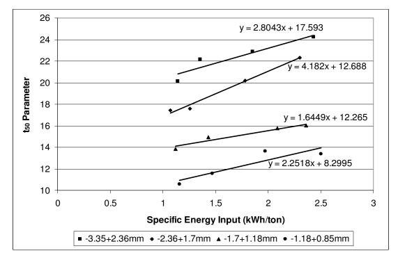
Figure 80:  $t_{50}$  parameter vs. specific energy input for different sizes of calcite samples
