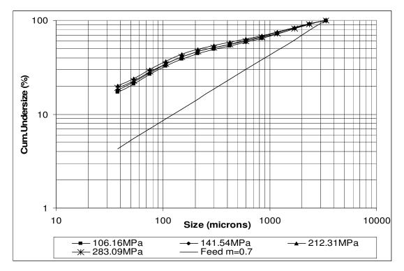
Figure D. 15: Product particle size distribution graph of m=0.7 calcite sample
