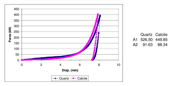
**Figure C. 6:** -2.36+1.7mm quartz and calcite samples comminuted in die-piston under 400kN force
