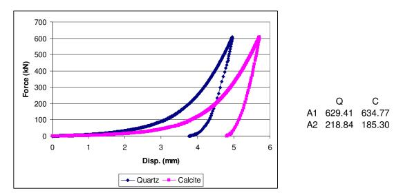
Figure C. 19: m=0.5 quartz and calcite samples comminuted in die-piston under 600kN force
