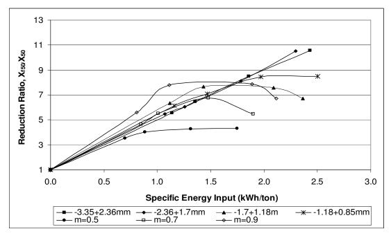
**Figure 50:** Reduction ratio as a function of specific energy input for different sizes of calcite samples comminuted in the piston-die-press
