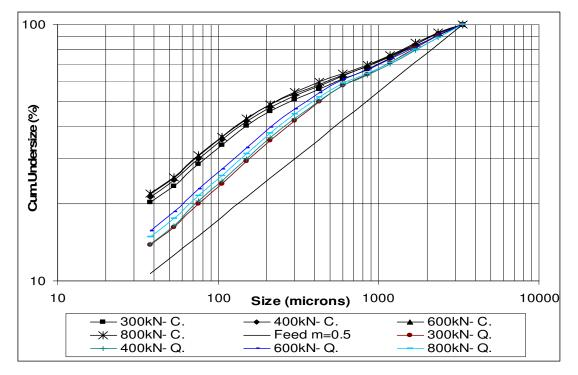
**Figure D. 18:** Comparison of product particle size distribution graphs of calcite and quartz samples for m=0.5 distribution modulus
