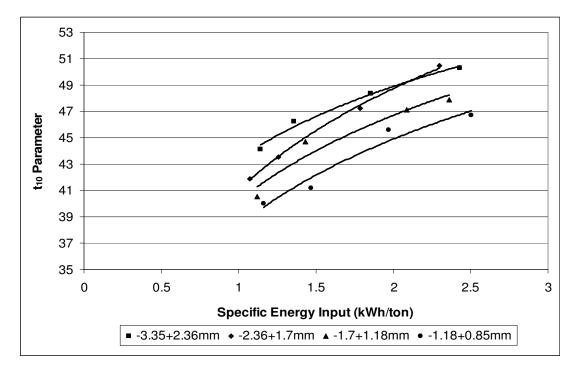
Figure 82:  $t_{10}$  parameter vs. specific energy input for different sizes of calcite samples
