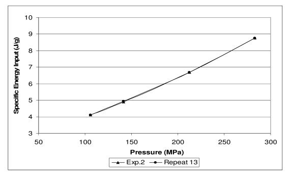
**Figure F. 7:** Repeatability of specific energy input values of -3.35+2.36mm calcite sample at 40 ton load in piston-die-press set-up
