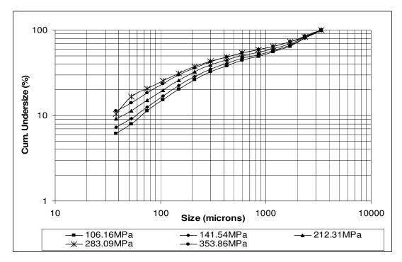
Figure 11: Product particle size distribution graph of -3.35+2.36mm quartz sample
