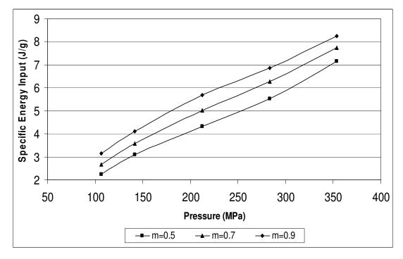
**Figure 35:** Specific Energy versus Pressure for m=0.5 m=0.7 and m=0.9 values of quartz sample
