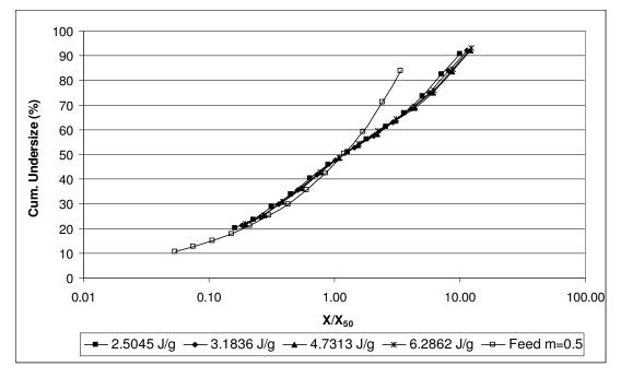
Figure 24: Self-similar size distributions of m=0.5 calcite sample comminuted in piston-die-press
