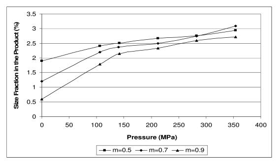
**Figure 66:** Size fraction of  $-53+38\mu$ m quartz sample in m=0.5, m=0.7 and m=0.9 distribution moduli at specified pressures
