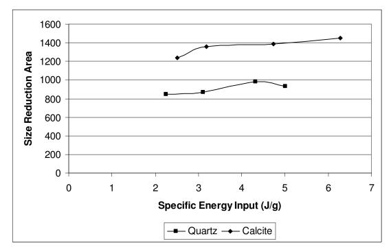
**Figure 75:** Comparison of size reduction areas for quartz and calcite samples having distribution moduli of 0.5 to evaluate the energy utilization
