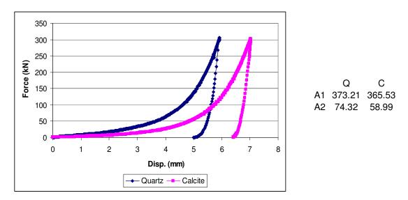
**Figure C. 25:** m=0.9 quartz and calcite samples comminuted in die-piston under 300kN force
