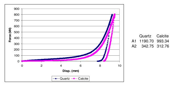
**Figure C. 12:** -1.7+1.18mm quartz and calcite samples comminuted in die-piston under 800kN force
