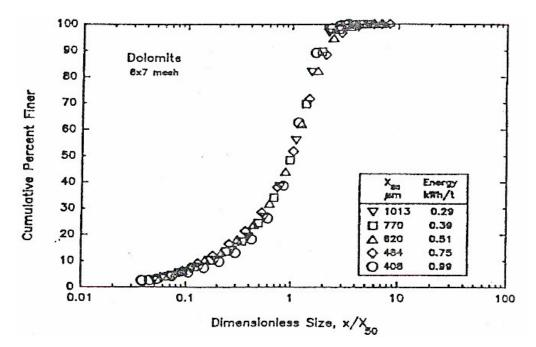
**Figure 6:** Self-similar size distribution of dolomite comminuted in the single-particle mode (Fuerstenau and Kapur, 1994)
