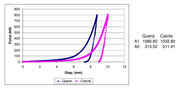
**Figure C. 16:** 1.18+0.85mm quartz and calcite samples comminuted in die-piston under 800kN force
