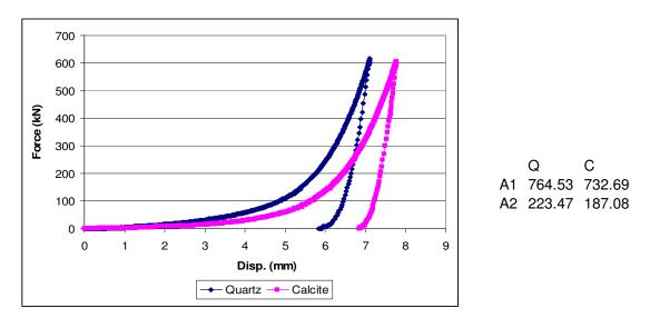
Figure C. 27: m=0.9 quartz and calcite samples comminuted in die-piston under 600kN force
