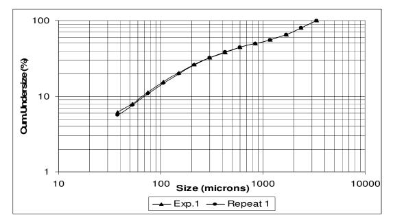
**Figure F. 2:** Repeatability of particle size distribution of -3.35+2.36mm quartz sample at 30 ton load in piston-die-press set-up
