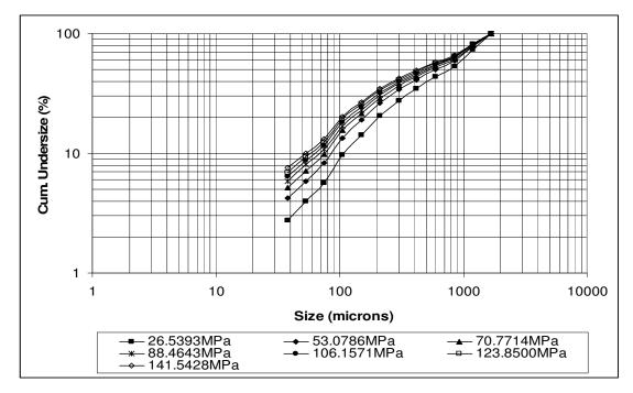
**Figure D. 4:** Product particle size distribution graph of -1.7+1.18mm quartz sample comminuted in MTS Compression Testing Machine
