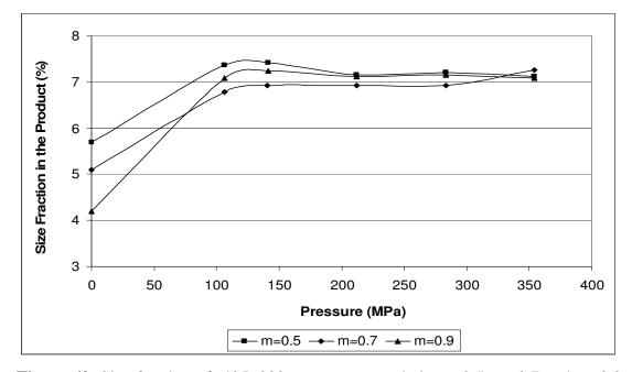
**Figure 62:** Size fraction of -425+300µm quartz sample in m=0.5, m=0.7 and m=0.9 distribution moduli at specified pressures
