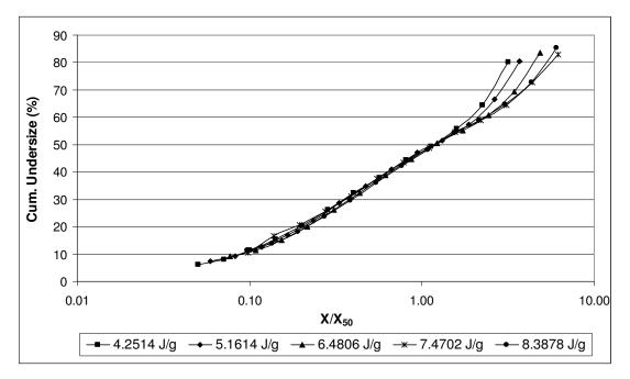
**Figure 13:** Self-similar size distributions of -3.35+2.36mm quartz sample comminuted in piston-die-press
