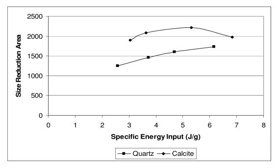
**Figure 76:** Comparison of size reduction areas for quartz and calcite samples having distribution moduli of 0.7 to evaluate the energy utilization
