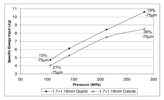
**Figure 29:** Specific energy comparison of -1.7 +1.18mm quartz and calcite samples at specified pressures
