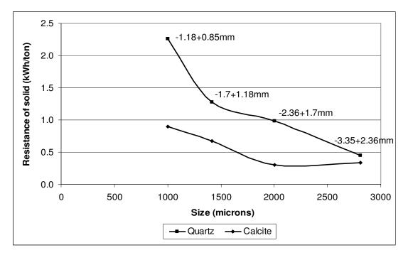
**Figure 78:** Resistances of narrow-range size fractions of quartz and calcite to size reduction in die-piston press.
