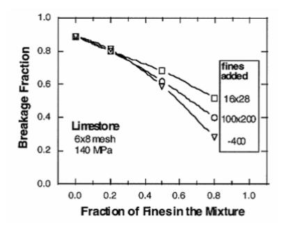
**Figure 2:** Breakage probability for 6x8 mesh limestone comminuted in the presence of fines (Gutsche and Fuerstenau, 1999)
