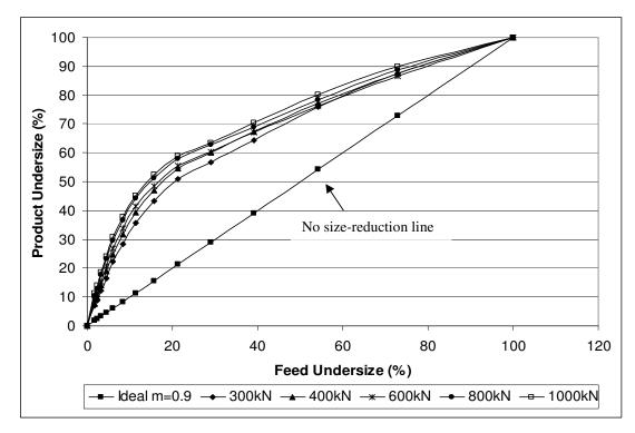
Figure 70: Size reduction curves for quartz sample of m=0.9
