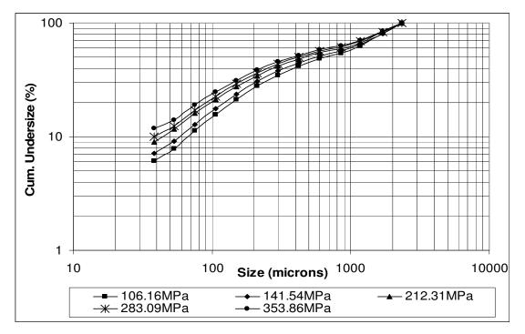
Figure D. 2: Product particle size distribution graph of -2.36+1.7mm quartz sample
