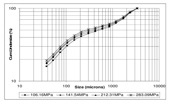
Figure 12: Product particle size distribution graph of -3.35+2.36mm calcite sample
