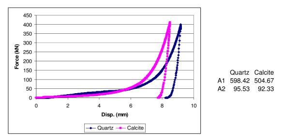
**Figure C. 10:** -1.7+1.18mm quartz and calcite samples comminuted in die-piston under 400kN force
