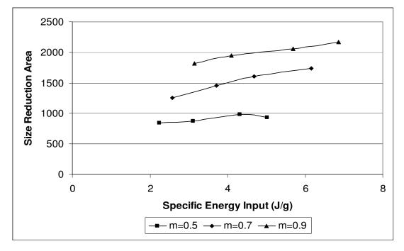
**Figure 73:** Size reduction areas of quartz as a function of specific energy inputs for different distribution moduli compared to evaluate the energy utilization of samples
