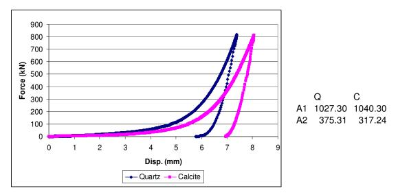
**Figure C. 28:** m=0.9 quartz and calcite samples comminuted in die-piston under 800kN force
