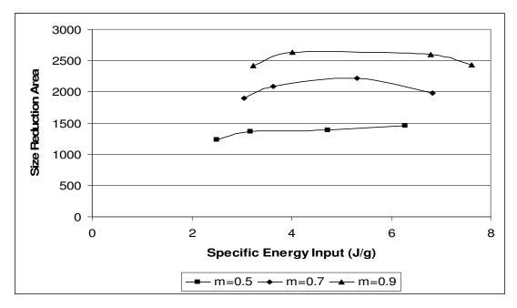
**Figure 74:** Size reduction areas of calcite as a function of specific energy inputs for different distribution moduli compared to evaluate the energy utilization of samples
