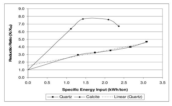
**Figure 53:** Reduction ratio as a function of specific energy input for -1.7+1.18mm quartz and calcite samples comminuted in the piston-die-press
