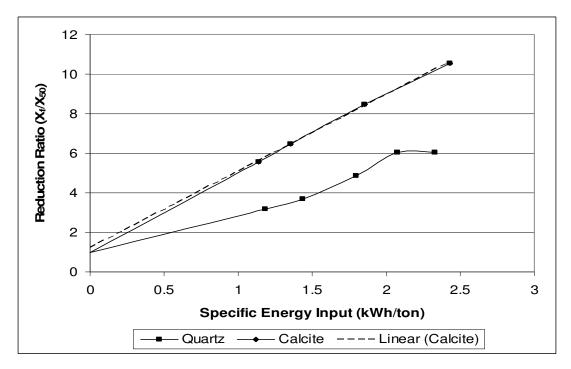
**Figure 51:** Reduction ratio as a function of specific energy input for -3.35+2.36mm quartz and calcite samples comminuted in the piston-die-press
