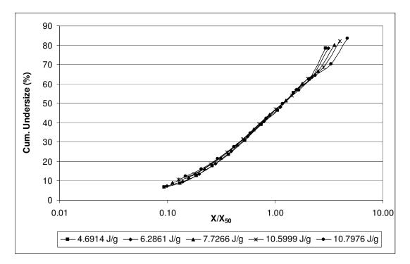
**Figure 15:** Self-similar size distributions of -1.7+1.18mm quartz sample comminuted in piston-die-press
