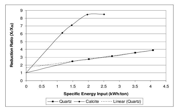
**Figure 54:** Reduction ratio as a function of specific energy input for -1.18+0.85mm quartz and calcite samples comminuted in the piston-die-press
