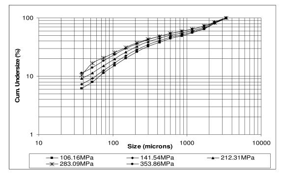
Figure D. 1: Product particle size distribution graph of -3.35+2.36mm quartz sample
