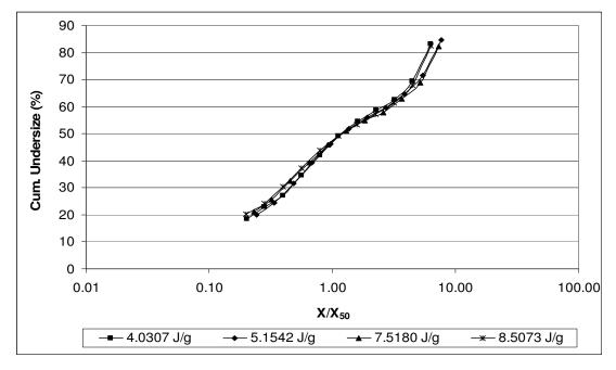
**Figure 22:** Self-similar size distributions of -1.7+1.18mm calcite sample comminuted in piston-die-press
