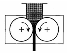
Figure 1: High pressure roll mill operating principle
