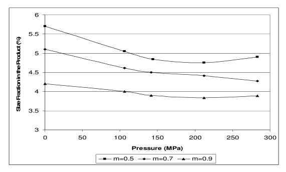
**Figure 63:** Size fraction of -425+300µm calcite sample in m=0.5, m=0.7 and m=0.9 distribution moduli at specified pressures
