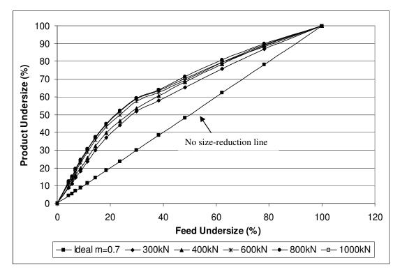
Figure 69: Size reduction curves for quartz sample of m=0.7
