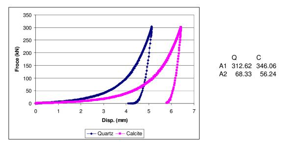
**Figure C. 21:** m=0.7 quartz and calcite samples comminuted in die-piston under 300kN force
