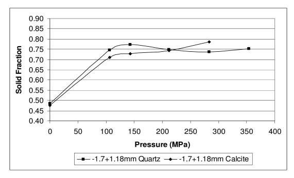
Figure 40: Solid fraction as a function of pressure applied in the particle bed comminution of quartz and calcite
