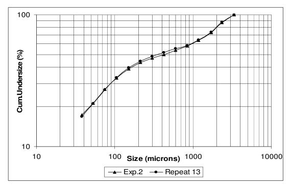
**Figure F. 8:** Repeatability of particle size distribution of -3.35+2.36mm calcite sample at 40 ton load in piston-die-press set-up
