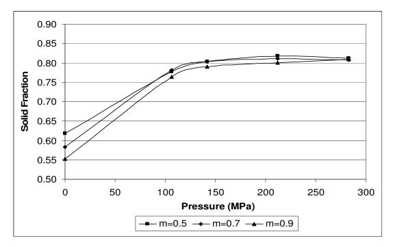
**Figure 48:** Solid fraction as a function of pressure applied in the particle bed comminution of calcite at different GGS distribution moduli
