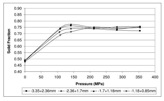
**Figure 45:** Solid fraction as a function of pressure applied in the particle bed comminution of quartz at different size ranges
