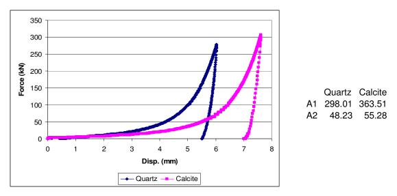
**Figure C. 5:** -2.36+1.7mm quartz and calcite samples comminuted in die-piston under 300kN force
