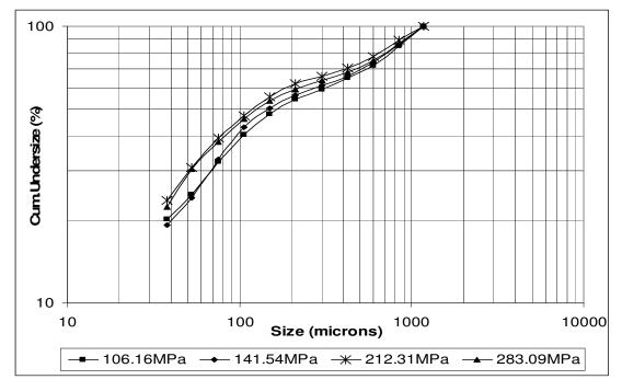
Figure D. 13: Product particle size distribution graph of -1.18+0.85mm calcite sample
