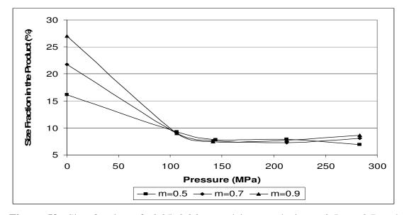
**Figure 59:** Size fraction of -3.35+2.36mm calcite sample in m=0.5, m=0.7 and m=0.9 distribution moduli at specified pressures
