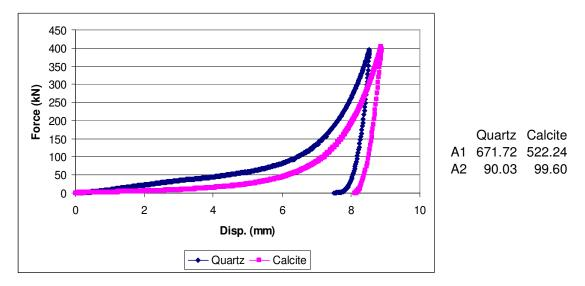
**Figure C. 14:** -1.18+0.85mm quartz and calcite samples comminuted in die-piston under 400kN force
