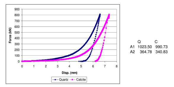
**Figure C. 24:** m=0.7 quartz and calcite samples comminuted in die-piston under 800kN force
