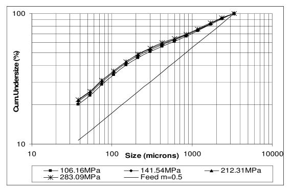
Figure D. 14: Product particle size distribution graph of m=0.5 calcite sample
