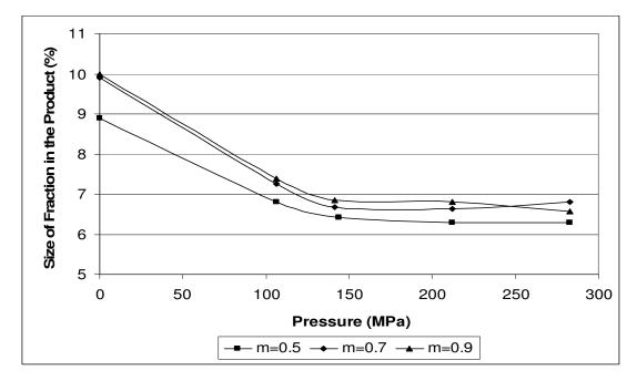
**Figure 61:** Size fraction of -1.18+0.85mm calcite sample in m=0.5, m=0.7 and m=0.9 distribution moduli at specified pressures
