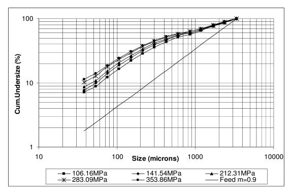
Figure D. 8: Product particle size distribution graph of m=0.9 quartz sample
