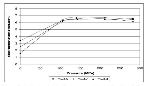
**Figure 65:** Size fraction of -150+106µm calcite sample in m=0.5, m=0.7 and m=0.9 distribution moduli at specified pressures
