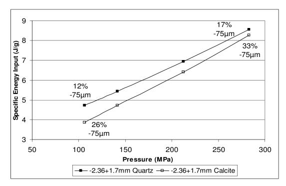
**Figure 28:** Specific energy comparison of -2.36 +1.7mm quartz and calcite samples at specified pressures
