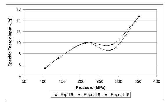
**Figure F. 3:** Repeatability of specific energy input values of -1.18+0.85mm quartz sample at 80 ton load in piston-die-press set-up
