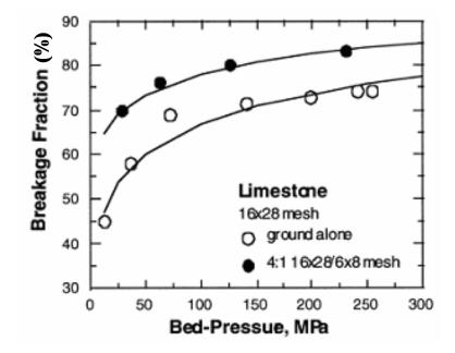
**Figure 3:** Breakage probability for 16x28 mesh limestone comminuted in the presence of 6x8 mesh coarse particles (Gutsche and Fuerstenau, 1999)
