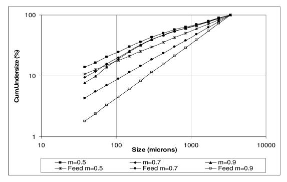
Figure D. 9: Comparison of the areas between ideal moduli lines at 0 pressure and the curves of those moduli, comminuted under 141.54 MPa pressure for quartz samples. 106
