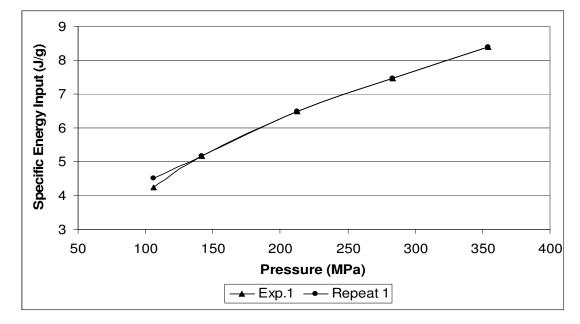
**Figure F. 1:** Repeatability of specific energy input values of -3.35+2.36mm quartz sample at 30 ton load in piston-die-press set-up
