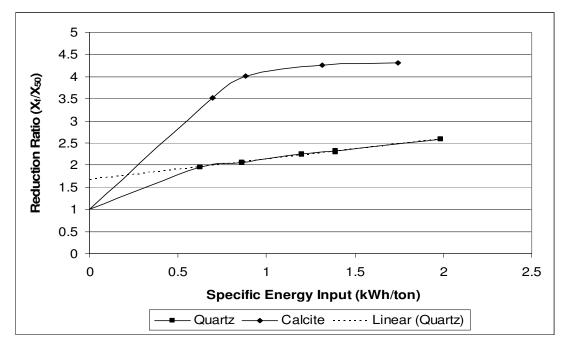
**Figure 55:** Reduction ratio as a function of specific energy input for m=0.5 quartz and calcite samples comminuted in the piston-die-press
