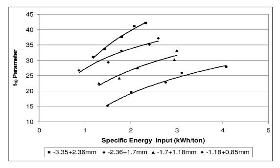
Figure 81:  $t_{10}$  parameter vs. specific energy input for different sizes of quartz samples
