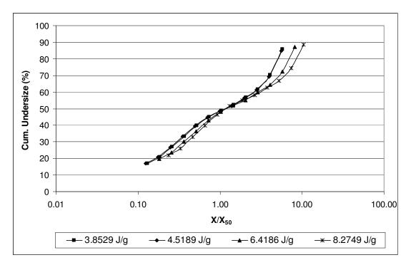
**Figure 21:** Self-similar size distributions of -2.36+1.7mm calcite sample comminuted in piston-die-press
