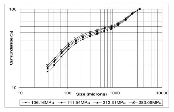
Figure D. 10: Product particle size distribution graph of -3.35+2.36mm calcite sample
