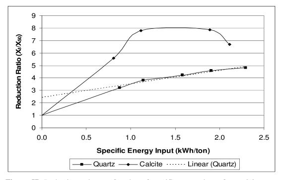
**Figure 57:** Reduction ratio as a function of specific energy input for m=0.9 quartz and calcite samples comminuted in the piston-die-press
