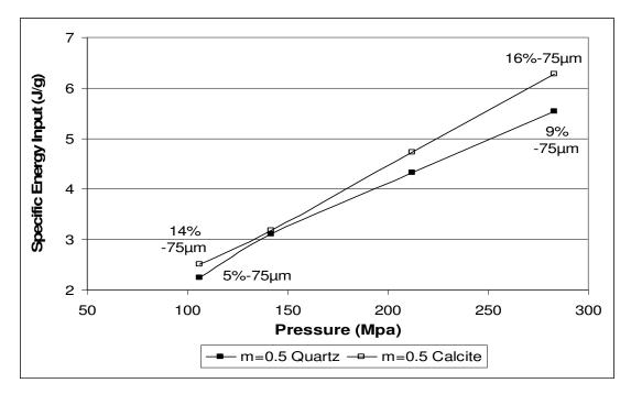
Figure 31: Specific energy comparison of m=0.5 quartz and calcite samples at specified pressures
