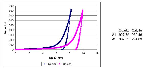
Figure C. 4: -3.35+2.36mm quartz and calcite samples comminuted in die-piston under 800kN force
