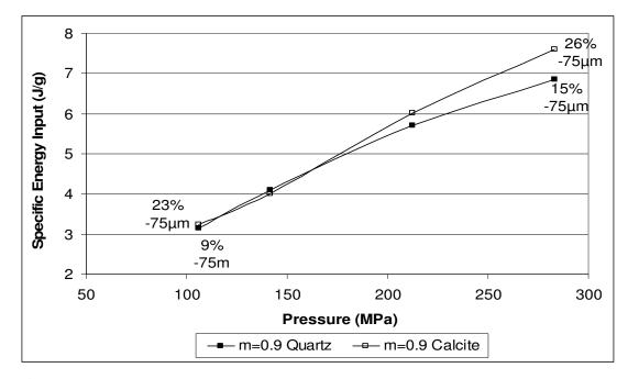
Figure 33: Specific energy comparison of m=0.9 quartz and calcite samples at specified pressures
