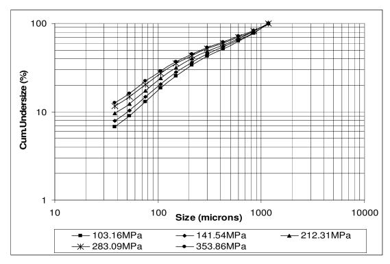
Figure D. 5: Product particle size distribution graph of -1.18+0.85mm quartz sample
