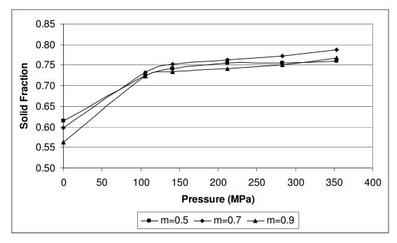
Figure 47: Solid fraction as a function of pressure applied in the particle bed comminution of quartz at different GGS distribution moduli
