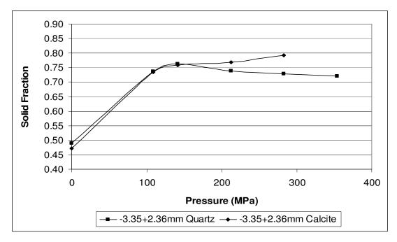
**Figure 38:** Solid fraction as a function of pressure applied in the particle bed comminution of quartz and calcite
