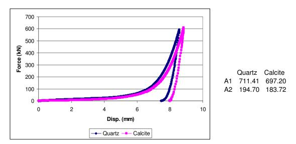
**Figure C. 7:** -2.36+1.7mm quartz and calcite samples comminuted in die-piston under 600kN force
