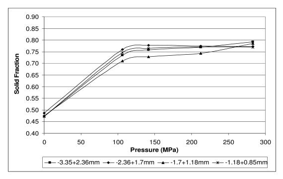
**Figure 46:** Solid fraction as a function of pressure applied in the particle bed comminution of calcite at different size ranges
