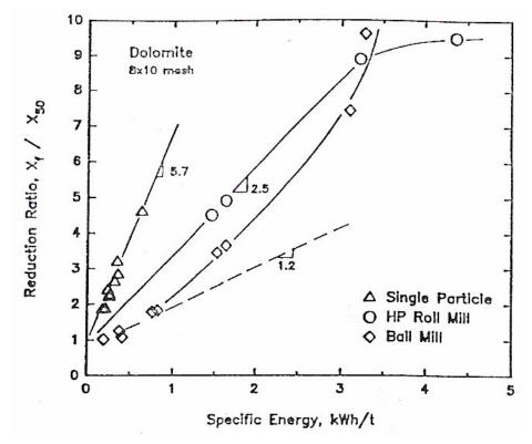
**Figure 7:** Reduction ratio as a function of specific grinding energy when 8x10 mesh dolomite is comminuted dry in the single particle mode, a high pressure roll mill and in a ball mill (Fuerstenau and Kapur, 1994)
