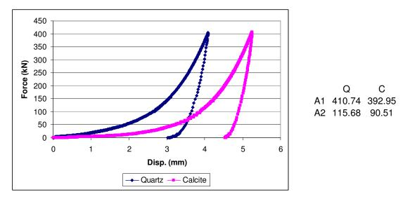
**Figure C. 18:** m=0.5 quartz and calcite samples comminuted in die-piston under 400kN force
