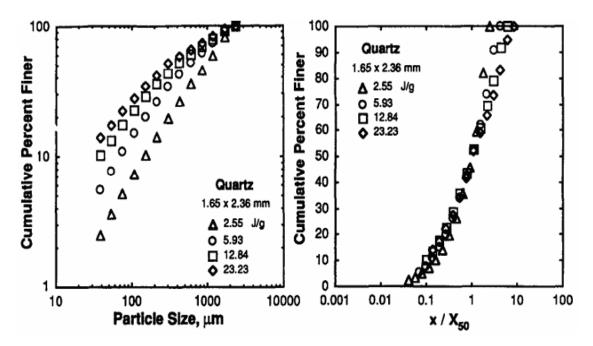
**Figure 4:** Self-similar size distribution of quartz comminuted in piston-die-press (Fuerstenau et. al., 1996)
