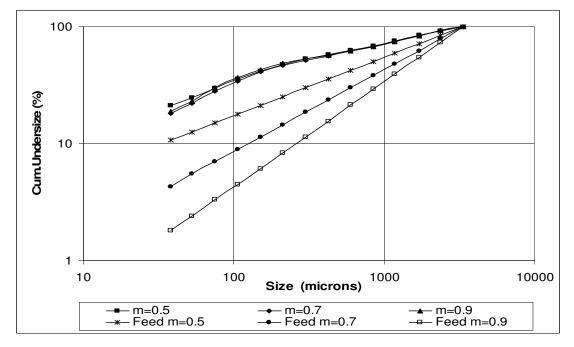
**Figure D. 17:** Comparison of the areas between ideal moduli lines at 0 pressure and the curves of those moduli, comminuted under 141.54 MPa pressure for calcite samples.
