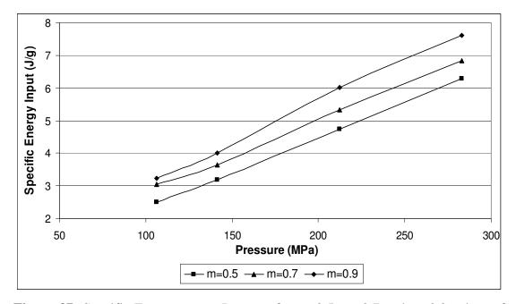
**Figure 37:** Specific Energy versus Pressure for m=0.5; m=0.7 and m=0.9 values of calcite sample
