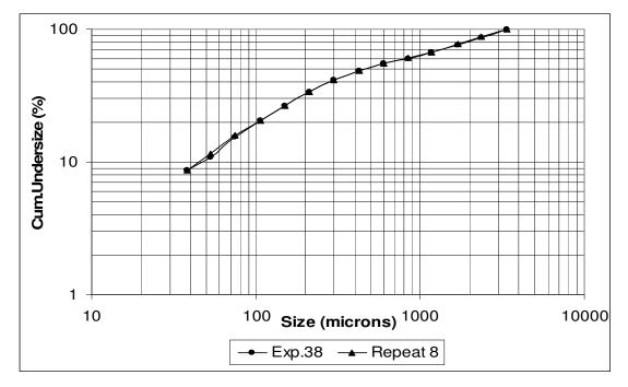
**Figure F. 6:** Repeatability of particle size distribution of m=0.9 quartz sample at 60 ton load in piston-die-press set-up
