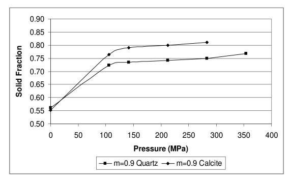
**Figure 44:** Solid fraction as a function of pressure applied in the particle bed comminution of quartz and calcite
