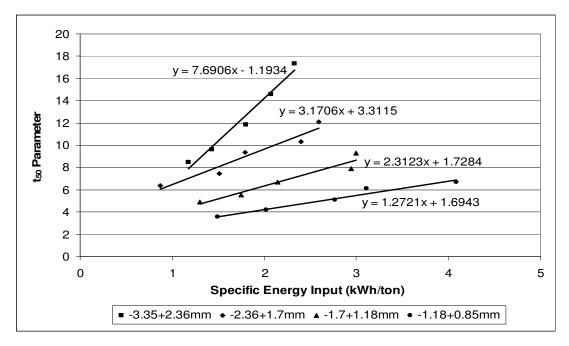
Figure 79: t<sub>50</sub> parameter vs. specific energy input for different sizes of quartz samples
