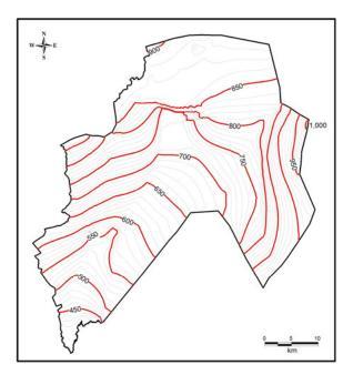
Figure 5.5 Calculated groundwater levels
