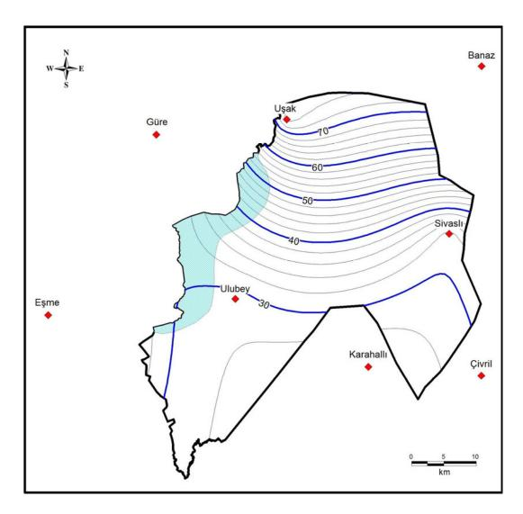
Figure 5.1 Areal distribution of recharge within the model domain (mm/year) and meteorological stations for which recharge is calculated by Thornthwaite method
