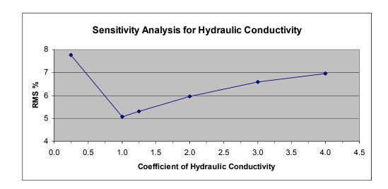
Figure 5.10 Results of sensitivity analysis for hydraulic conductivity
