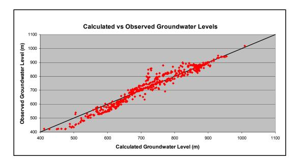
Figure 5.6 The graphical relation between calculated and observed groundwater levels
