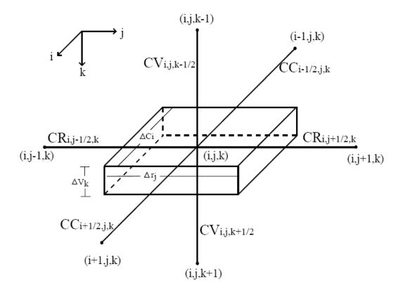
Figure 4.1 Definition of conductance terms between model cells
