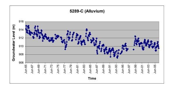
Figure 3.24 Temporal variation of groundwater in monitoring well 5289-C representing alluvium
