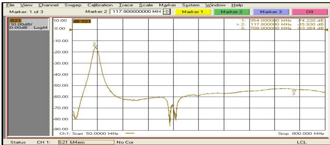
b) the response of filter at 118 MHz (S31)
