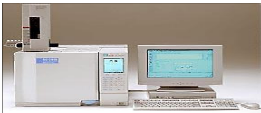
Figure 1.9 Shimadzu gas chromatograph (GC-2010 Series A) with flame ionization detector used during the study
