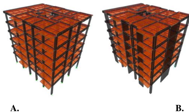
Figure 4.5 A. (Original Structural System of the Damaged Building Model F) B. (Re-designed Structural System Model G)
