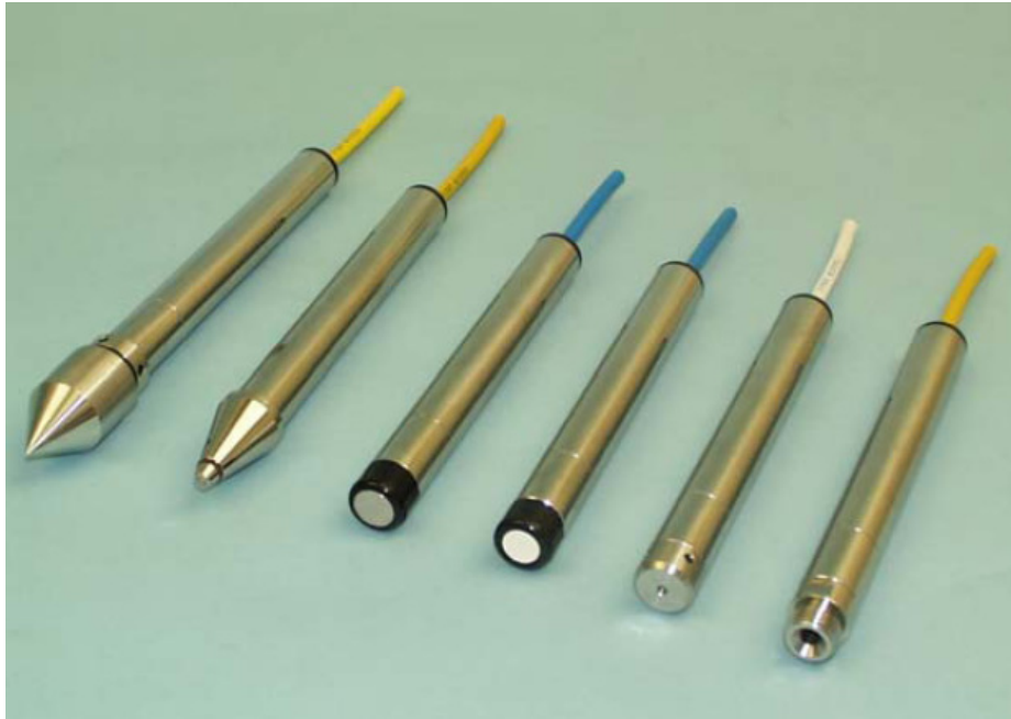
Figure 3.3 Vibrating wire piezometer (SISGEO, 2004-a)
