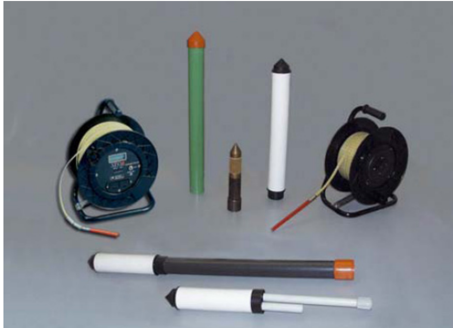
Figure 3.1 Standpipe piezometers and accessories (SISGEO,2004-a)
