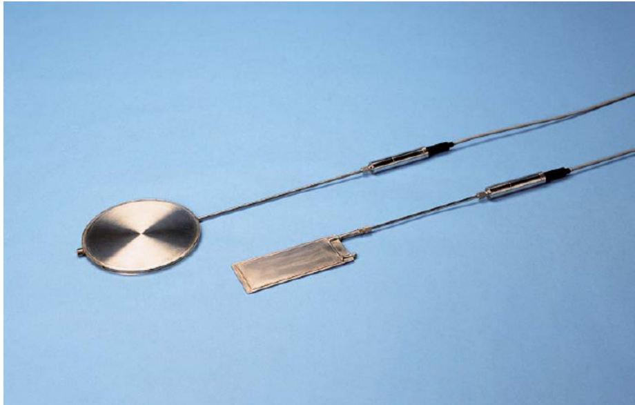
Figure 3.13 Total pressure (stress) cells (SISGEO, 2003-b)
