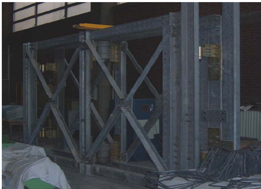
Figure 4.2 - Detailed View of the Steel Closed Frame
