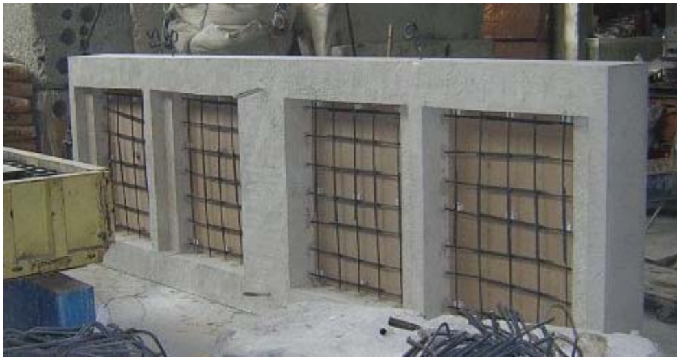
Figure 3.9 - Frame after Anchorage of Reinforcement
