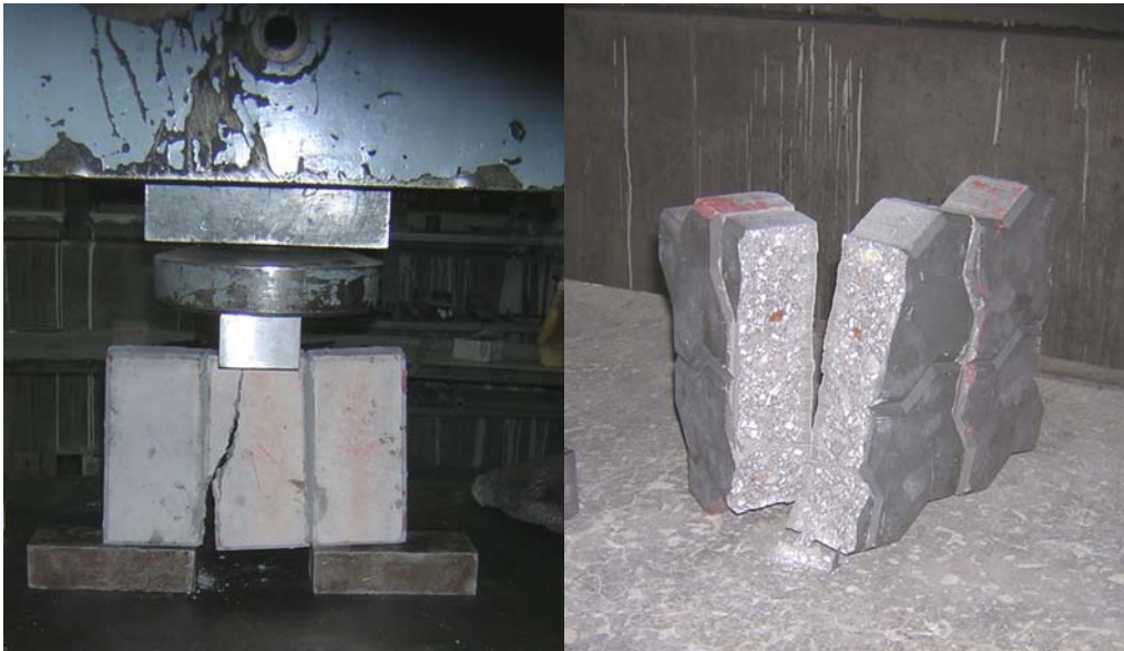
Figure 1.3 - Failure of Concrete Blocks Joined by Concrete 1406 Mortar
