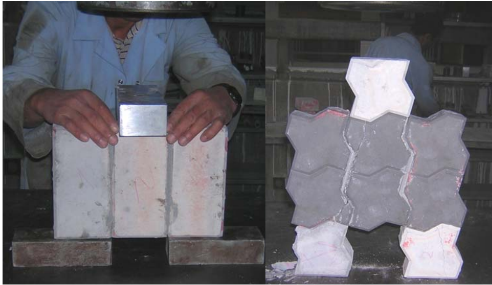
Figure 1.2 - Experimental Setup for the Shear Strength of Concrete Blocks Joined by Concrete 1406 Mortar
