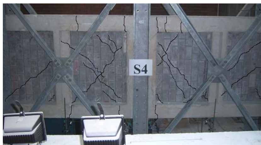
Figure 5.36 - Final View of the Specimen S4
