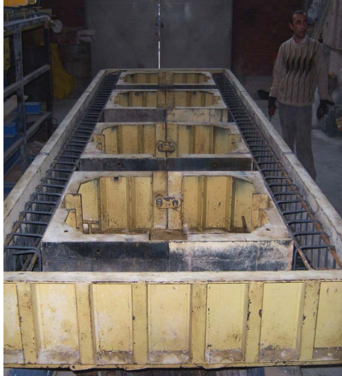
Figure 3.3 - General View of the Formwork
