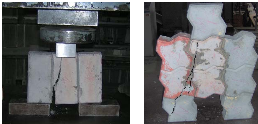
Figure 3.14 – Concrete Blocks After the Compression Test
