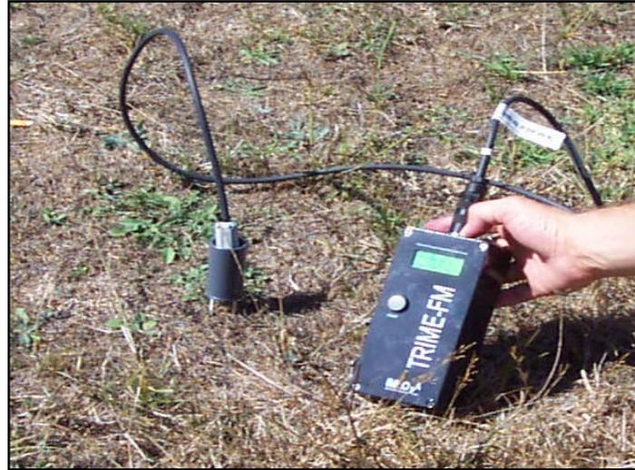
Figure 3.6. A typical measurement with a TDR
