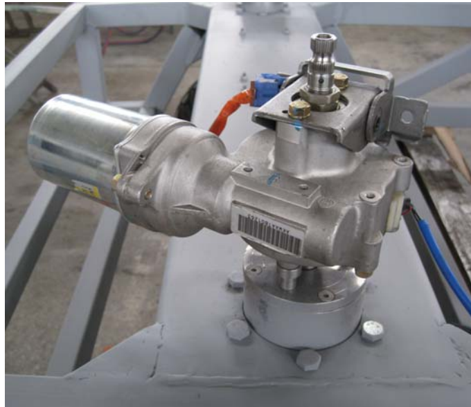
Figure 86 DC motor and gearbox at the top of the fork structure
