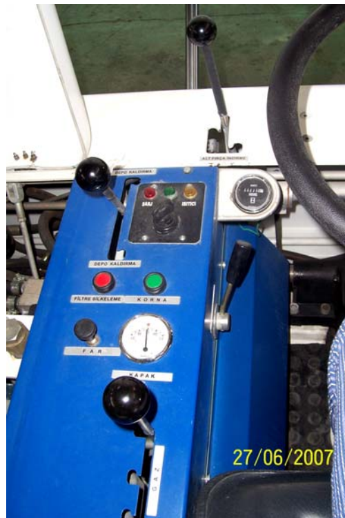
Figure 4 Müsan VSM 060 sweeper control panel
