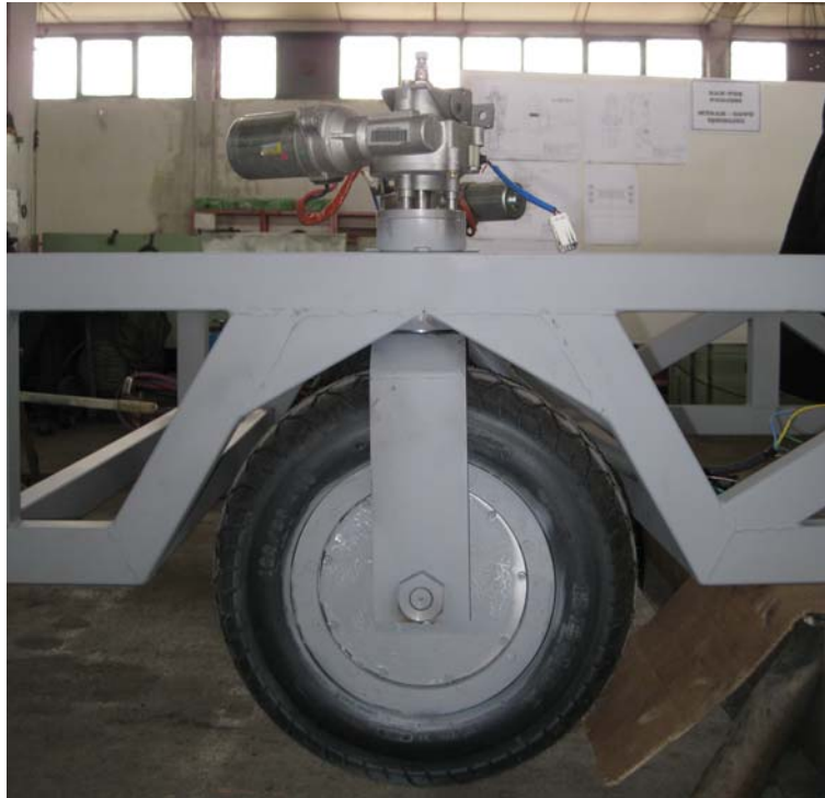
Figure 85 Fork structure, wheel and DC motor
