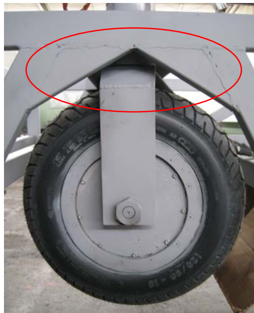
Figure 67 Critical locations from stress point of view
