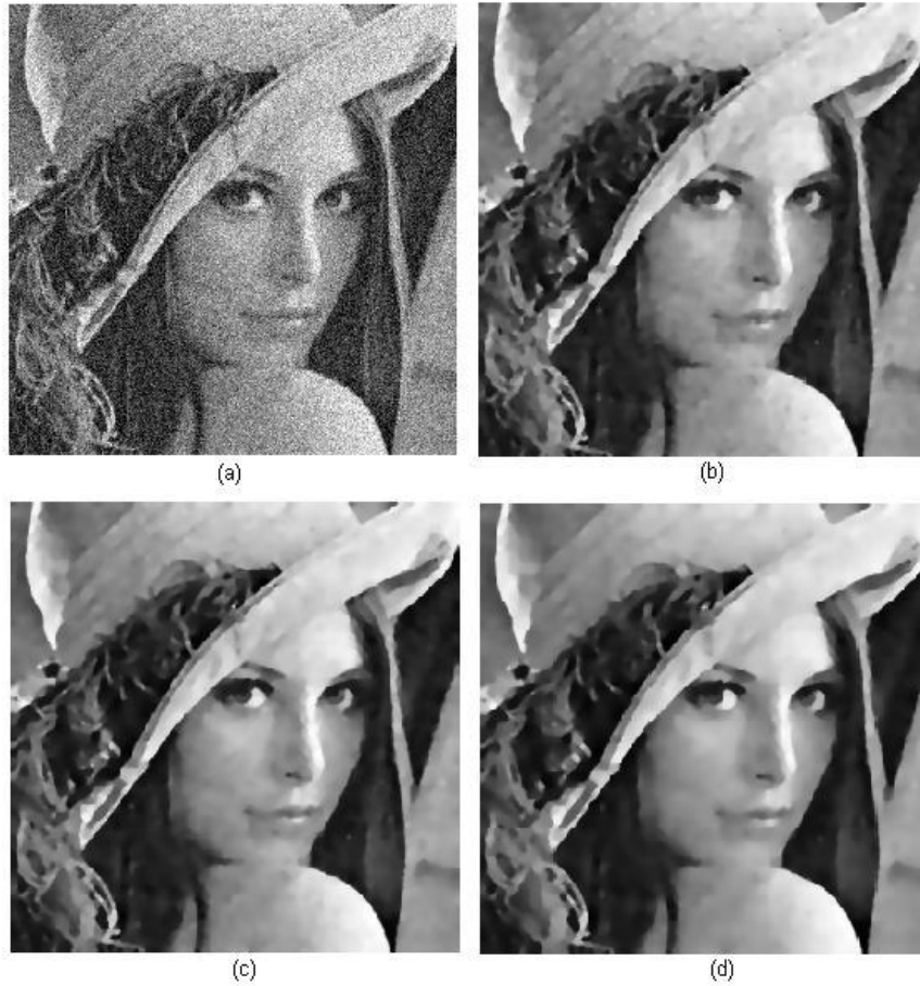
Figure 2.4: (a) Original noisy image. (b) The result of the PM model for 50 iterations, (c) the result for 60 iterations, (d) the result for 75 iterations.
