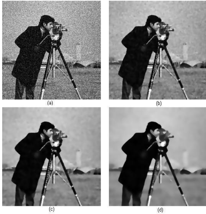
Figure 2.1: (a) The initial noisy image. (b) The result of the PM nonlinear diffusion for 30 iterations with k given by (2.4), (c) the result for 50 iterations and (d) the result for 100 iterations.
